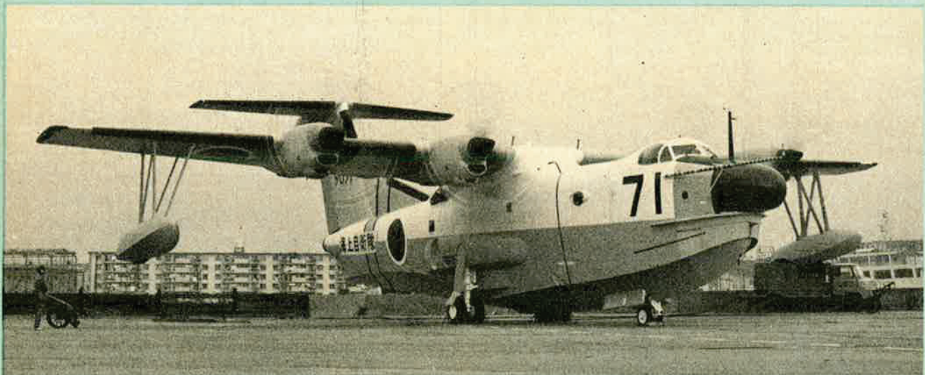
The first Shin Meiwa US-1, a STOL air/sea rescue amphibian development from the PS-1 anti-submarine flying-boat
