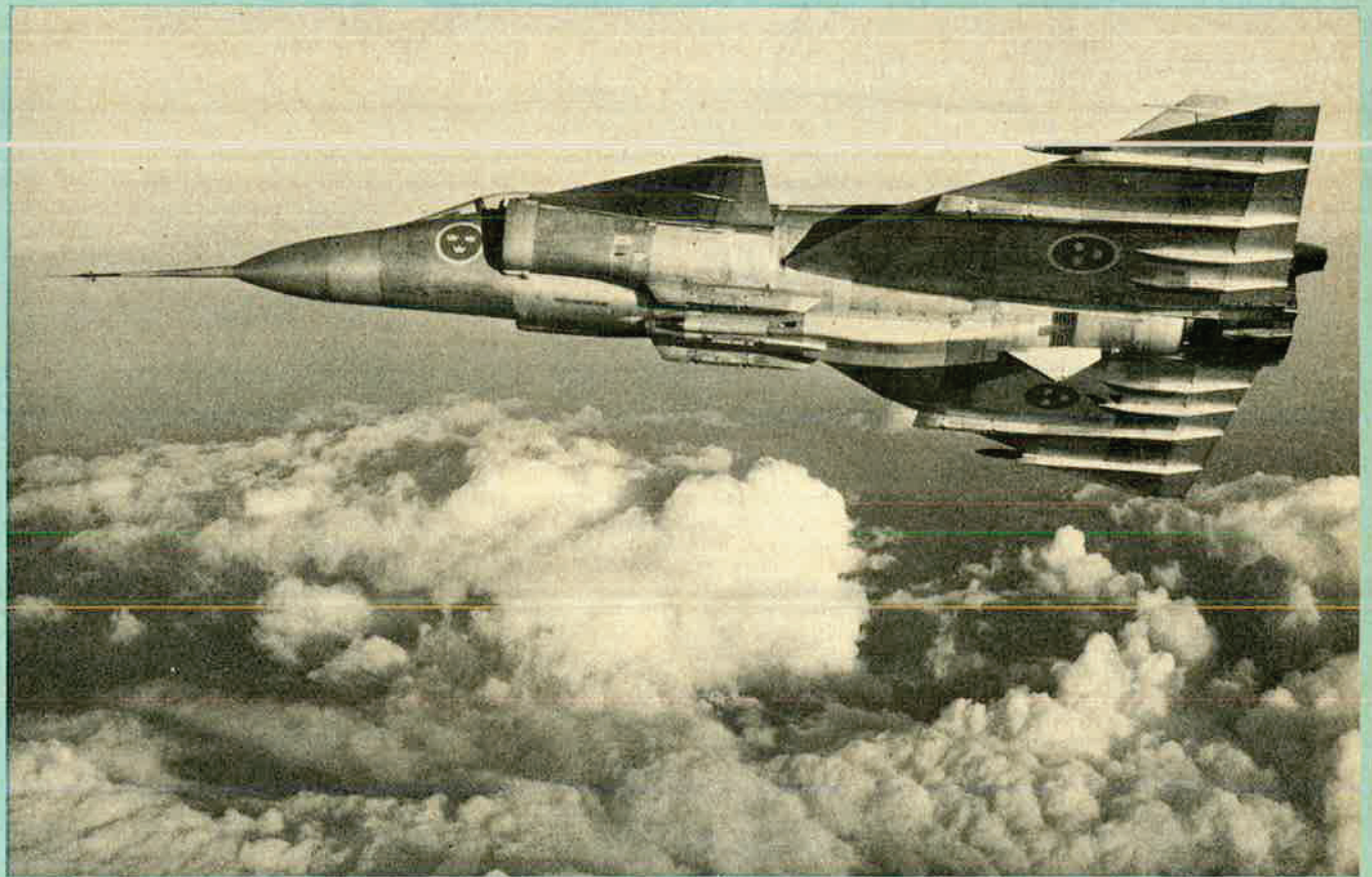
This view of a JA 37 development aircraft shows well the underfuselage 30 mm gun installation on this interceptor version of the Viggen
