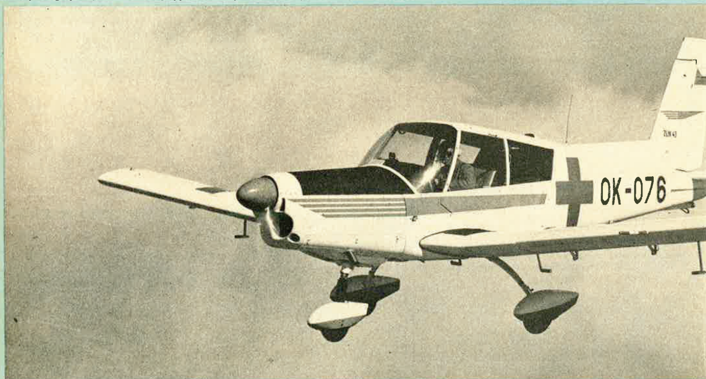
First photograph of a Zlin 43 equipped to carry a stretcher for air ambulance duties
