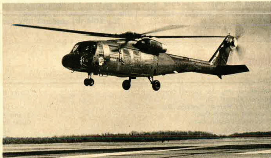
The Army's newest aircraft, the YUH-61A, made its first flight recently. Developed under the Boeing Vertol's Utility Tactical Transport Aircraft System program, the YUH-61A is a twin-engine, single hingeless rotor system helicopter in the 15,000-pound weight class. It boasts of reliability, safety, low vibration and noise levels, and economy.
