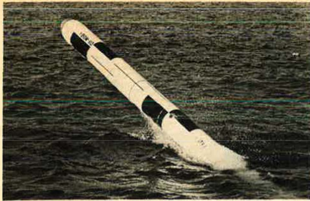
A Navy Cruise Missile Inert Test Vehicle, designed by LTV. In operation, this type missile—sub-, air-craft-, or ground-launched—would be boosted to flight speed by a rocket motor, extend its wings, and fly long distances powered by a small turbofan engine. Missions: tactical or strategic.
