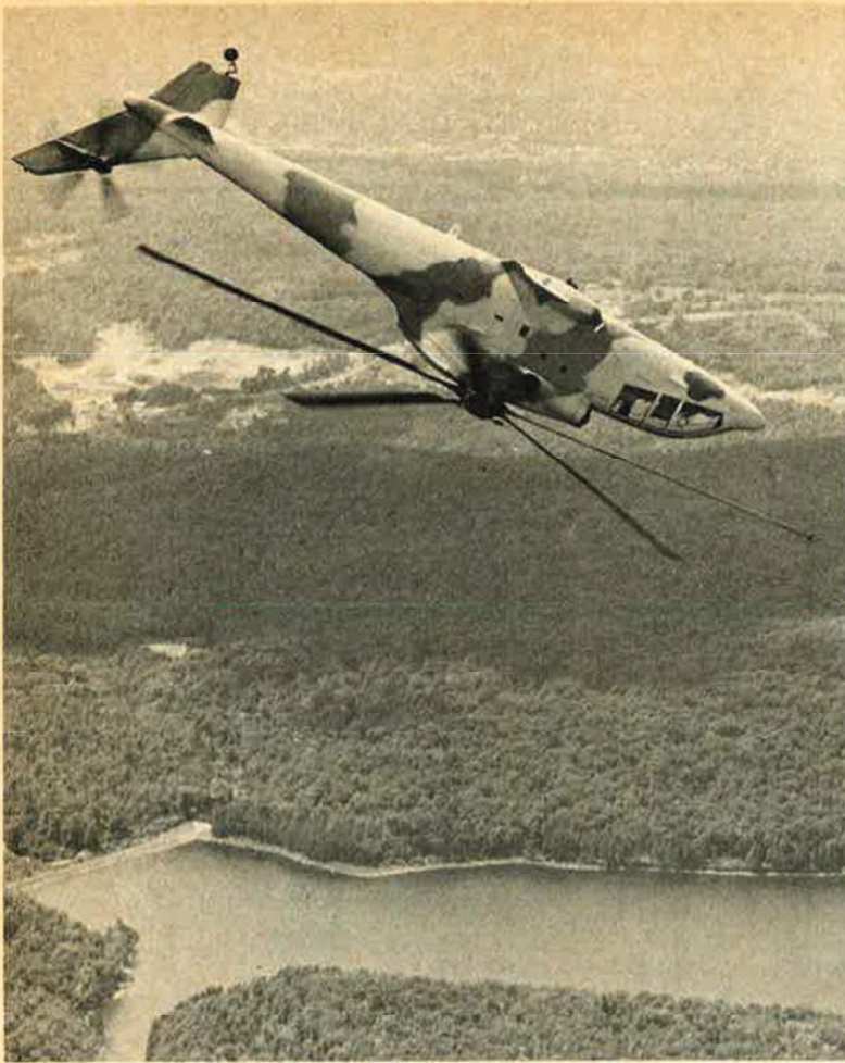
Holder of the world speed record for helicopters, the S-67 Blackhawk here rolls on its back to start a split-S turn, a manoeuvre Sikorsky considers normal for a combat helicopter.
