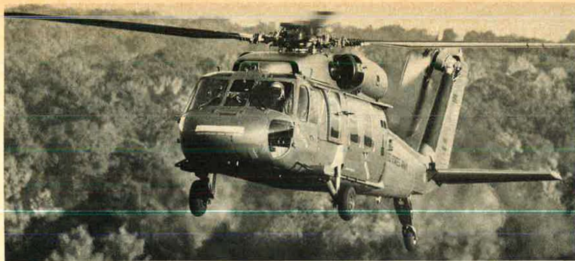
Sikorsky YUH-60A, first of the important UTTAS prototypes to fly, on 17 October 1974. Advanced features include swept blade tips, canted tail rotor, and low profile.
