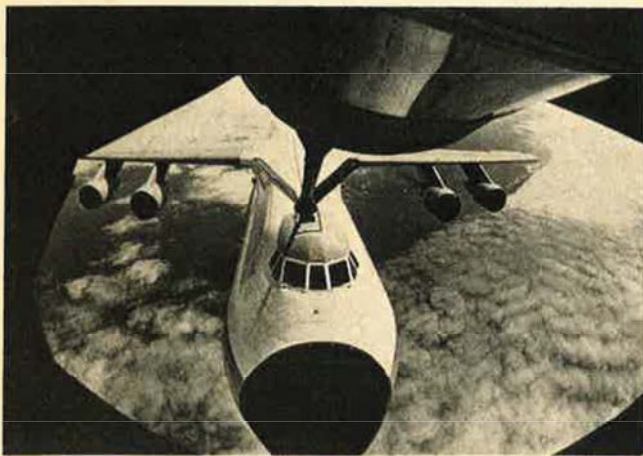
The Air Force's strategic airlift capabilities have been extended another giant step now that C-5 aircrews are being trained in aerial refueling techniques. This fish-eye lens photo of the huge cargo craft was taken by TSgt. Phil Tarbell from the boom operator's position aboard a KC-135 tanker on an inflight refueling mission out of Travis AFB, Calif. MAC also plans to equip its C-141s for aerial refueling.
