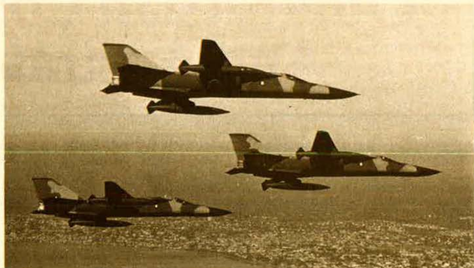
The Australian Air Force has one squadron of F-111Cs. Like SAC's FB-111 bombers, the C model has a longer wing than TAC's F-111s.
