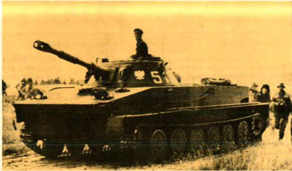
Chinese armored units use Soviet-built tanks and their own versions of Soviet designs, including this PT-76 amphibious tank.
