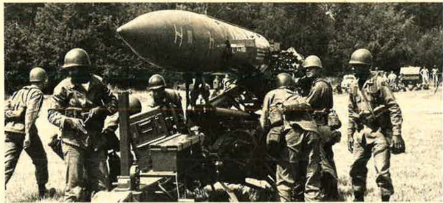
The US Army is replacing its Honest John and Sergeant surface-to-surface missiles with the Lance , shown here in Germany. Lance will carry either a conventional or a nuclear warhead, and is believed to have a range of about seventy-five miles.
