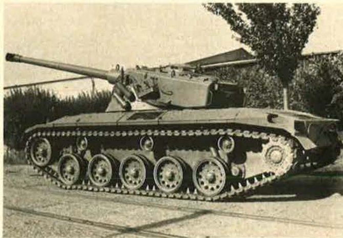
The Austrians developed and produced this Kuerassier tank destroyer for their army. It is equipped with a laser range-finder, and is highly maneuverable.
