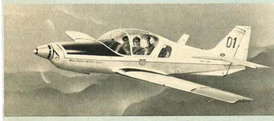
Artist's impression of the Scottish Aviation Bulldog Series 200, with retractable landing gear and four seats
