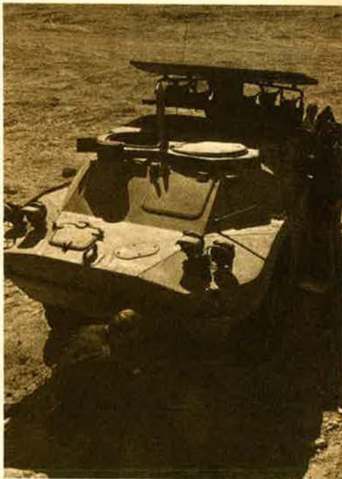
Soviet-built Sagger anti-tank missiles deployed by Egypt and Syria were highly effective in the Middle East war. The transporting vehicle is amphibious.
