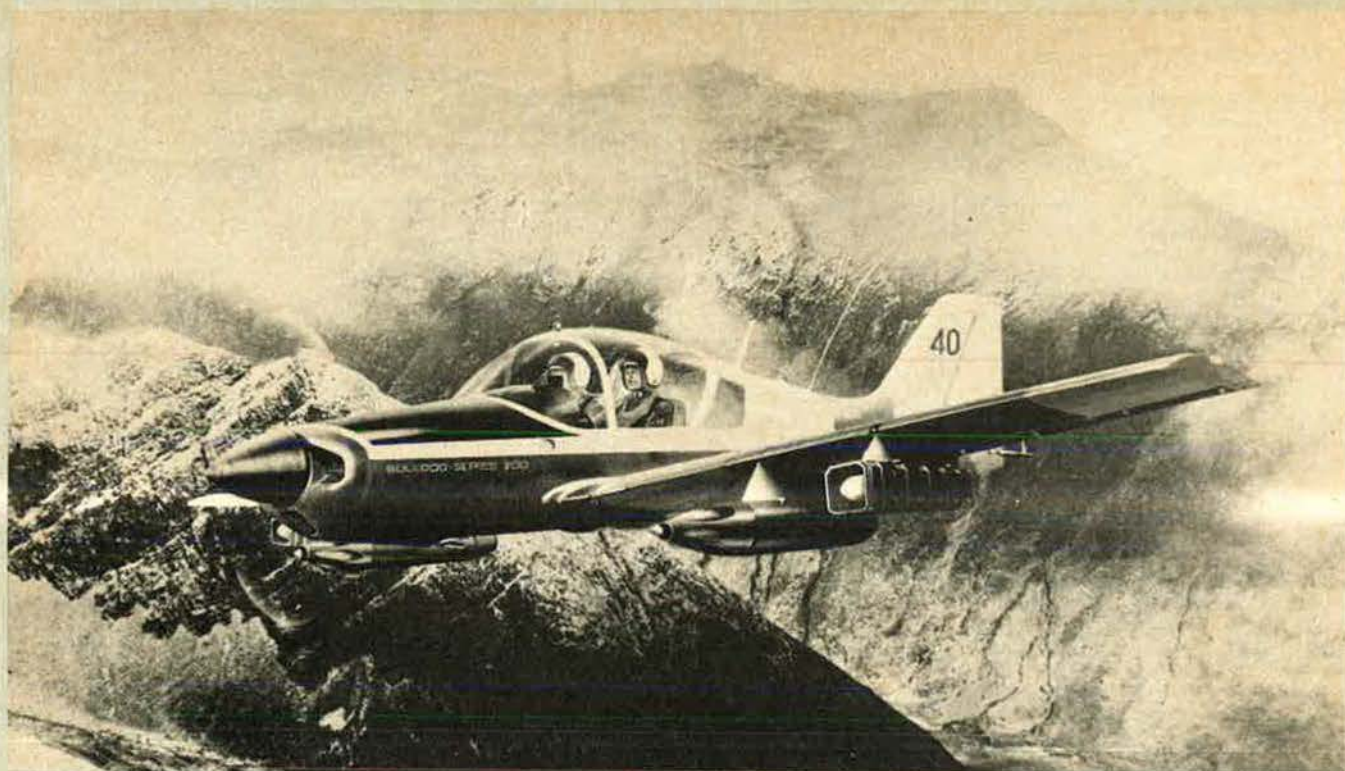
Bulldog Series 200 in light strike configuration, with underwing missiles and rocket pods
