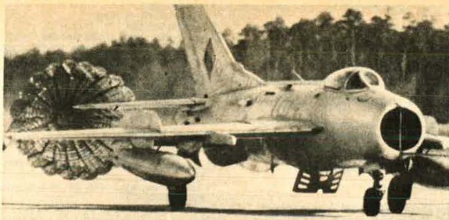
The MiG-19, a Mach 1.4 fighter, was first displayed publicly in 1955. It is still widely used by Pact and other air forces. This one bears Rumanian markings.
