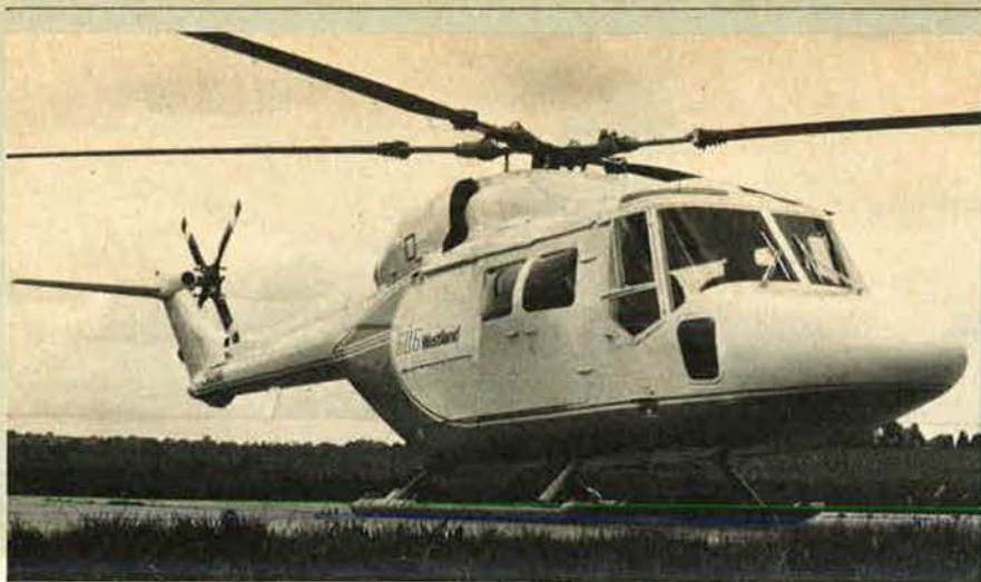
Full-scale mockup of the Westland 606 multi-purpose civil helicopter, derived from the military Lynx
