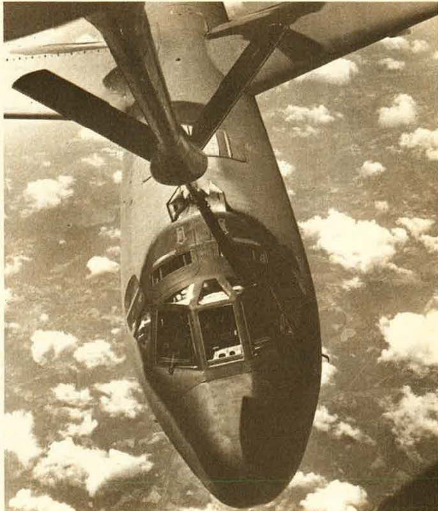
Air refueling gives the B-52G unlimited range. The big bomber can gulp 25,000 pounds of fuel from the KC-135 in as little as five minutes.
