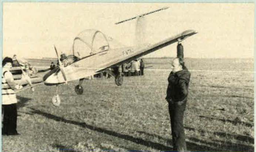
This photograph illustrates the fact that the Cricri is the world's smallest and lightest twin-engined aeroplane
