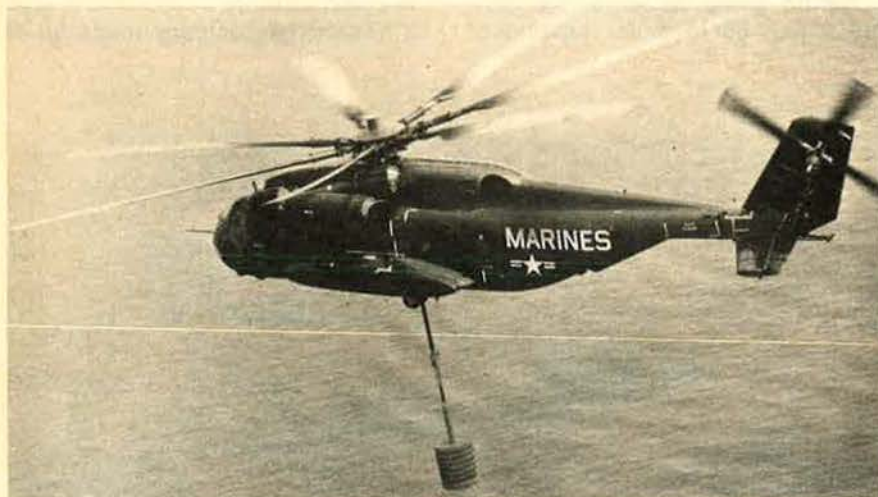
During a test flight, Sikorsky Aircraft's YCH-53E, a prototype heavy-lift helicopter under development for the Navy and Marine Corps, carries a payload of more than sixteen tons at 144 mph. The three-engine "E" is a growth version of the two-engine CH-53, in service since 1965.
