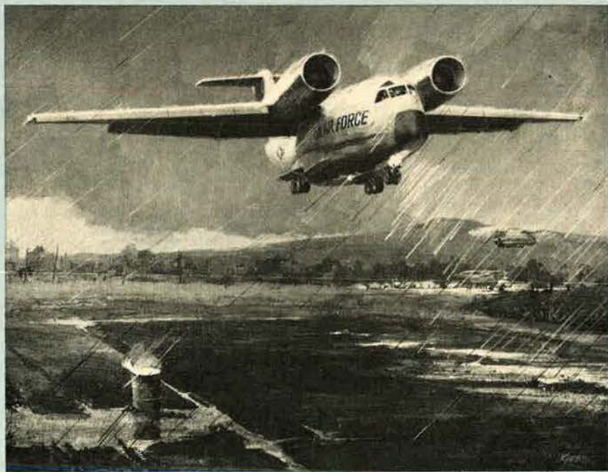
Artist's impression of the Boeing YC-14 prototype advanced medium STOL transport (AMST)
