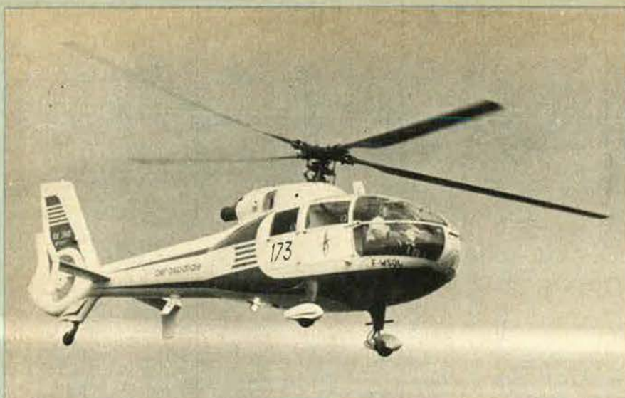
First prototype of the Aérospatiale SA 360 Dauphin, with original unstepped nose (J. M. G. Gradidge)
