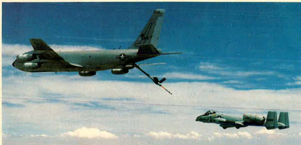
Fairchild Republic's A-10 close-air-support aircraft, powered by two GE TF34 engines, can carry an eight-ton flexible payload and is designed to deliver aerial firepower in support of friendly ground troops.
