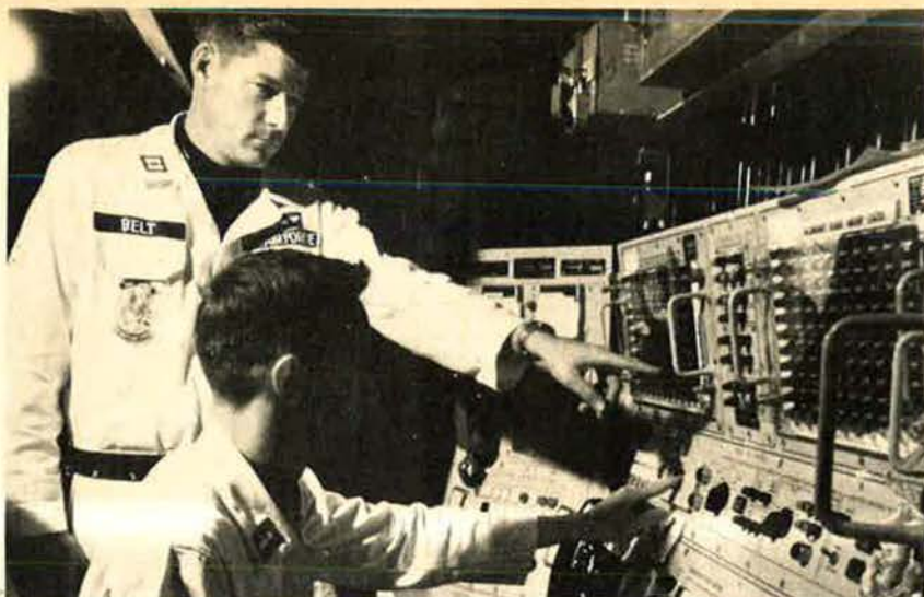
The launch control panel showing the status of the missiles is checked constantly by the combat crew.
