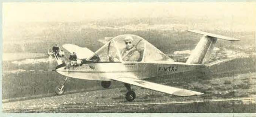
Colomban MC 10 Cricri homebuilt lightplane (two 9 hp Rowena two-stroke engines)
