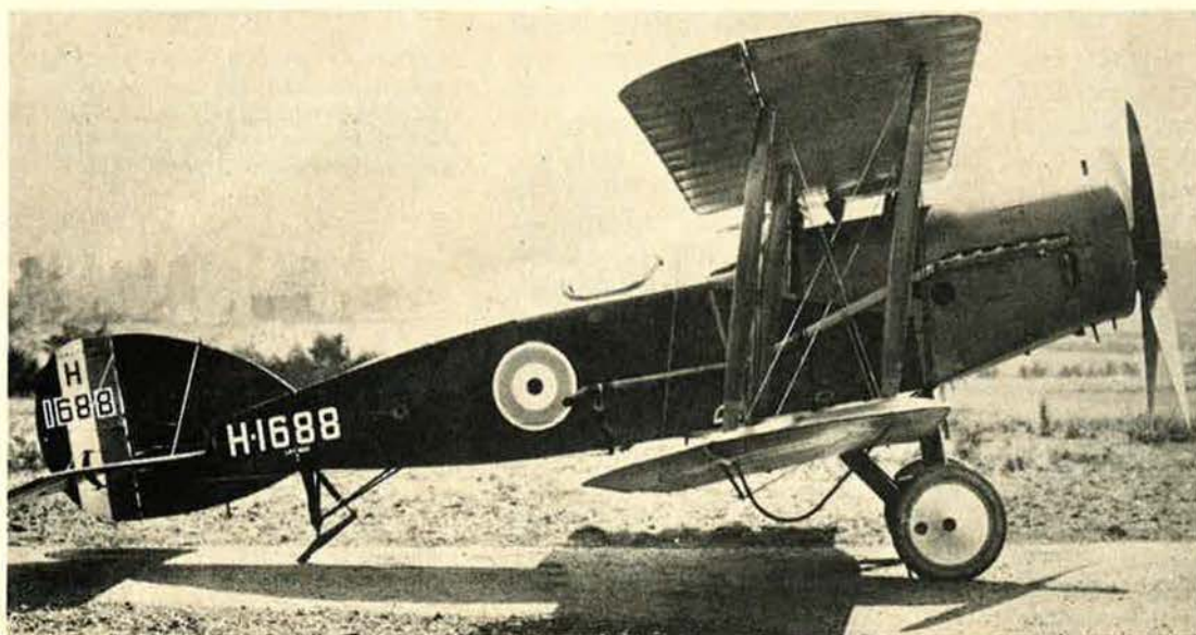
This prototype model of the Bristol Fighter was not yet fitted with the Scarff gun ring. The long exhaust pipes were also abandoned later.
