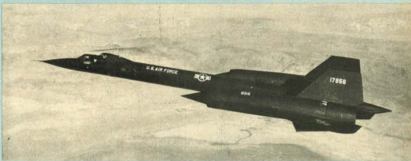
The SR-71B/C tandem two-seat training versions of the SR-71 were built with an elevated rear cockpit
