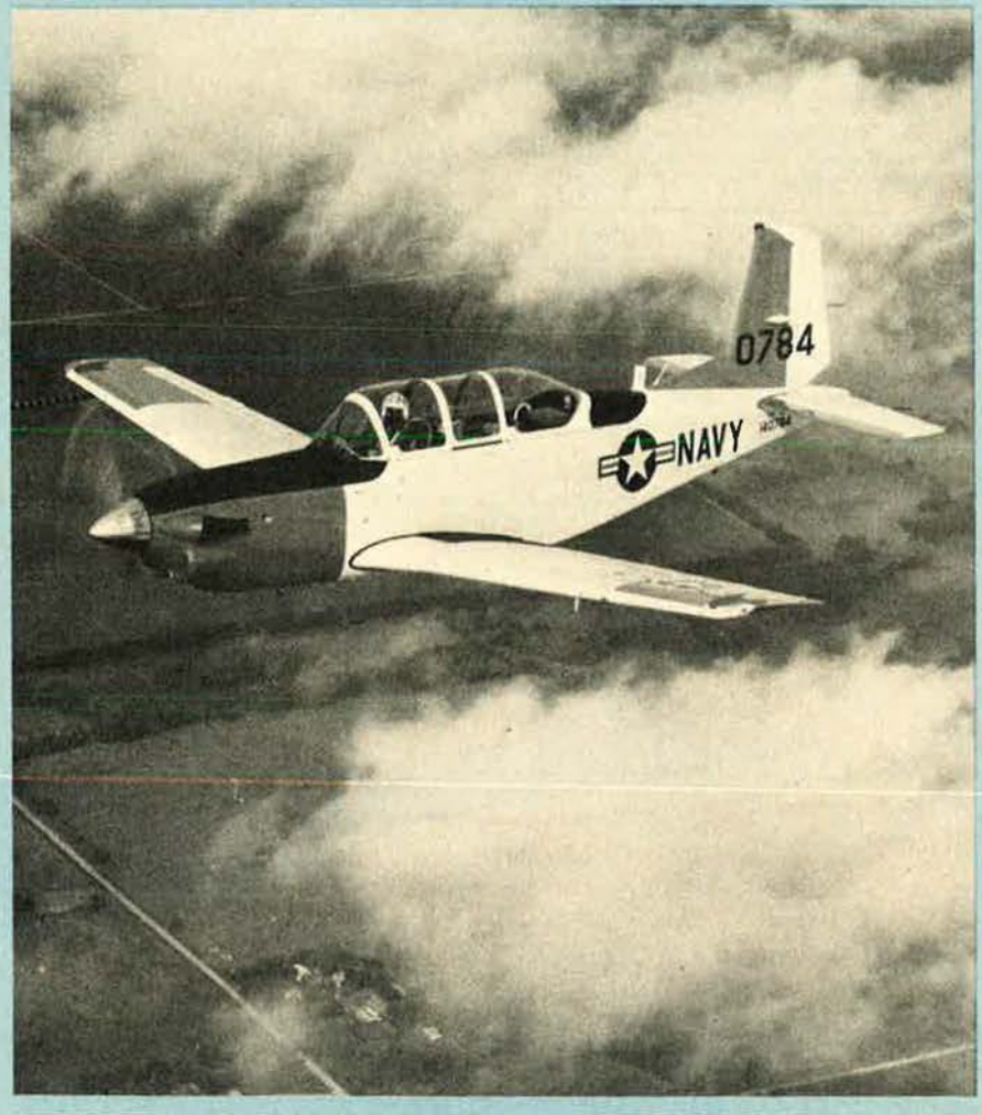
Beechcraft YT-34C Turbo Mentor, an experimental conversion of the T-34B Mentor trainer with a 715 shp United Aircraft of Canada PT6A-25 turboprop engine
