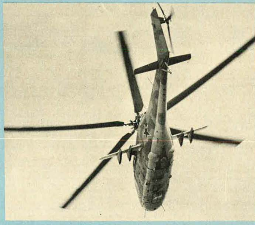
This version of the Mi-24, with only four weapon attachments on its auxiliary wings, has the NATO code name "Hind-B"
