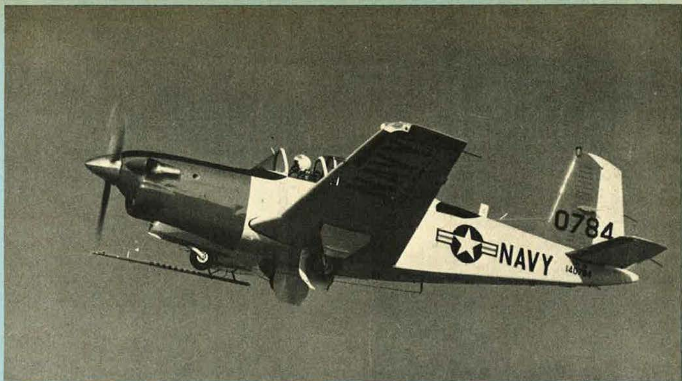
Beechcraft YT-34C Turbo Mentor, the gross weight of which is 1,000 lb (454 kg) more than that of the original Mentor, is continuing its test programme this Summer
