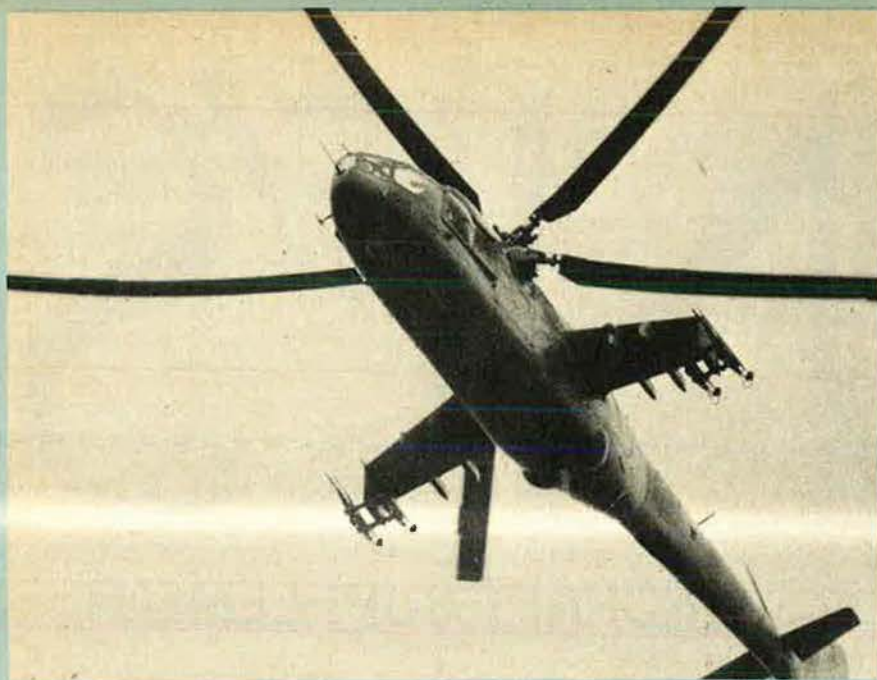
"Hind-A" version of the Mil Mi-24 with wingtip launchers for anti-tank missiles
