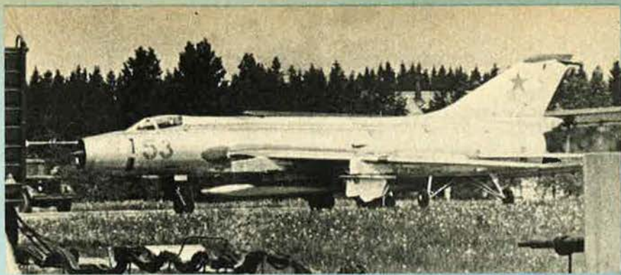
Improved "Fitter-B" variable-geometry fighter-bomber, with additional underwing weapon attachments and dorsal spine fairing containing fuel tankage (Tass)
