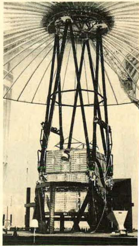
Above: Built by Fairchild Industries for NASA's Goddard Space Flight Center, ATS-6 can communicate with many simple and inexpensive ground terminals. Right: Heart of the new satellite is its Earth Viewing Module that includes high-powered transmitters and antenna feeds.
