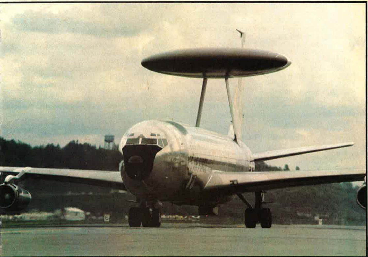
The E-3A AWACS aircraft is a modified Boeing 707-320 jetliner powered by TF33 engines and deploying a large radar rotodome.
