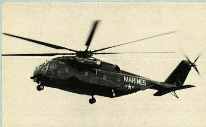
The three-engined Sikorsky YCH-53E prototype heavy-lift helicopter, photographed during its first flight, with landing gear extended
