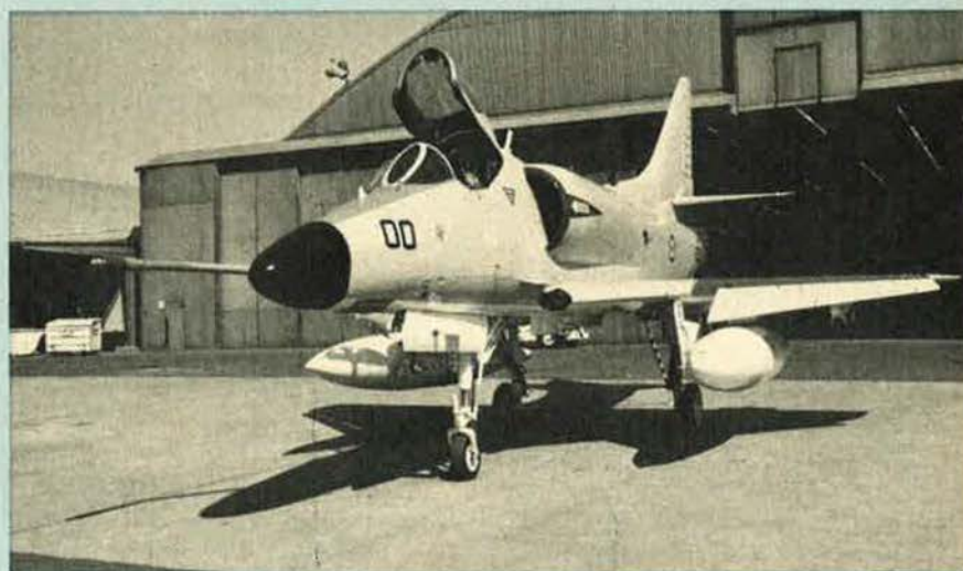
First of eight McDonnell Douglas A-4S Skyhawk fighter-bombers refurbished and modified for Singapore Air Defence Command by LAS at Ontario, California. Another 32 are being produced in Singapore
