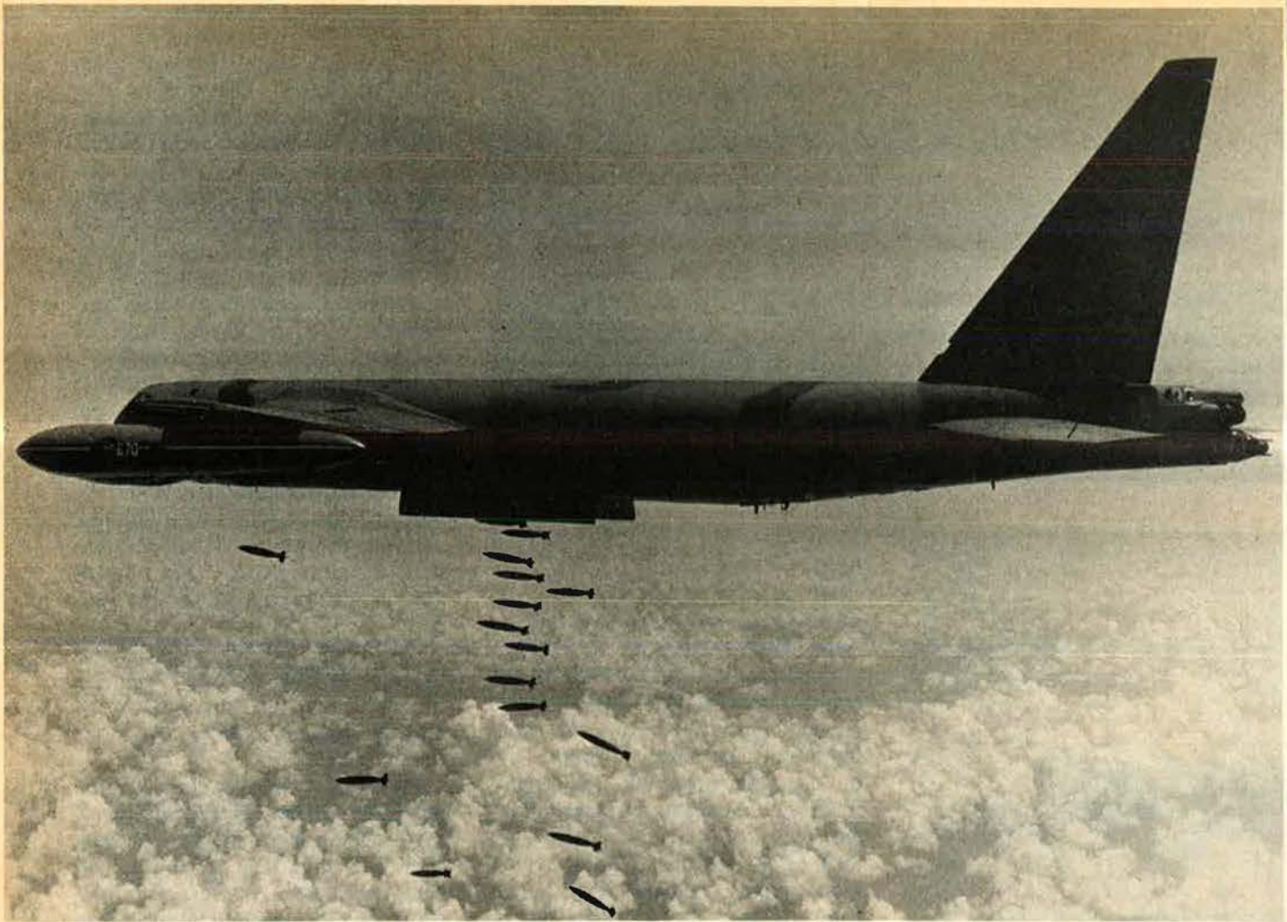
Flying in cells of three aircraft, the B-52s could deliver their bombs on command from ground-based precision radars, by LORAN, or with their own integral radar-bombing systems.
