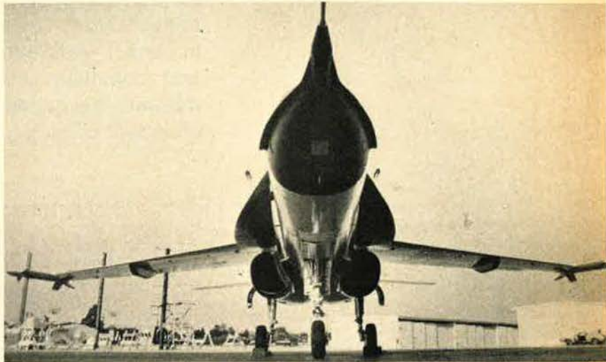
The YF-17's nose fuselage strakes contribute to control and stability in high-G turns. Slotted and highly swept leading-edge wing extensions improve maneuverability and ensure uninterrupted airflow to the engines at high angles of attack.
