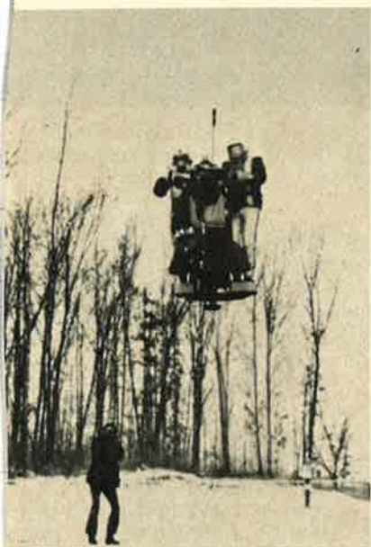
For the US Marine Corps, Williams Research Corp., Walled Lake, Mich., has designed this two-man flying platform. Turbine powered, it can stay airborne for thirty minutes at speeds of sixty mph. It produces 700 pounds of thrust.
