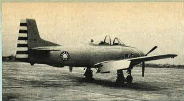
AIDC XT-CH-1A prototype secondary trainer (1,450 ehp Lycoming T53-L-701 turboprop engine)
