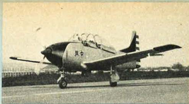
The AIDC XT-CH-1A is a tandem two-seat secondary trainer. The first one flew on 23 November 1973
