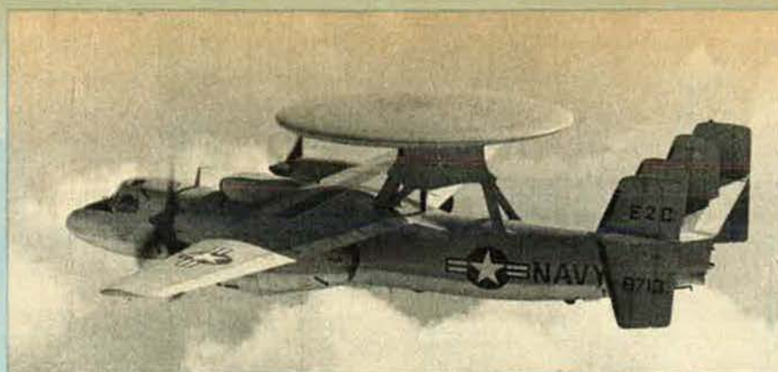
Grumman E-2C Hawkeye airborne early-warning aircraft (two 4,910 ehp Allison T56-A-422 turboprop engines)
