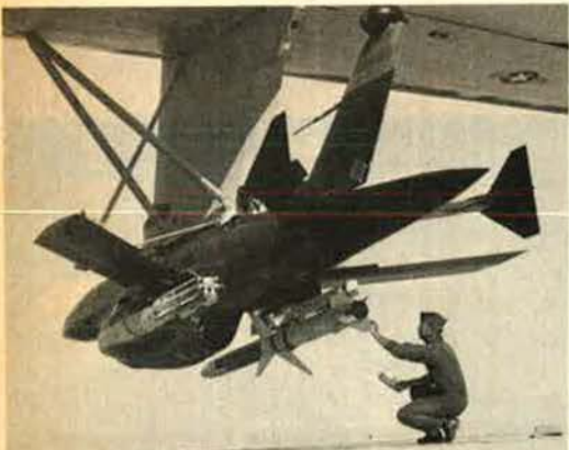
BGM-34 with Shrike missile under right wing and Mk IV bomb under left wing
