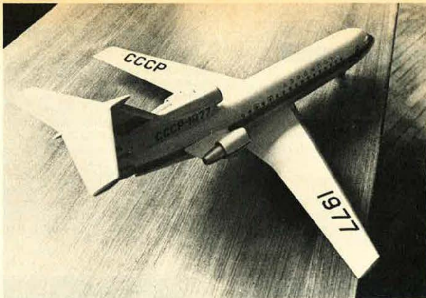
A model of the Yak-42 transport, developed for Aeroflot, the Soviet airline. The Yak-42 can be configured to carry 120 passengers and has a range of more than a thousand kilometers at a cruising speed of 820-870 km. per hour.
