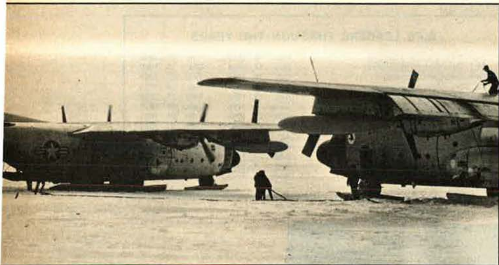
Ski-equipped C-130s of AAC's 17th Tactical Airlift Squadron provide logistic support to Distant Early Warning radar sites on the Greenland ice cap.
