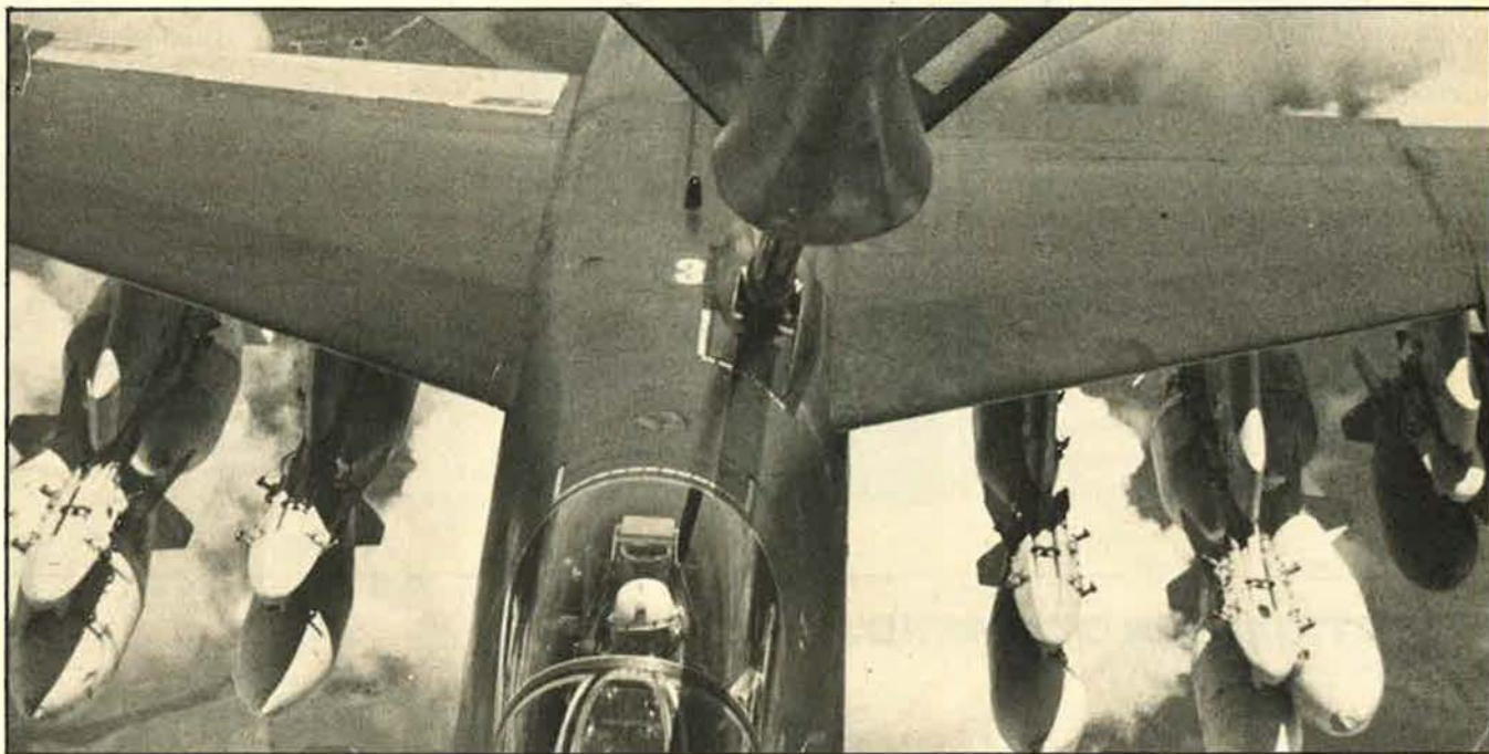
One of TAC's A-7Ds, loaded with more than 12,000 pounds of bombs, refuels from a KC-135 en route to a target range.
