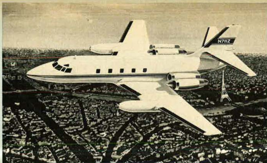
Artist's impression of Lockheed JetStar II executive transport (four AiResearch TFE 731-3 turbofan engines)
