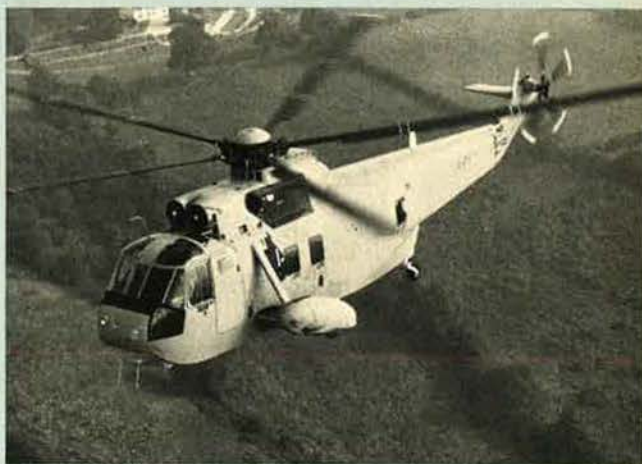
Westland Commando is a development from the Sea King. Designed for land-based operation, it will be able to carry up to 30 troops in the Mk 2 form
