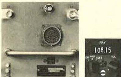
Typical of off-the-shelf avionics is the AN/ARN-108(V) combining VOR, ILS, marker.
