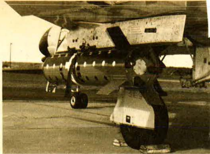
Rear view of 500-pound FAE weapon shows four "second-event guns," which position the detonators in the fuel cloud.
