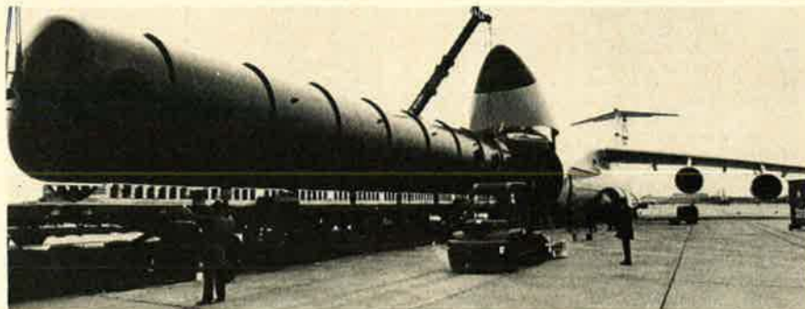
The bulkiest equipment ever airlifted, a ninety-one-by-fourteen-foot underground fuel storage tank, is eased aboard a C-5 Galaxy at Rhein-Main AB, Germany, for airlift to Incirlik AB, Turkey. Using extreme caution, it required six hours to load the 86,000-pound container and more than four hours to offload. The cargo hold of the C-5 is 121 feet long by nineteen feet wide.
