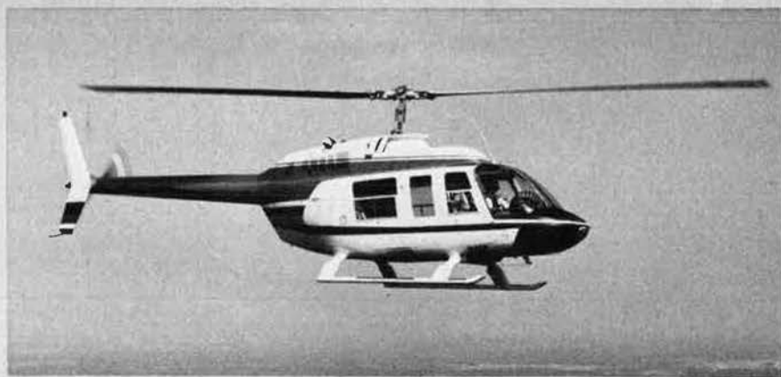
Bell Model 206L Long Ranger, a stretched seven-seat development of the JetRanger II
