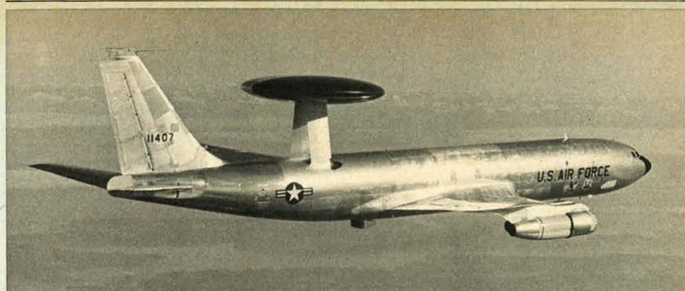
Boeing EC-137D testbed aircraft for the USAF's Airborne Warning And Control System (AWACS) programme
