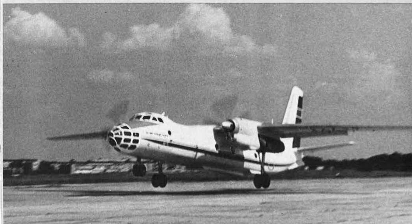
Antonov An-30, a new aerial survey aircraft developed from the An-24 twin-turboprop transport
