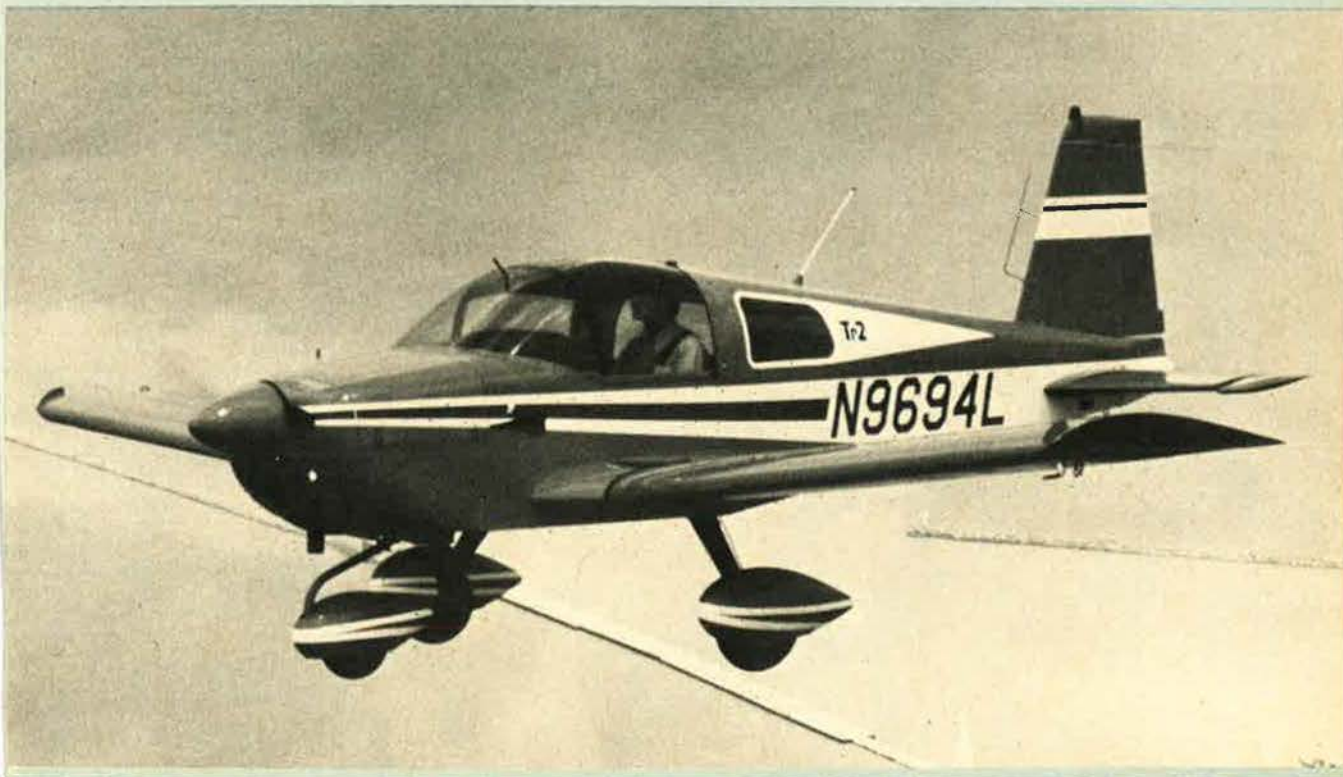
Grumman American Tr2 two-seat light aircraft (108 hp Lycoming O-235-C2C engine)
