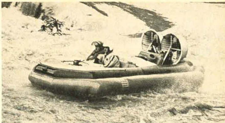
One of a number of lightweight inflatable hovercraft designed and built in Great Britain, a Skima 4 shows its potential in rapids during a recent 300-mile journey on unnavigable waters in North America. The craft may be put to a variety of uses once fully proved out (see item below).
