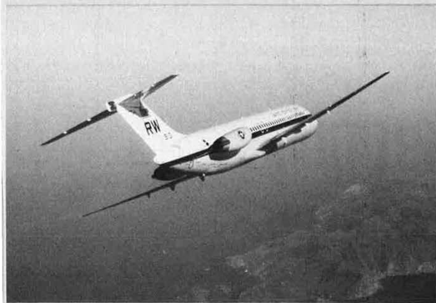
The US Navy's McDonnell Douglas C-9B Skytrain II combines the basic DC-9 Series 30 airframe with the power plant of the Series 40
