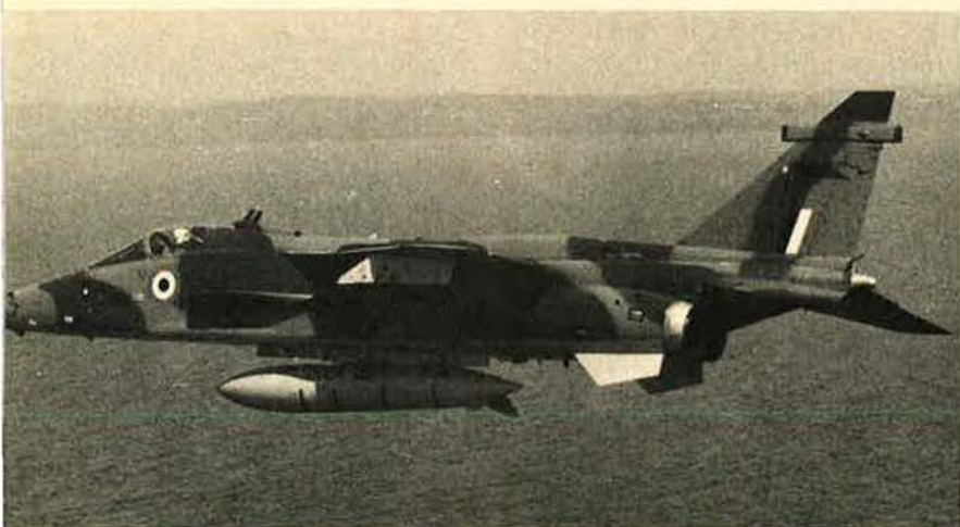
Equipment on the RAF Jaguar tactical fighter includes a nose-mounted laser rangefinder and tail-mounted ECM pod.
