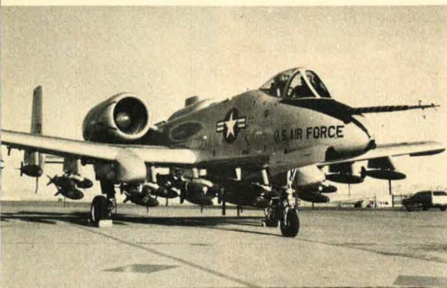
The Fairchild Republic A-10A was designed specifically for close-support work, with emphasis on heavy weapon loads and high survivability.
