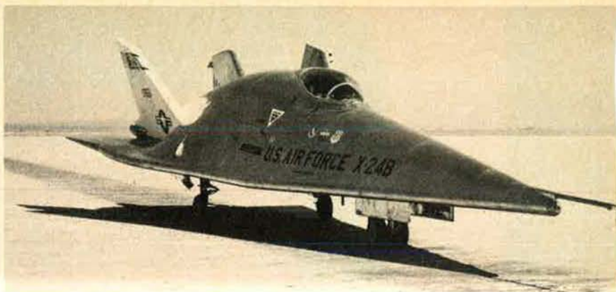
A joint USAF/NASA project, the X-24B lifting body flight-test program got under way last summer at Edwards AFB, Calif. The Air Force is currently considering the feasibility of building yet a third-generation X-24 capable of attaining speeds of Mach 5 (3,500 mph).
