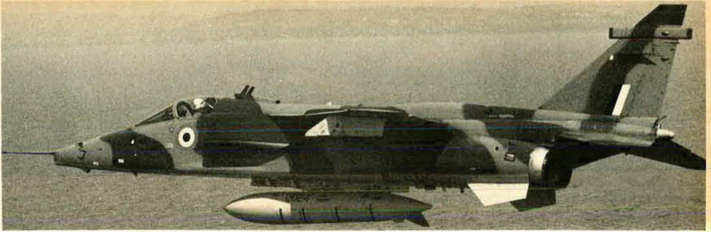
The Anglo/French Jaguar S.07, a supersonic tactical support aircraft, is now in service with the French Air Force. It can operate from short fields.
