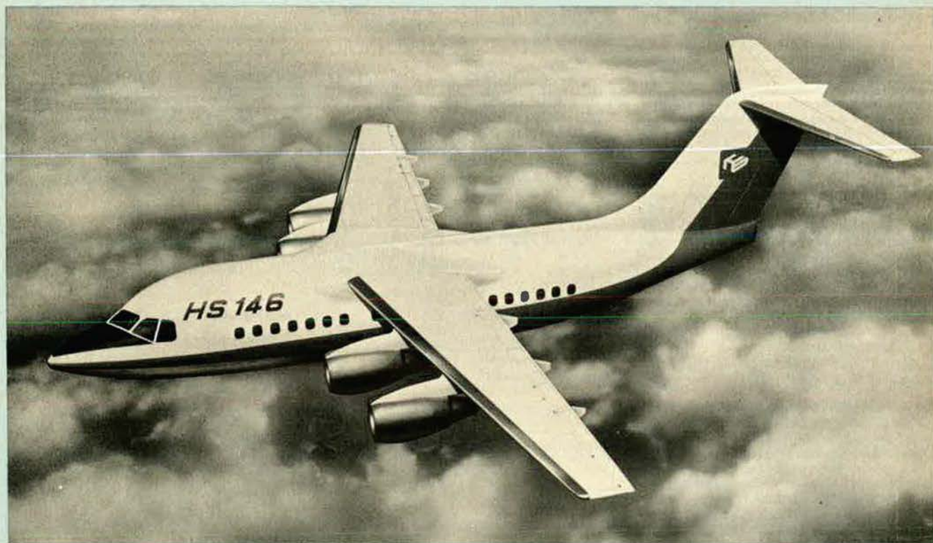
Artist's impression of the HS 146 (four Avco Lycoming ALF 502-H turbofan engines)
