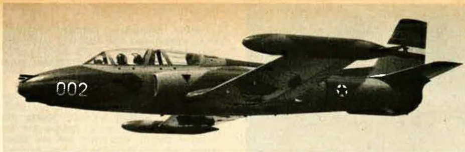
Yugoslavia produces its own jet trainer, the G-2-A Galeb (Seagull), with a more advanced version—the G-3—being developed for support and recce roles.
