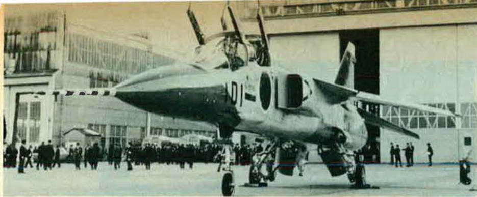
The Mitsubishi XT-2 jet trainer and light attack aircraft is Japan's first domestically designed supersonic plane, capable of Mach 1.6 speed.
