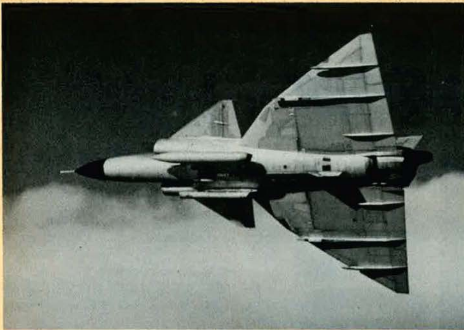
Sweden's SAAB AJ-37 Viggen is a Mach 2.0 multimission fighter that can be equipped for attack, intercept, reconnaissance, or training roles.
