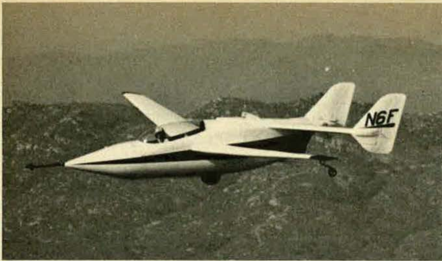
Ryson STP-1 Swallow two-seat cruise/soar aircraft (76 hp CE-2200 Barker-converted Volkswagen engine)
