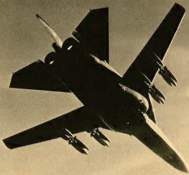
The Australian Air Force is integrating the F-111C into its operational forces. The "C" has a slightly longer wing than USAF F-111s.
