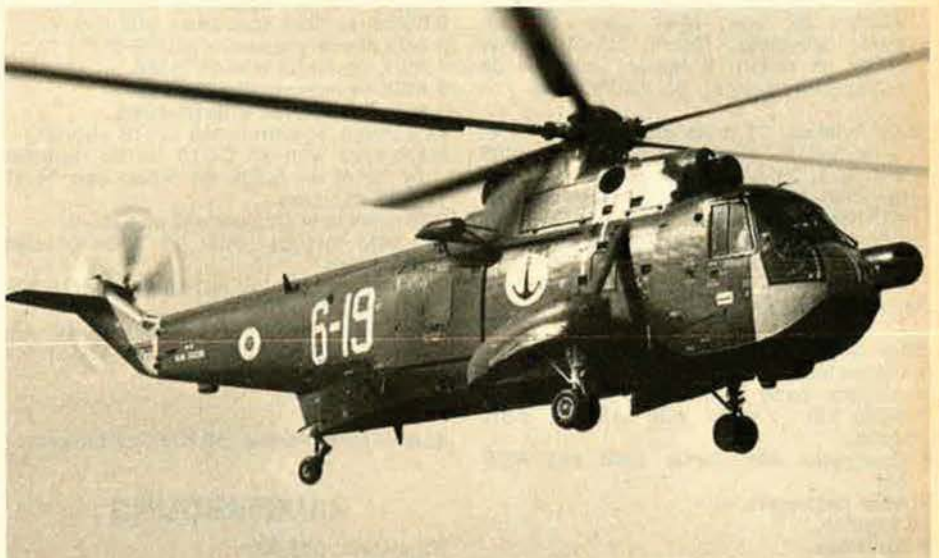
One of the Italian Navy's Agusta-Sikorsky SH-3D Sea King ASW helicopters with AN/APN-195 search radar.
