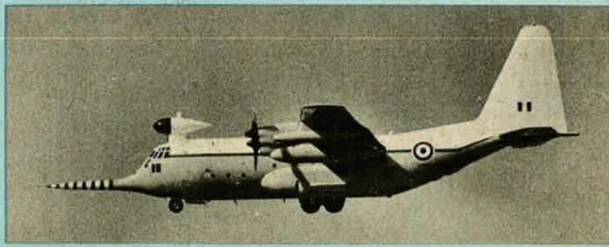
Hercules W. Mk 2, modified from a C. Mk 1 by Marshall of Cambridge for the RAF's Meteorological Research Flight
