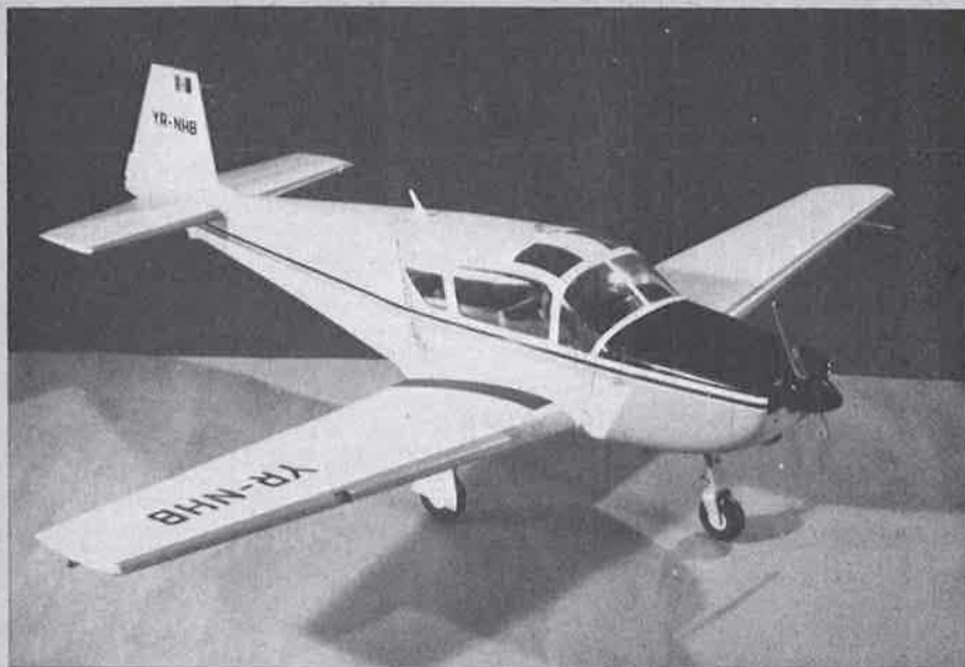
Model of IAR-823 two/five-seat light aircraft (290 hp Lycoming IO-540-G1D5 engine)
