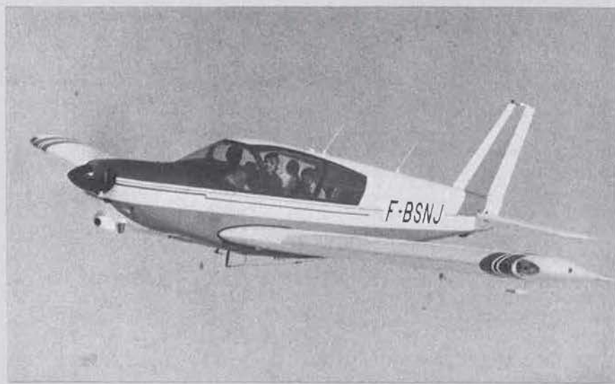
CERVA CE.43 Guépard four-seat light aircraft (250 hp Lycoming IO-540-C4B5 engine)
