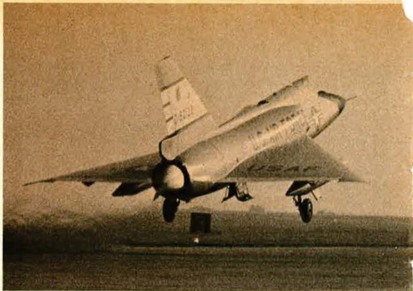
A single 24,500-pound-thrust engine propels the F-106 skyward.
