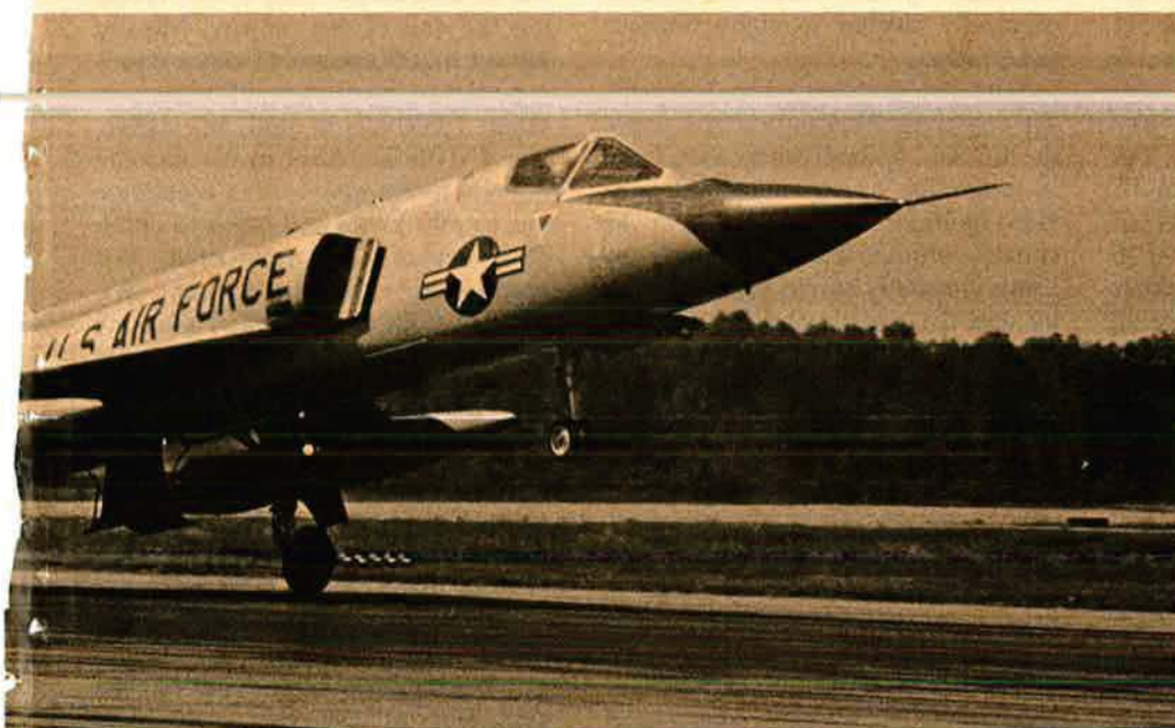
Aerodynamic braking helps bring the F-106 to a halt. The lack of wing flaps causes the 'Six' to fly final approach at speeds nearing 200 knots. Speed brakes and drag chute further cut the landing distances.
