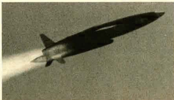
MQM-74/CHUKAR. The first low-cost jet-powered drone.
