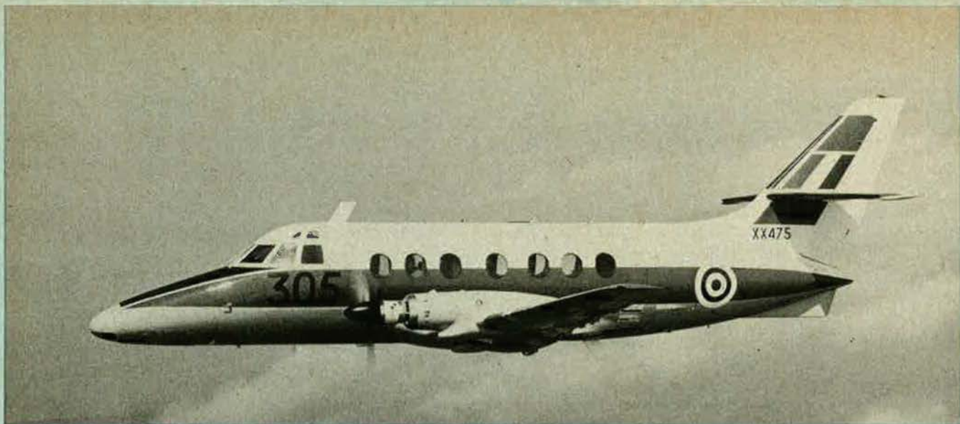
Scottish Aviation Jetstream T. Mk 1 multi-engine pilot training aircraft for the Royal Air Force
