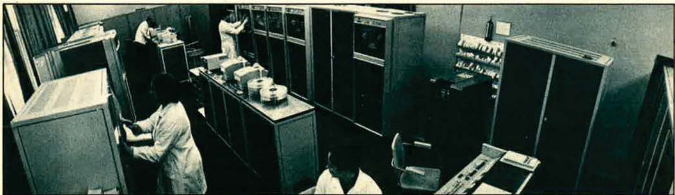
Computer installation, of the Minsk type, is used to automate and control Tu-144 fabrication.
