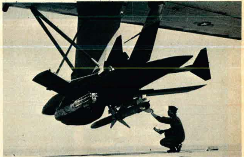
A Teledyne Ryan Model 234 RPV armed with a Shrike missile and a Mark IV bomb.
