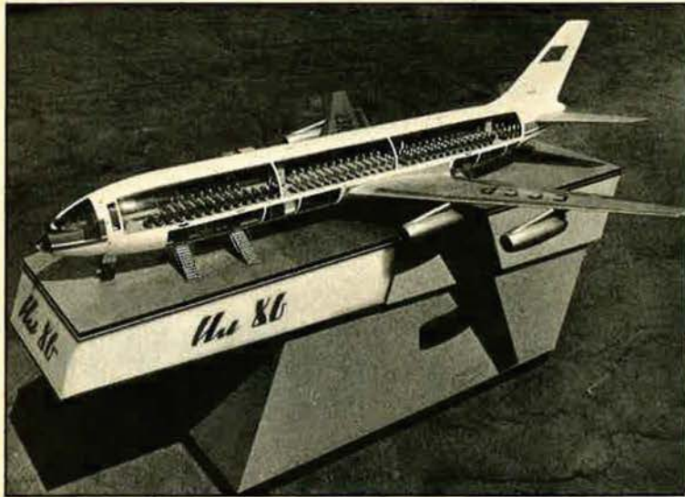
The Il-86, the Soviet airbus, will accommodate up to 350 passengers, mainly on domestic routes.
