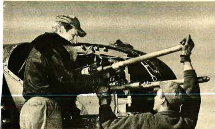
Two airmen of the 3d Bomb Wing check the twin .50-caliber machine guns mounted in the nose of this B-26.
