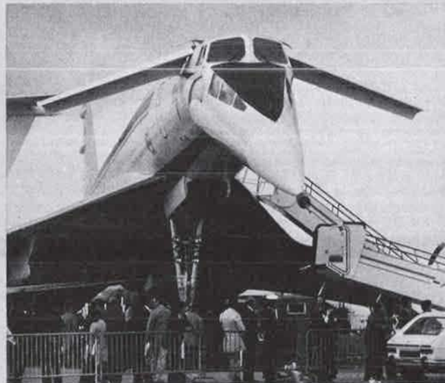
The Tu-144's "moustache" foreplanes are pivoted from points near the top of the fuselage, immediately aft of the flight deck, and are retractable (Air Portraits)
