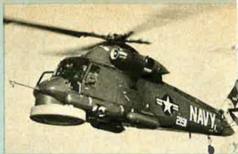
Kaman HH-2D modified for test-flying Cubic Corporation's retractable radar antenna in an inflatable radome
