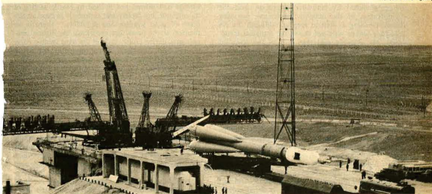
The Soyuz-10 orbital spacecraft is shown mounted on the standard, heavy-duty rocket launcher used by the USSR in slightly varying configuration for different payloads.
