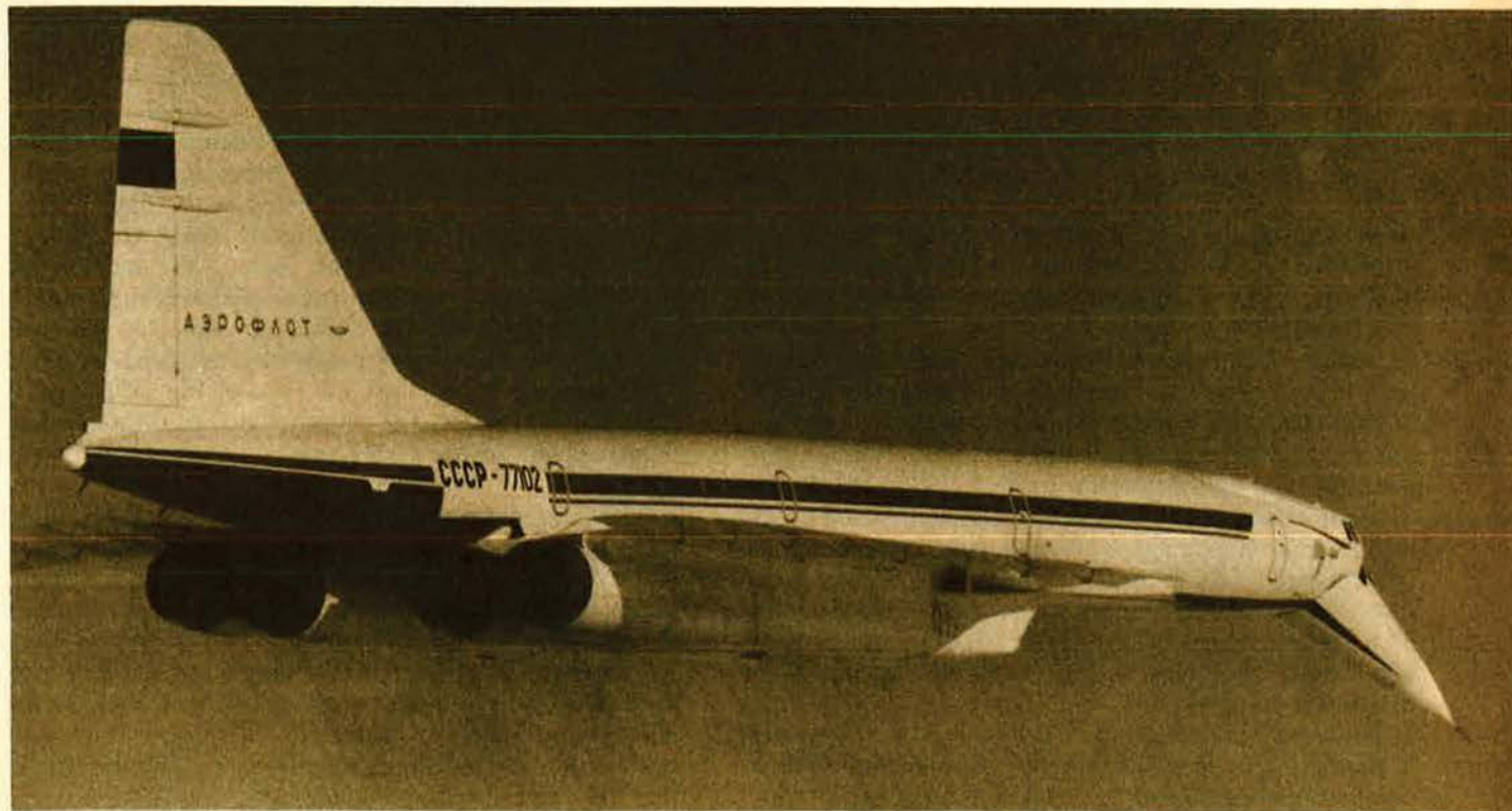
Soviet TU-144, shown in flight with its movable nose in down position, can transport 150 passengers over a distance of more than 4,000 statute miles and will cost less than the British-French Concorde.
