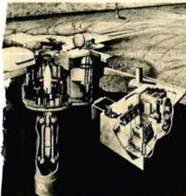
Minuteman III's advanced silo and launch control center, shown here in cutaway form, will be able to survive a near miss from a large-yield weapon, according to SAC briefers at the AFA Symposium.
