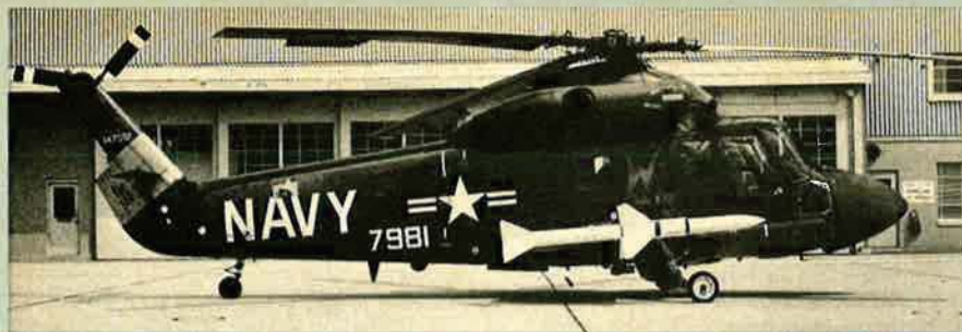
Kaman NUH-2C Seasprite, a one-off modification of the UH-2C to carry Sparrow III or Sidewinder missiles, seen here with a Sparrow
