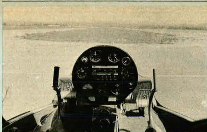
This photograph from the cabin emphasizes the helicopter-like forward field of view offered by the Explorer
