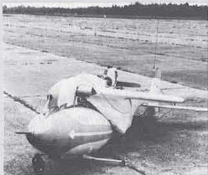
Fairchild Sailwing RPV fitted with lightweight jettisonable landing gear and with wings folded
