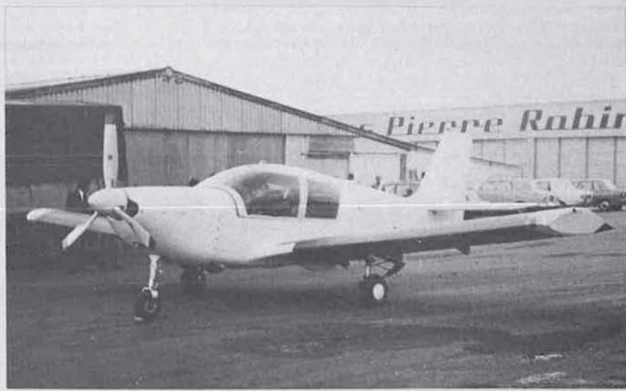
First Robin aircraft with retractable landing gear, the HR 100/Tiara prototype, unpainted before its first flight
