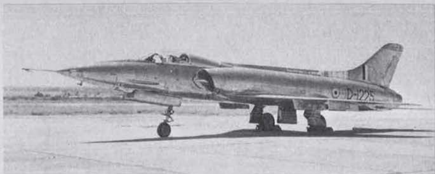
HAL HF-24 Marut Mk I (two Rolls-Royce Bristol Orpheus 703 turbojet engines)
