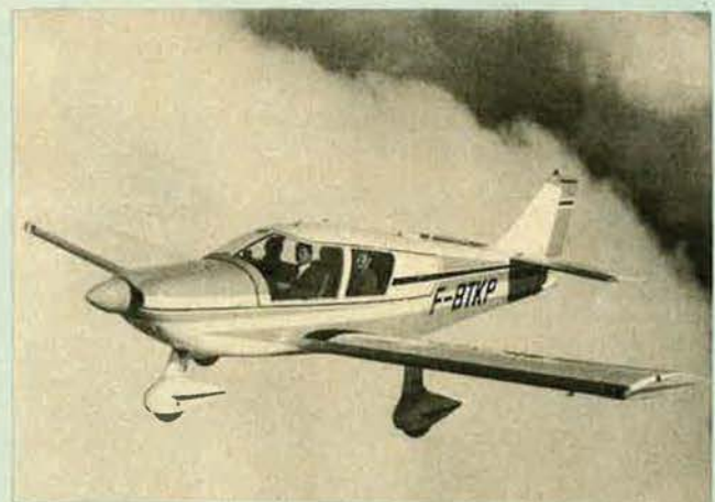
The all-metal HR 100/210F, with 210 hp Continental IO-360 engine and fixed landing gear
