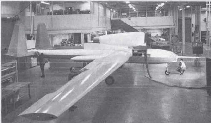
Boeing YQM-94A strategic RPV, built under the USAF's Compass Cope programme
