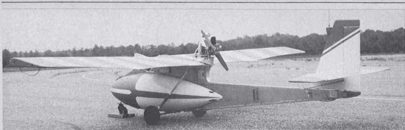
Fairchild Sailwing RPV (13 hp McCulloch engine) with tricycle landing gear attached
