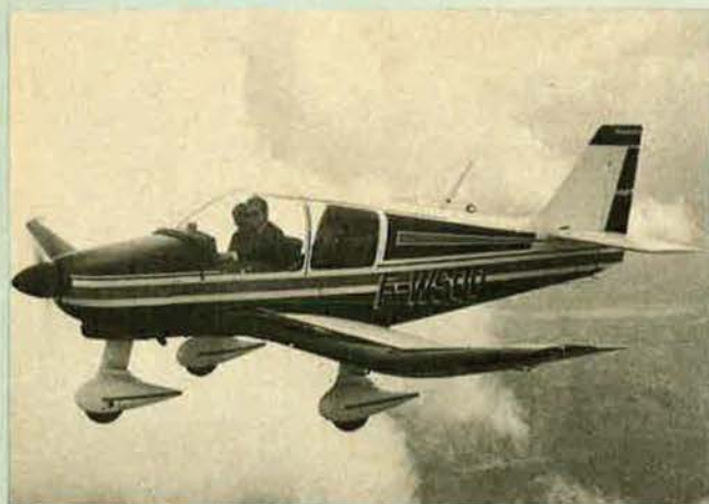
Robin DR 400/180 Régent, most powerful of the 400 series of wooden lightplanes, with a 180 hp Lycoming O-360-A engine
