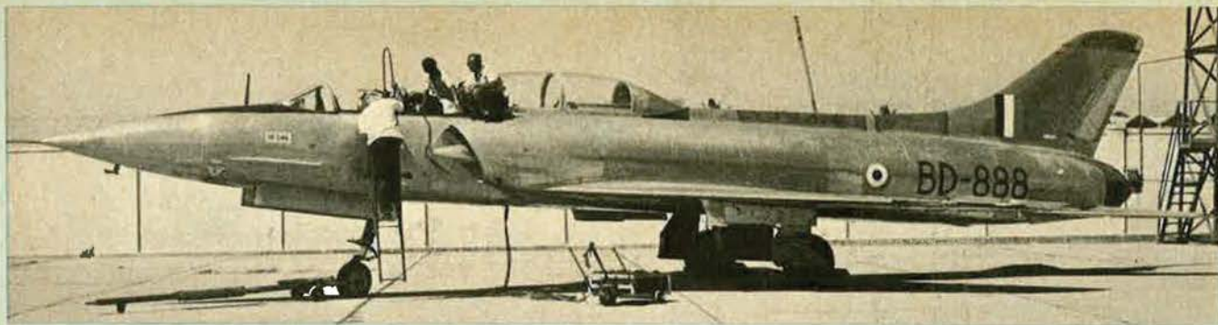
Prototype of the HAL HF-24 Mk IT two-seat training version of the Marut (Alan W. Hall)
