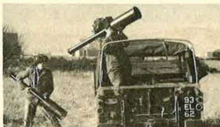
The man-portable Blowpipe, with IFF capability, is an answer to the infantryman's need for a small, lightweight, short-range anti-aircraft missile.
