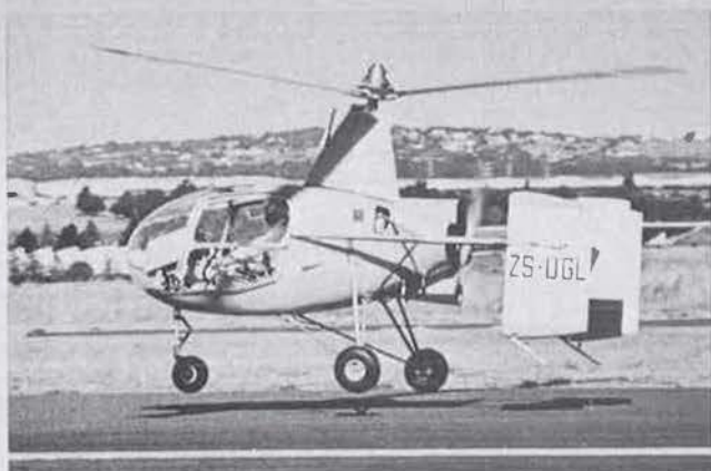
CSIR Experimental Autogyro II (180 hp Lycoming O-360-A engine)
