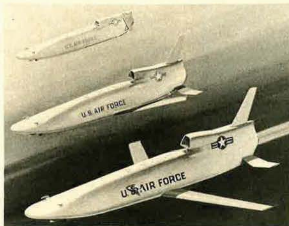
Artist's concept of SCAD sequence, from launch (top) to cruise configuration
