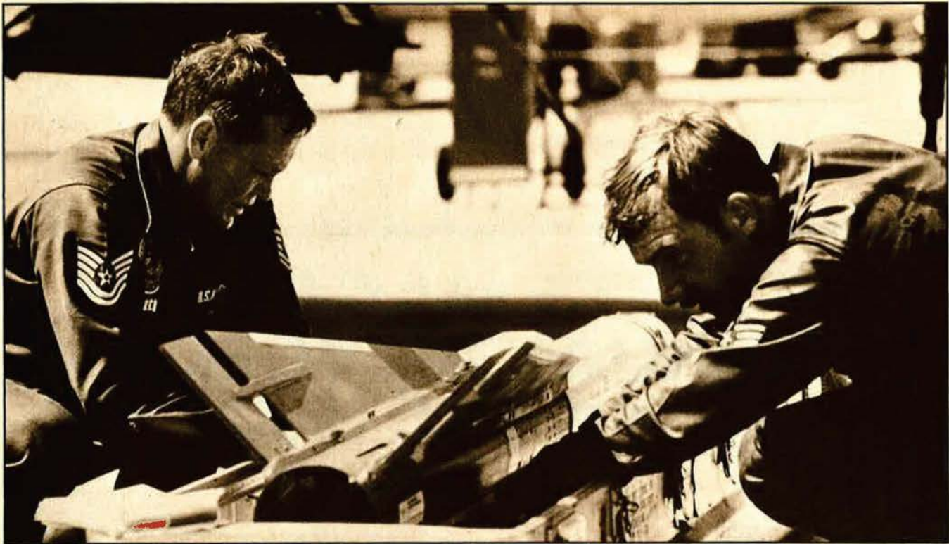
Weapons crew prepares to load a supersonic Falcon air-to-air missile aboard an ADC aircraft.
