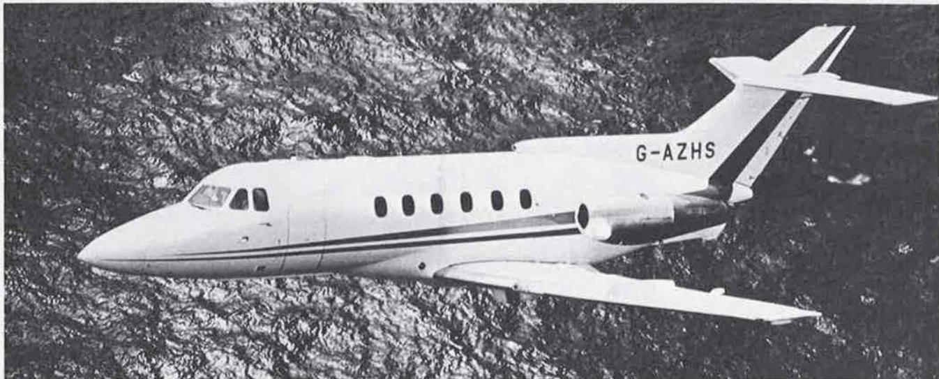
Hawker Siddeley 125 Srs 600A/Beechcraft Hawker BH 125-600 business aircraft (two Rolls-Royce Bristol Viper 601-22 turbojet engines)
