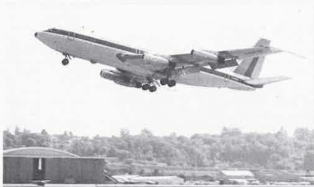
The Boeing 720 test-bed, here taking off, has demonstrated its ability to operate for long periods at low altitude and also to perform well in a high-altitude environment
