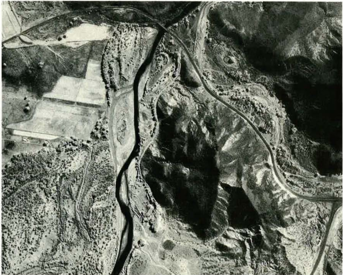
This aerial infrared photo was taken by a WB-57F weather aircraft over northern New Mexico. Note how the trees and other vegetation appear light colored, a characteristic of infrared film due to the high reflectance of foliage in the photographic infrared.
