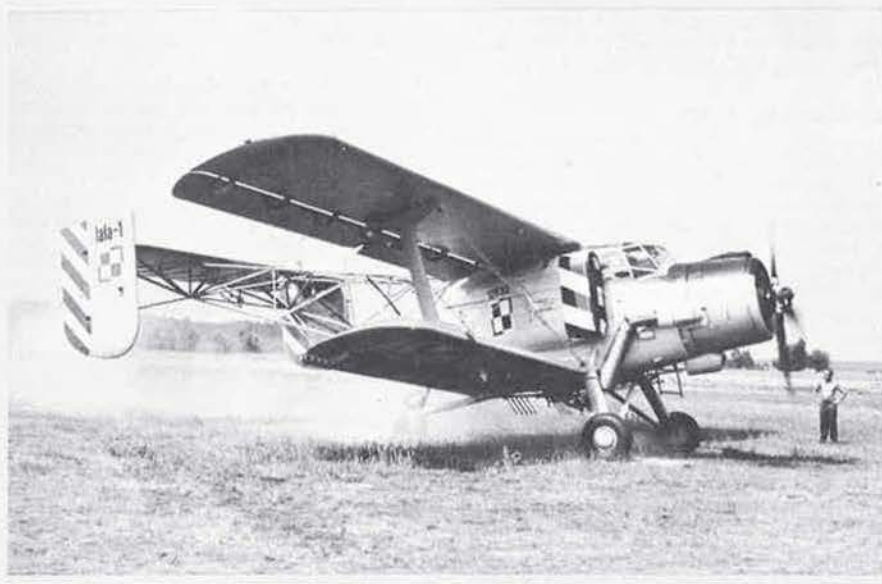
Lala-1 test-bed (1,000 hp Shvetsov ASH-621R radial piston-engine, plus Ivchenko AI-25 turbopfan engine behind crew compartment) (Biil)
