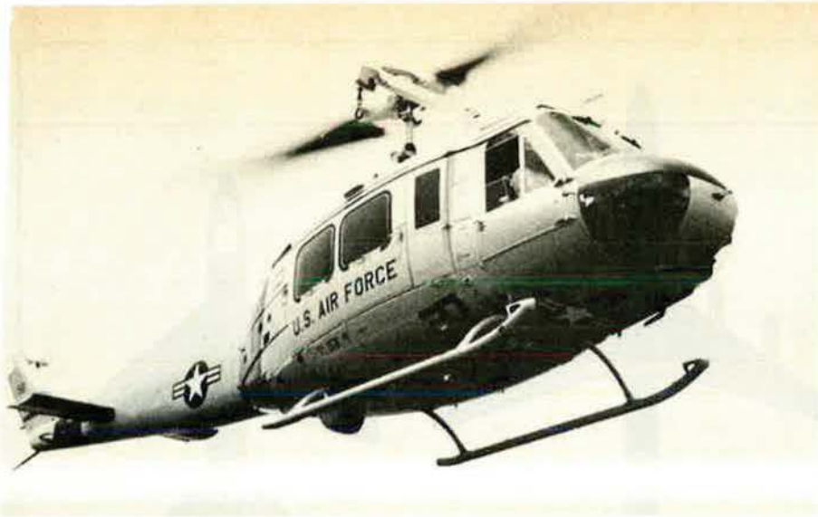
The Air Force has accepted delivery of the first HH-1H Huey helicopter, designed for a rescue role with Aerospace Rescue and Recovery Service units. Built by Bell Helicopter Co., the Huey can carry five passengers and a crew of two.
