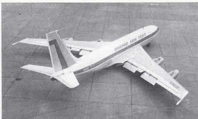
Boeing 720 test-bed modified to demonstrate the potential of the company's ASW projects, which would be based on the generally-similar 707-320C airframe
