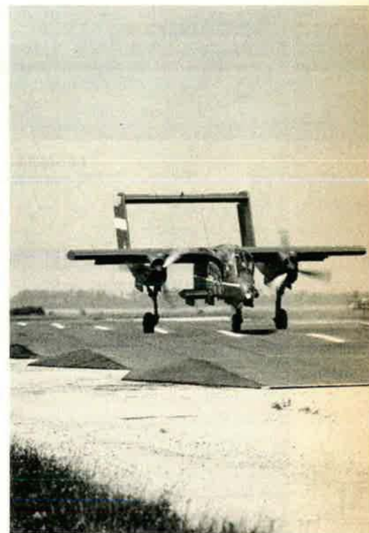
The OV-10's landing gear was tested at ninety-five knots on this torture course.
