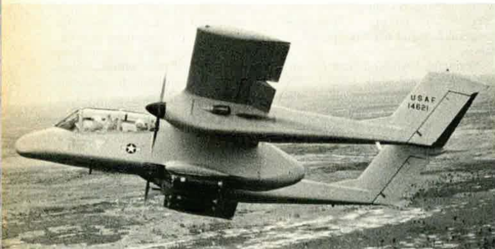
In addition to its four rocket pods, the OV-10 carries four 7.62-mm machine guns—a lot of sting for a “hummingbird.”
