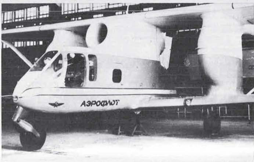
Mock-up of the WSK-Mielec M-15 agricultural aircraft (Ivchenko AI-25 turboprop engine) (Biil)
