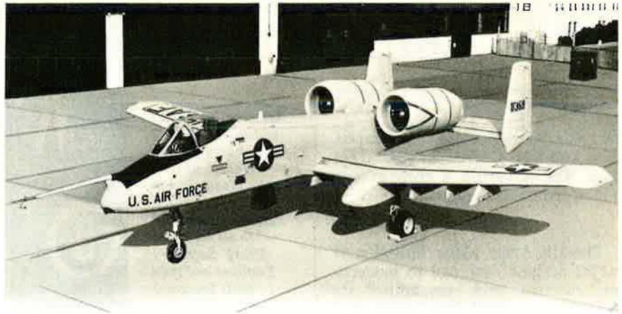
Fairchild Industries' A-10A, the aircraft selected by USAF to fill a close-support role in the future (see item). The A-10A is designed to carry a variety of ordnance, and the production model, if approved, will mount a 30-mm cannon in the nose.
