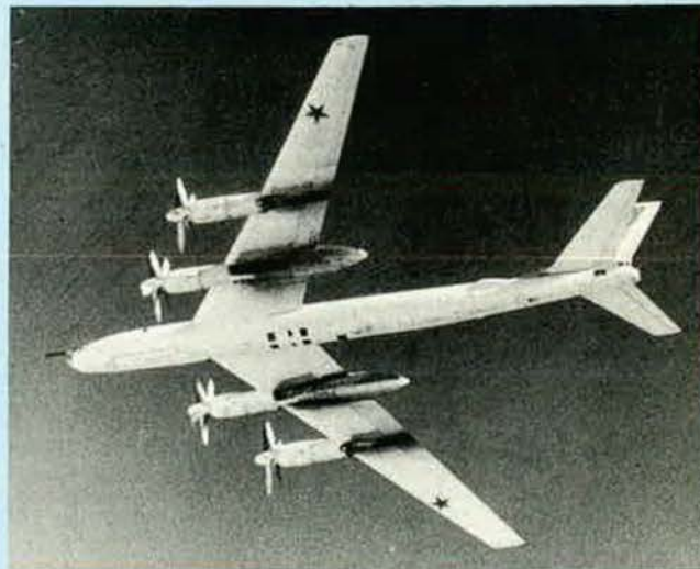
Camera ports under the bomb-bay are a recognition feature of "Bear-E", latest identifiable version of the Tu-95 (Royal Navy)
