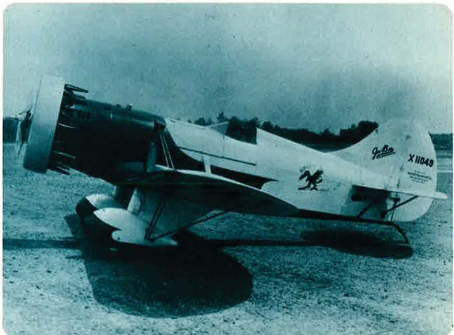
The Granvilles' earlier Gee Bee "Y" version, powered by a Pratt & Whitney 420-hp Wasp engine, could hit speeds of 200 mph.
