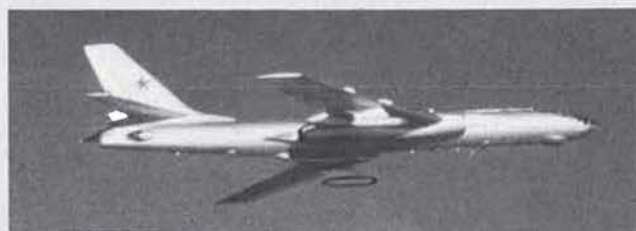
Underwing electronic pods identify this Tu-16 as the "Badger-F" version (Royal Air Force)
