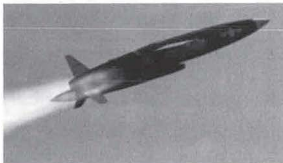
MQM-74/CHUKAR. The first low-cost jet-powered drone.
