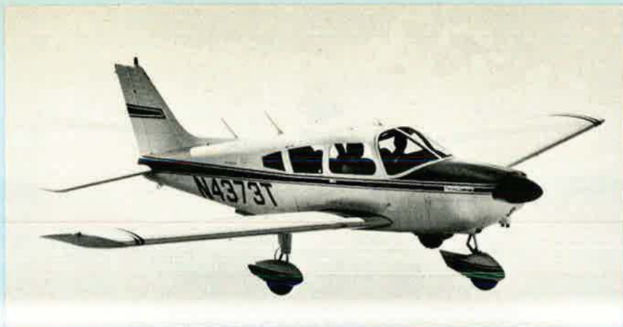
Piper Cherokee Challenger four-seat light aircraft (180 hp Lycoming O-360-A3A engine)
