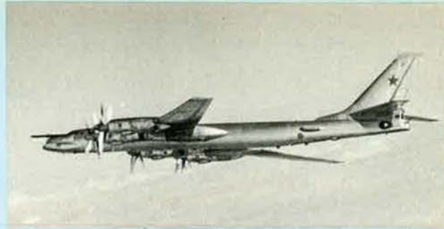
The streamlined blister fairing on the port side of the rear fuselage is a distinguishing feature of "Bear-C" (Royal Navy)
