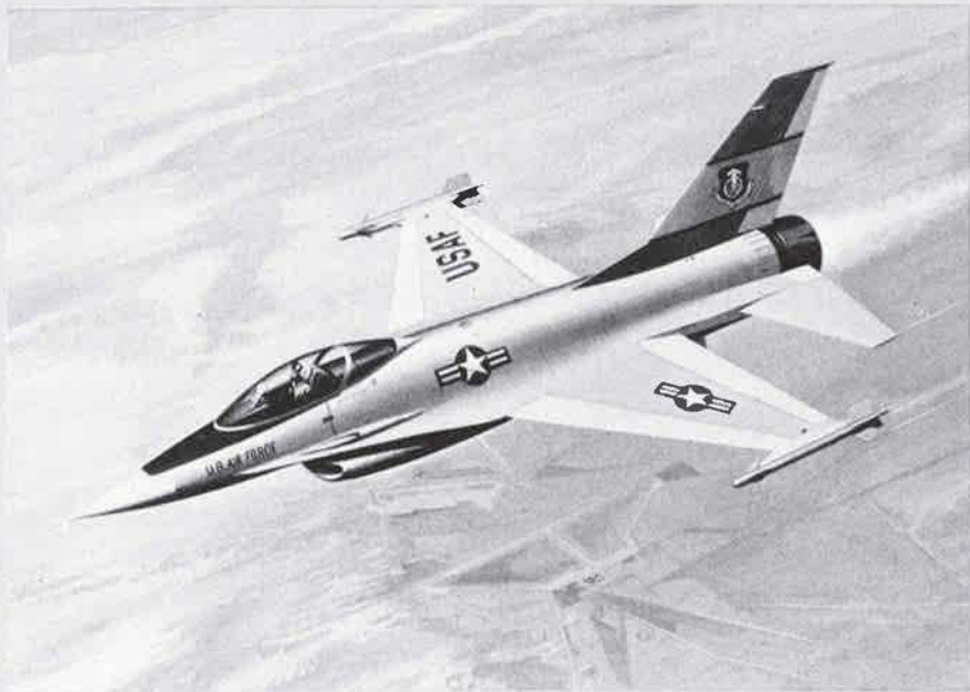
Artist's impression of the General Dynamics YF-16 (Model 401) LWF prototype (one Pratt & Whitney F100-PW-100 turbofan). The outboard wing trailing-edge flaps shown here will no longer be fitted
