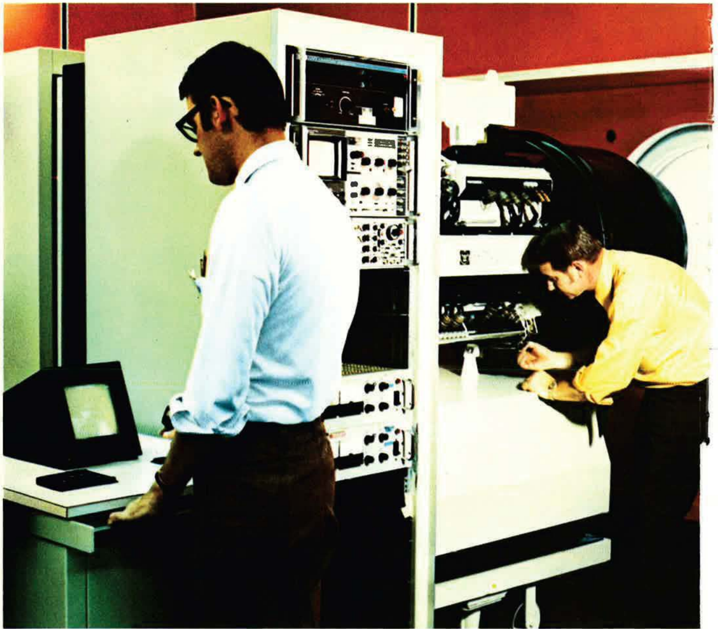
The WX-200 radar in system test. The radar is coherent, and provides a "Clean Scope."
