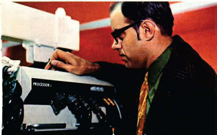
Unique programmable signal processor allows changes in radar characteristics via software.
