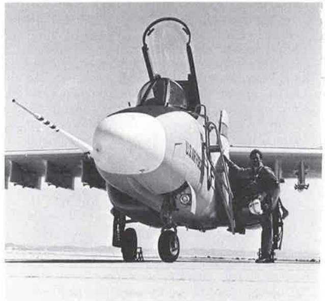
Northrop's A-X prototype—the A-9A—like its Fairchild competitor will carry up to eight tons of ordnance and a new 30-mm cannon.
