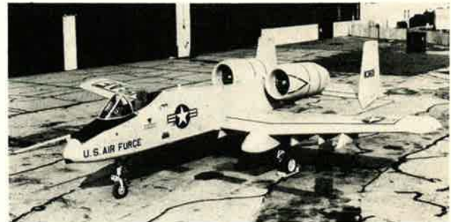
fifty-eight feet. Above right is the A-10, built by Fairchild Industries' Republic Division at Farmingdale, N. Y. It is fifty-two feet, seven inches in length, fourteen feet, 5.5 inches in height, and has a wingspan of fifty-five feet. USAF's Aeronautical Systems Division at Wright-Patterson AFB, Ohio, manages the A-X program.
