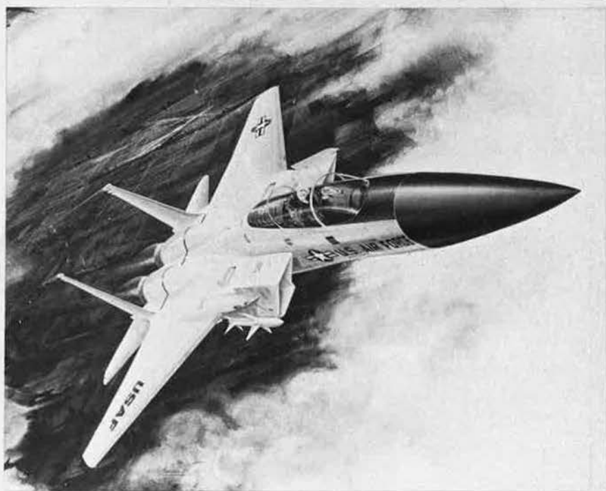
Artist's impression of the McDonnell Douglas F-15A (two Pratt & Whitney F100-PW-101 turbofan engines)
