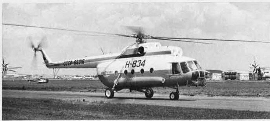
Mil Mi-8 transport helicopter, powered by two Isotov TV2-117A turboshaft engines (Air Portraits)
