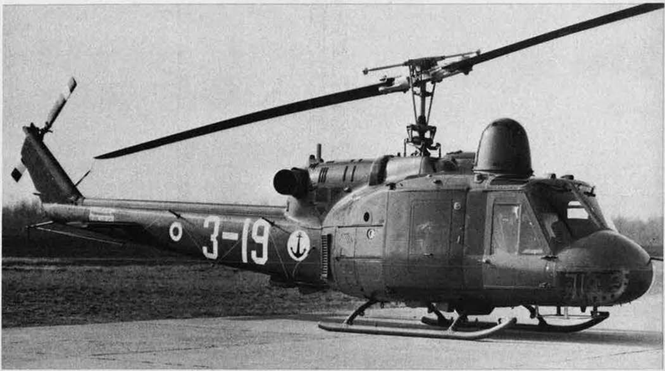
Agusta-Bell 204AS, the licence-built ASW helicopter which the AB 212AS is intended to replace
