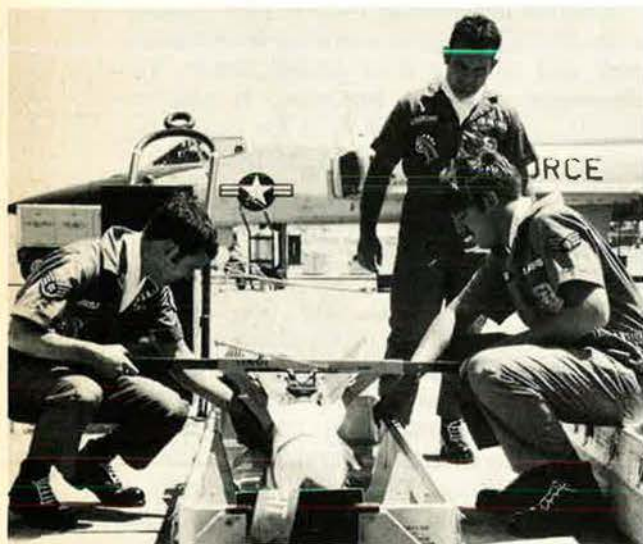
Ground crews of the 43rd Fighter Interceptor Squadron, winner of the Hughes Trophy, prepare an AIM-4 missile for removal from storage containers and loading aboard a waiting F-106.
