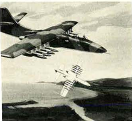
Northrop Corp. entry into competition for Air Force A-X contract has engines in wing root, conventional tail. This is artist's concept of how it will look.
