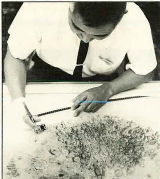
The airbrush technique is used to create the crater features of the lunar surface on a precisely detailed charting product.
