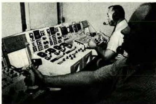
The AN/TSW-10 control station commands multiple RPV's at more than 250 nautical miles. It is one of five Motorola-built control stations, part of an integrated drone control system, AN/USW-3.
