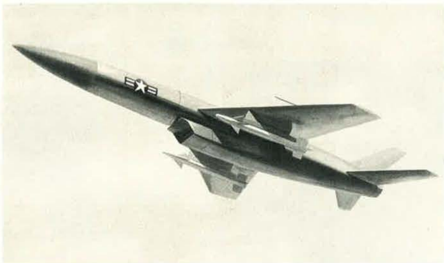
An artist's conception of a Remotely Piloted Vehicle (RPV) proposed for air-to-air combat missions (see Senior Editor Edgar Ulsamer's article on the subject, October '70 issue, p. 40). This is one of Northrop Corp.'s several designs for the RPV. Military planners see RPVs performing a number of combat missions, including air-to-surface attack, recce, and interdiction.
