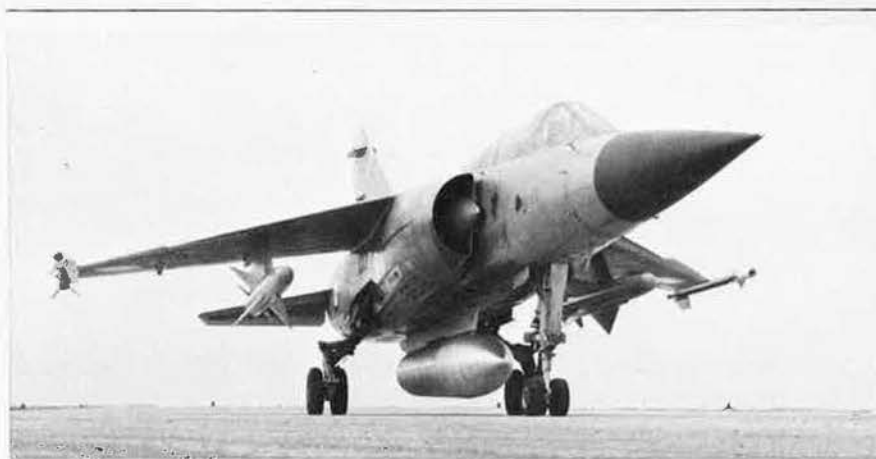
Dassault Mirage F1, carrying one 1,200 litre external fuel tank, two Matra R.530 and two Sidewinder air-to-air missiles
