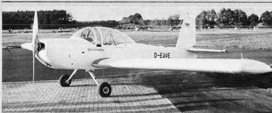
FLUWAG Bremen ESS 641 single-seat glider tug (180 hp Lycoming O-360-A3A engine)
