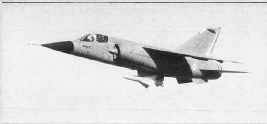
Dassault Mirage F1 in interceptor configuration, with under-fuselage Matra R.530 missile
