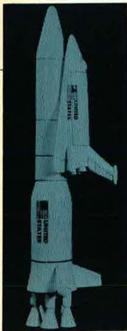
The McDonnell Douglas/Martin Marietta proposal for a recoverable, liquid-fueled rocket booster.
