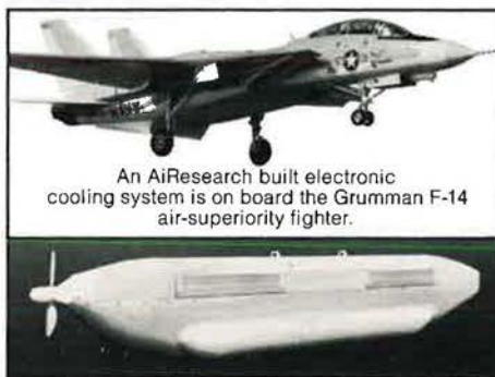
The ALQ-99 electronic countermeasure system is powered by an AiResearch RAT and cooled by our system.
