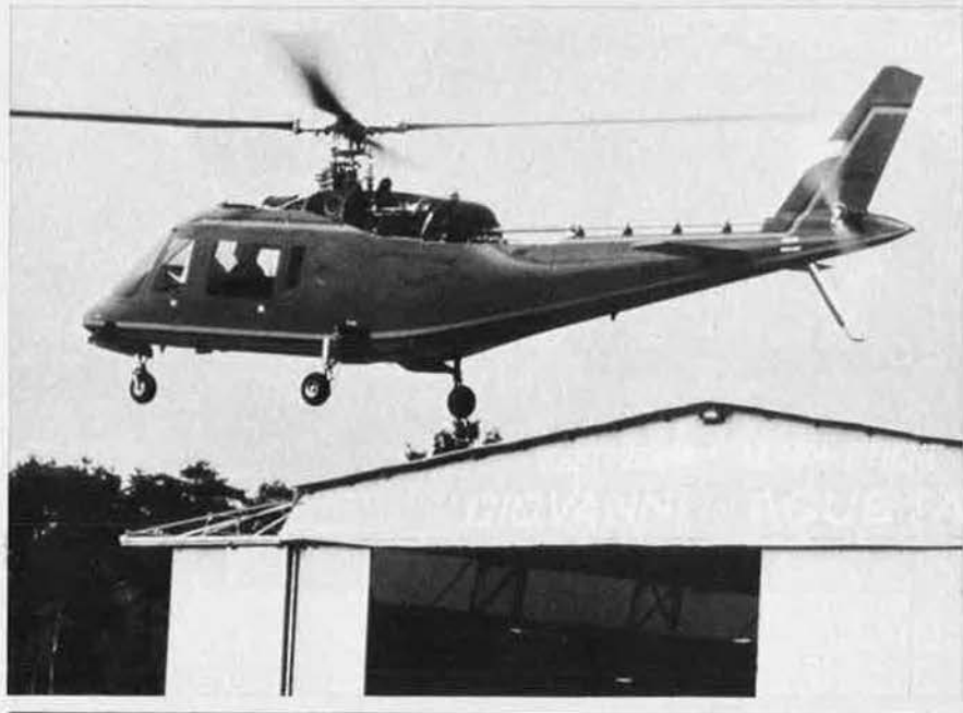
The prototype Agusta A 109 Hirundo as first flown, without engine cowlings and fairing over tail rotor shaft
