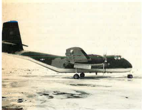
Joining the Air Force Reserve inventory is the versatile C-7 Caribou, a STOL utility transport that has seen extensive service in Vietnam, airlifting troops and equipment to isolated landing fields.
