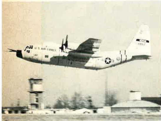
Search range and emergency response time will improve for the Reserve units reequipping with the HC-130, a modified version of the Hercules transport especially designed for rescue and recovery operations.
