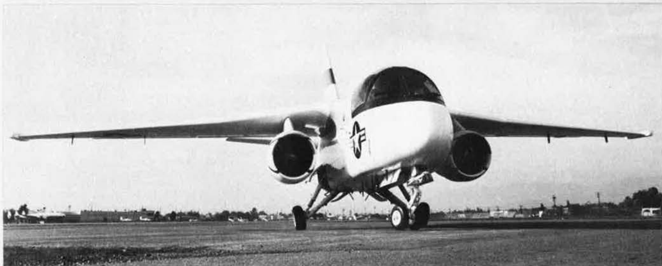
The first of eight Lockheed S-3A Viking research and development aircraft (two General Electric TF34-GE-2 turbofan engines)
