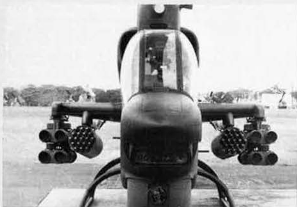
The KingCobra combines the slim profile of the AH-1J and AH-1G with new nose sensors and heavier armament
