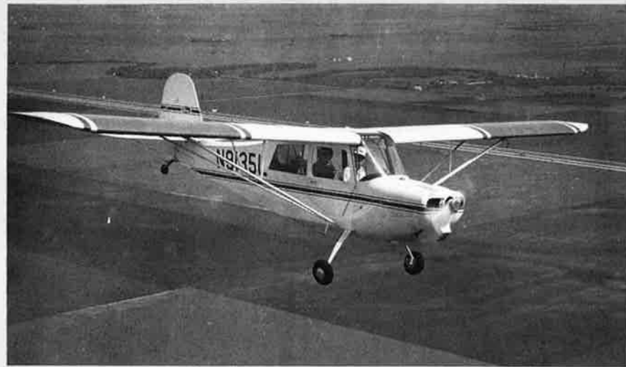
Bellanca (Champion) 7AC Champ two-seat lightplane (60 hp Franklin 2A-120-B engine) (Don Downie)
