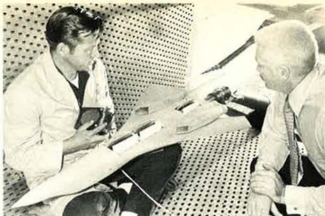
AF Systems Command's Arnold Engineering Development Center was the scene of wind-tunnel tests for launch of Short Range Attack Missile from B-1 bomber. For a story by Senior Editor Edgar Ulsamer on SRAM capabilities, see p. 28.
