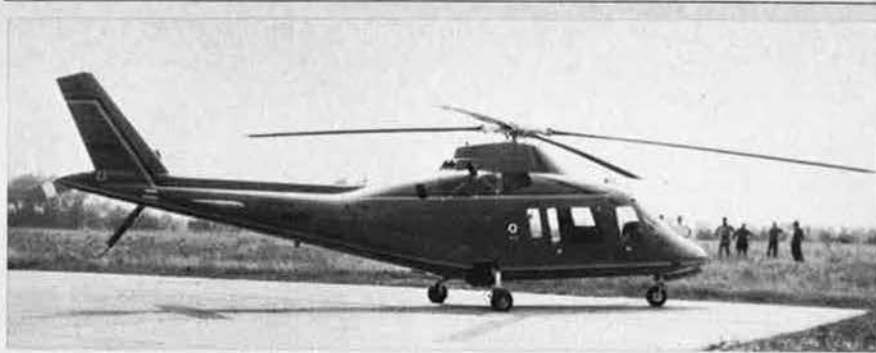
First prototype of the Agusta A 109 Hirundo (two 400 shp Allison 250-C20 turboshaft engines)
