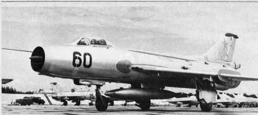
A Sukhoi Su-7, most successful of the many Soviet designs that have been powered by Lyulka turbojets (Tass)
