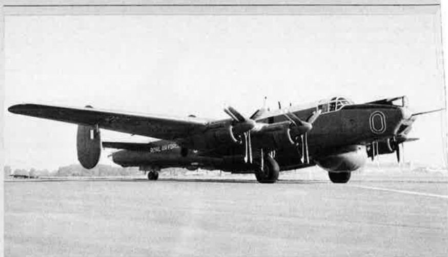
The Shackleton Mk 2 is the only British operational aircraft that is piston-engined and fitted with a tailwheel landing gear
