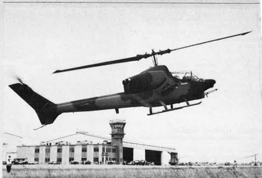
The first prototype of the Bell KingCobra armed helicopter (1,800 shp Pratt & Whitney T400-CP-400 coupled turboshaft)
