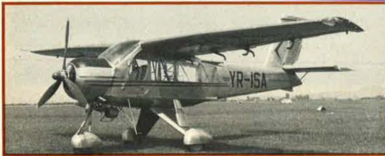
Romania's contribution to the general-purpose light STOL aircraft category is this IAR-23-A, first flown in 1967.
