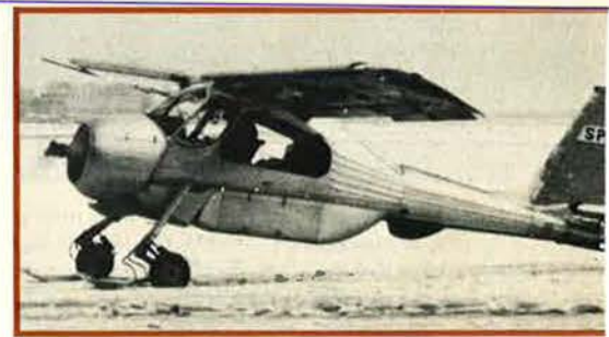
Poland's PZL-104 Wilga 40 general-purpose aircraft has several unique features, such as detachable cargo container and skis.
