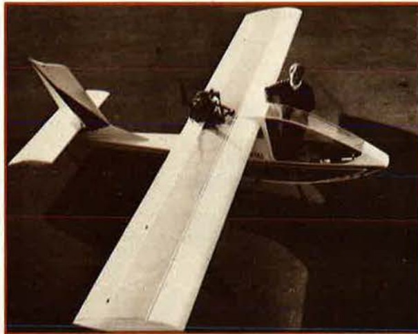
Poland's Janowski J-1 Przasniczka is an ultralight, single-seat aircraft that has been designed specifically to be built at home by a do-it-yourselfer. It has a range of about 250 miles.
