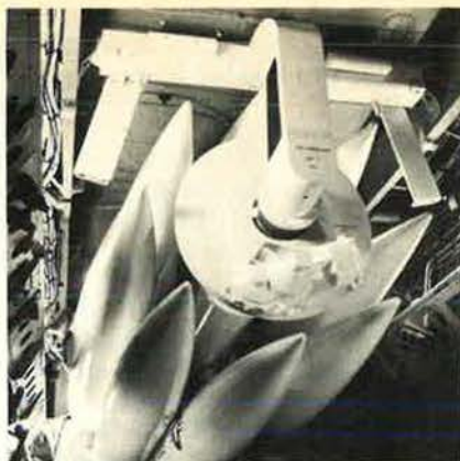
Eight new Short-Range Attack Missiles (SRAM) in rotary, rapid-launch configuration for installation aboard B-52s.
