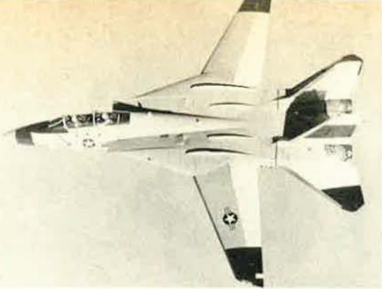
The US Navy's controversial F-14 fighter, now in its test stage, is shown here with its swingwing fully extended. It is designed as a carrier-based air-superiority fighter.
