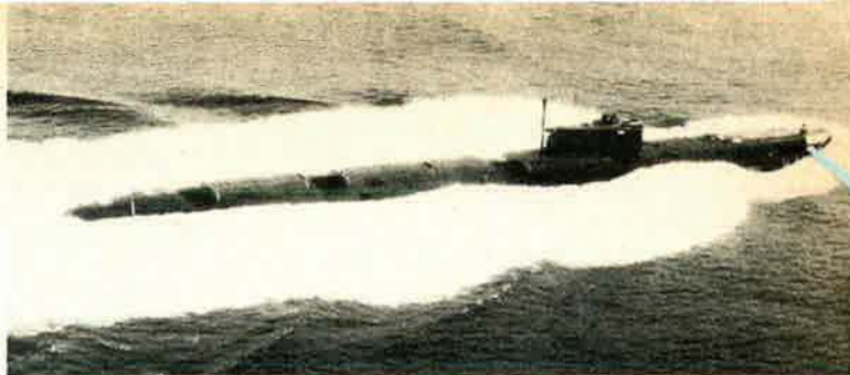
One of the USSR's 5,000-ton Echo II-class nuclear-powered submarines on exercises in the North Pacific. The submarine carries eight cruise missiles and a crew of 100.
