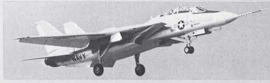
Grumman F-14A Tomcat (two Pratt & Whitney TF30-P-412 afterburning turbofan engines)
