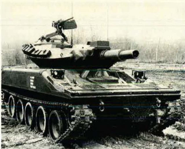
A General Sheridan armored reconnaissance vehicle equipped to launch the US Army's Shillelagh missile. The missile, effective against armor, fortifications, or troops, is forty-five inches long and about six inches in diameter.
