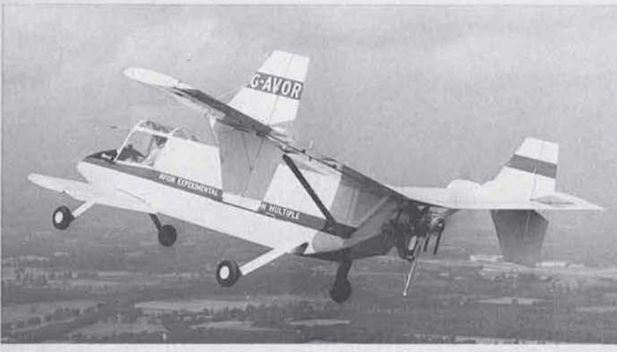
The prototype Lockspeiser LDA-01 (85 hp Continental C85-12 engine)
