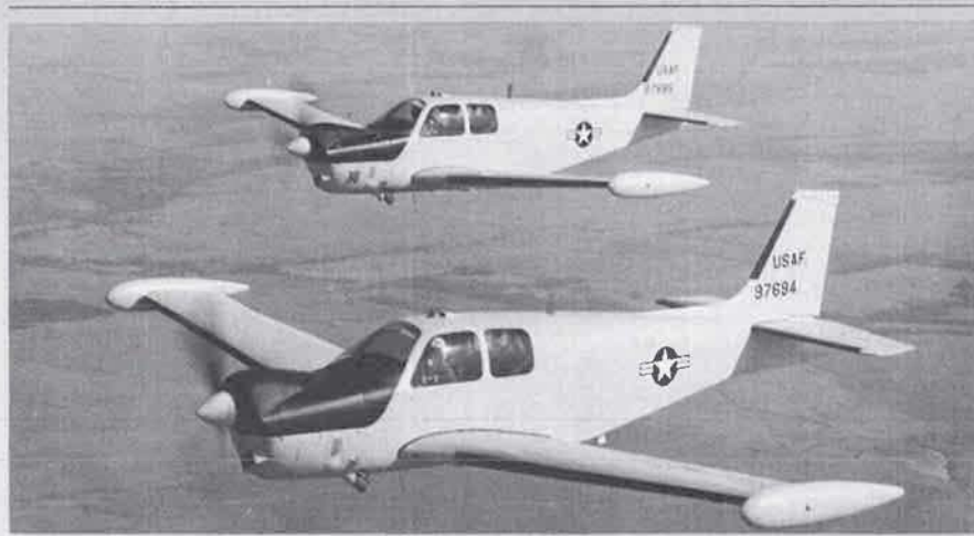
Beechcraft QU-22B version of the Model 36 Bonanza utilised under the USAF's Pave Eagle reconnaissance project
