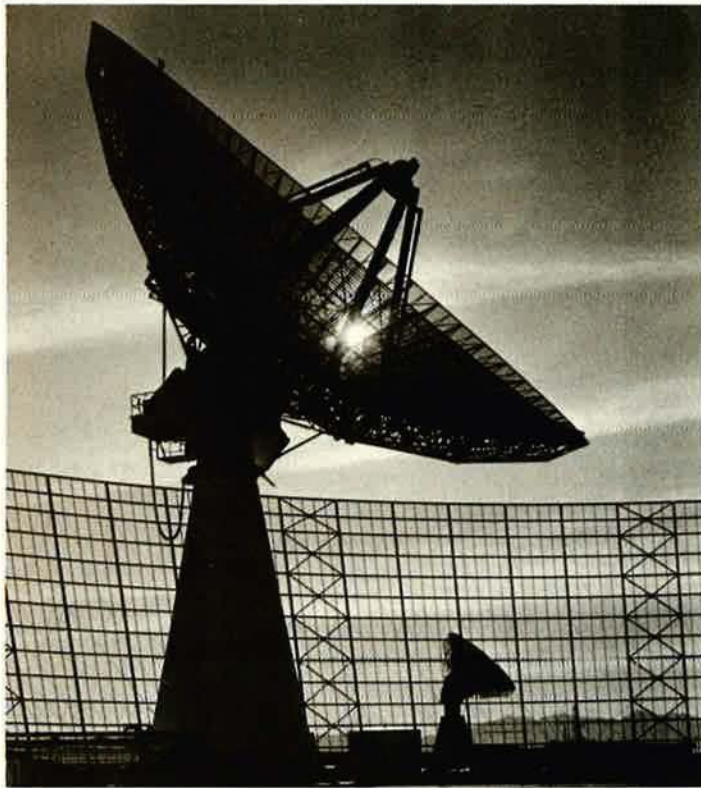
Reentry behavior of ABRES test vehicles is being recorded at White Sands Missile Range in New Mexico by specially shielded radar systems.
