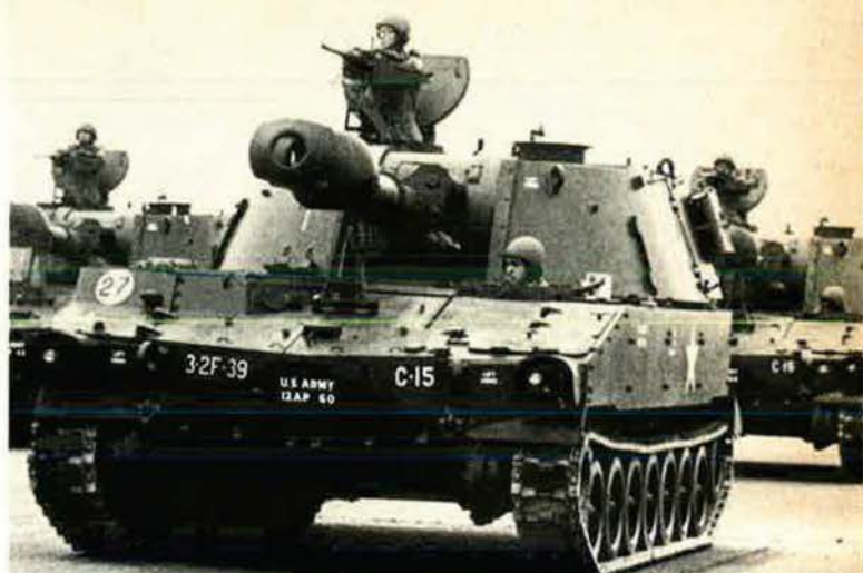
The 155-mm howitzer, mounted on a US Army M-109 self-propelled vehicle, swings in a full circle and can be elevated from minus three degrees to plus seventy-five degrees. Here it is seen in review at Kitzingen Airfield, Germany.
