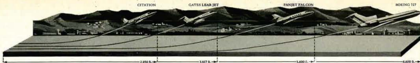
Distance it takes various jets to reach an altitude of 35 ft. at maximum gross weight; a principal measurement of balanced field length.
