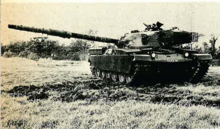
The Chieftain tank, mounting a 120-mm gun, is used exclusively by Great Britain. The first of the Chieftains was issued to the Army in 1965. British armored capability relies on the Chieftain and the smaller Centurion, 900 of them in all.
