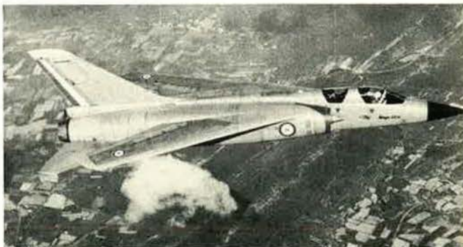
In its fourth flight—and four days after its maiden flight—the French Mirage G8 reached speeds of Mach 2.03 with wings in the fully swept configuration. The flight was in May 1971.
