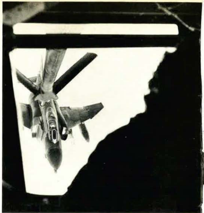
F-4 fighter aircraft, used by both the US Air Force and Navy, are deployed in Europe and the Pacific area. This F-4 is refueling from an Air National Guard KC-97 over Germany.
