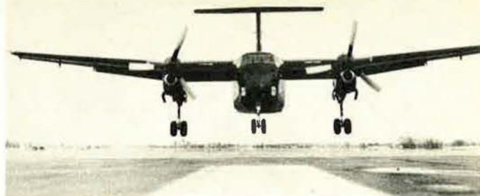
The de Havilland Canada Buffalo is powered by two General Electric T64s. This 41,000-pound STOL transport has a ground roll of only 800 feet for takeoff, 710 feet for landing.
