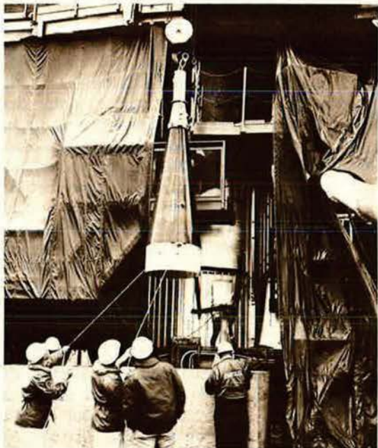
A technologically advanced, slender reentry vehicle is being hoisted for mating with an Atlas 134 ICBM and subsequent test launch.
