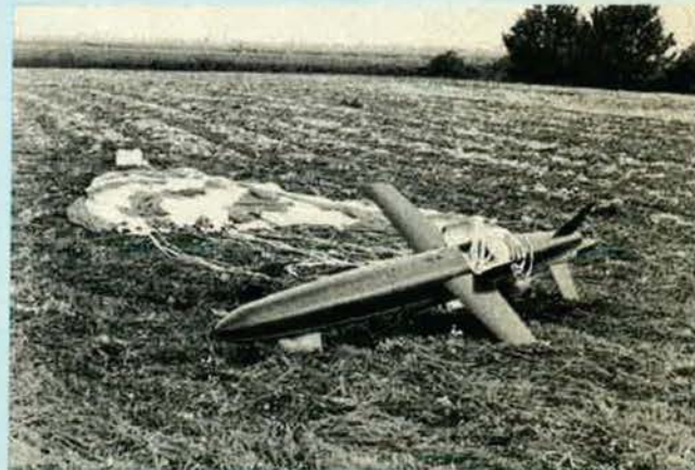
At left, below, Meteor Gufone tactical surveillance drone on its launcher, towed by a launch truck (LTK). Right, below, photo shows the Gufone's recovery 'chute and the air-bags which cushion the landing shock
