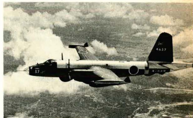
The Japanese Air Force Kawasaki P-2J patrol aircraft is built in Japan, based on the design of the Lockheed P-2V, a US Navy patrol bomber.
