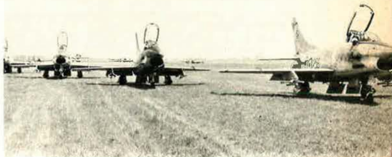
Fiat G-91 lightweight ground support and attack fighters of the Italian Air Force can operate from sod fields. The Italian Air Force has some 300 combat aircraft and a personnel strength of 74,000.
