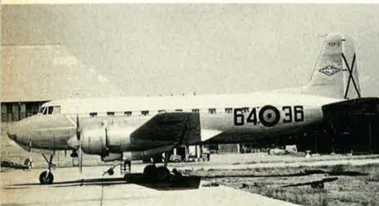
The CASA 207, which carries the Spanish Air Force designation T-7, has been built in both troop and military cargo transport versions. Passenger capacity is thirty to forty.
