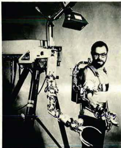
A "slave arm" that follows directions of its counterpart on a human arm gets its orders via three-dimensional TV system. It was developed by MBAssociates, under Navy/NASA/AEC contract.
