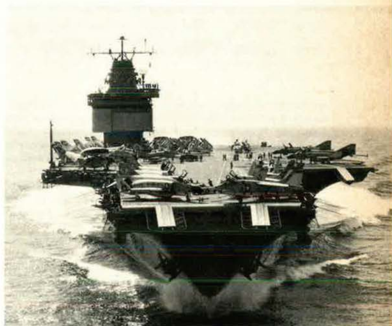
The US Navy's huge nuclear-powered aircraft carrier, USS Enterprise, carries about 100 planes of various types. The Enterprise, equipped with an automated combat direction system for command and control, has contributed much to the air action in Southeast Asia.
