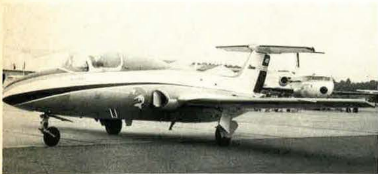
The L-29, a jet trainer designed and built in Czechoslovakia, has become the principal trainer for the Warsaw Pact air forces. More than 2,500 have been built. Shown here is the L-29A, a single-seat acrobatic version.
