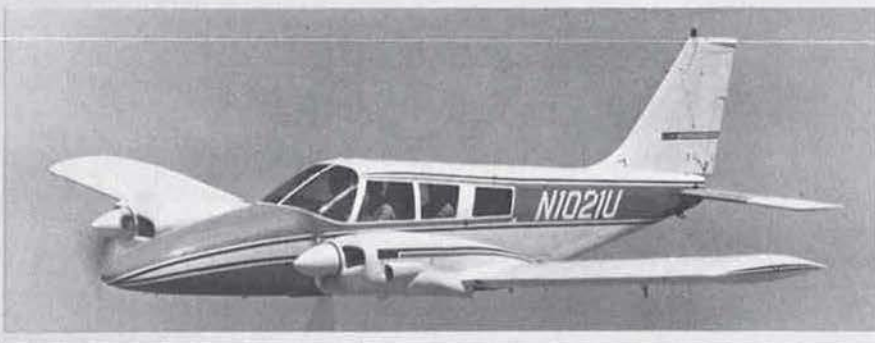
Piper PA-34 Seneca (two 200 hp Lycoming IO-360 engines)
