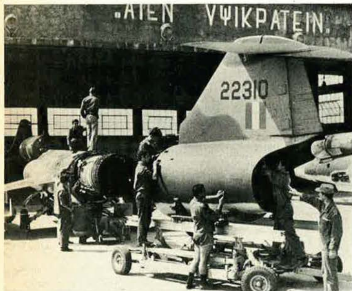
Greek Air Force mechanics perform nose-to-tail maintenance on a dismantled Lockheed F-104 fighter. As in all air forces, maintenance is the key to operational success.
