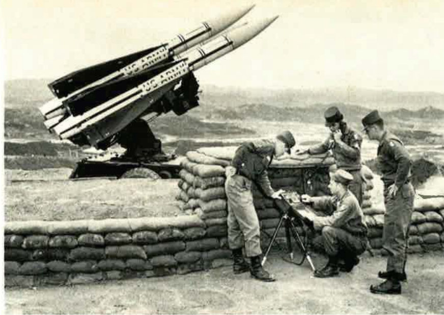
The US Army's Hawk air defense missile is a solid-propellant, two-stage, mobile system, highly effective against aircraft flying at medium altitude or as low as 100 feet above the ground.
