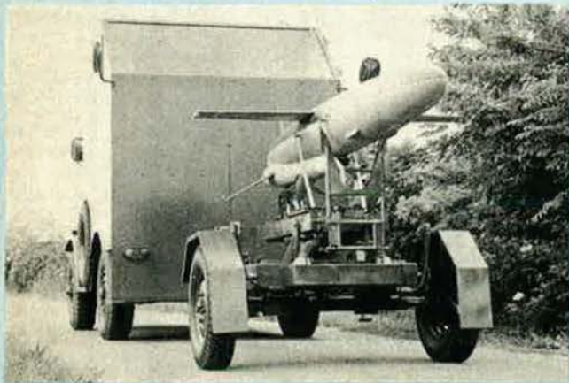
At left, below, Meteor Gufone tactical surveillance drone on its launcher, towed by a launch truck (LTK). Right, below, photo shows the Gufone's recovery 'chute and the air-bags which cushion the landing shock
