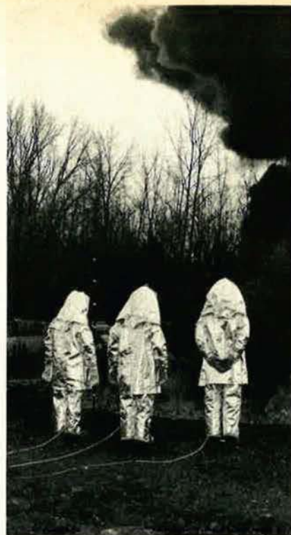
Jet fuel burns furiously during a test of various aluminized asbestos fire-fighting clothing. Note the instrumentation cables attached to the suits. Data gathered from the tests will help in designing more effective protective gear for both military and civilian use in combating blazes. Aircraft fires, because of inherent fuel stores, are particularly hazardous.
