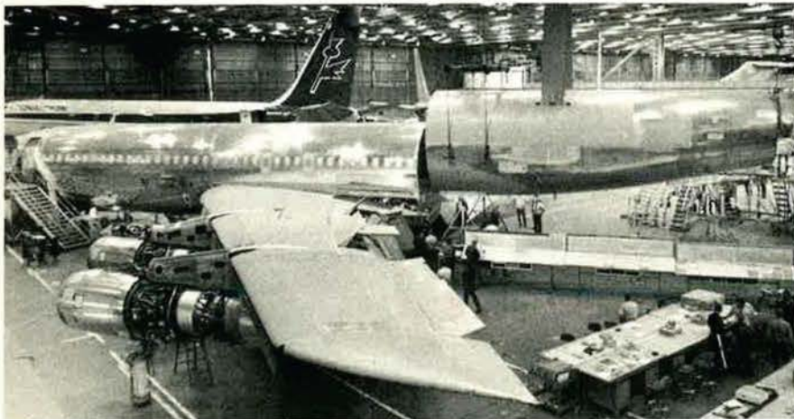
AWACS is beginning to shape up. Here, the fuselage section to support the huge radome is joined to the forward section at Boeing Co.'s Renton, Wash., plant.
