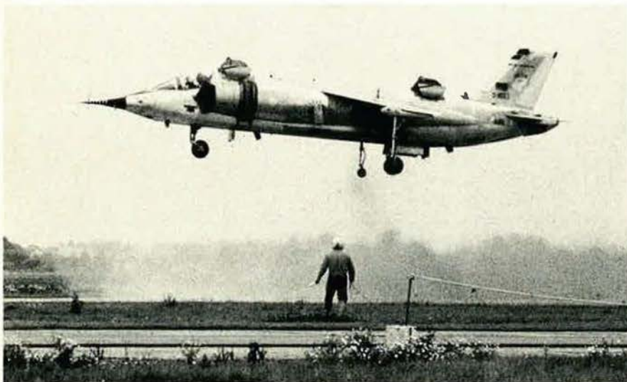
VFW-Fokker's VAK 191 B V/STOL strike aircraft flew for the first time in mid-September. The West's only other STOL aircraft in service is Britain's Harrier.
