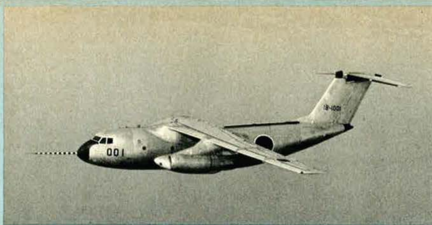
NAMC XC-1 military transport (two Pratt & Whitney JT8D-9 turbofan engines)
