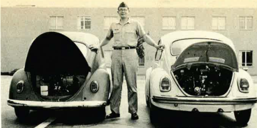
Six golf-cart batteries make up the powerplant for Air Force Capt. Joe Allred's "electromobile" on the left. (A normal VW is on the right.) He built the electric power system into his 1962 Volkswagen in his spare time. Its range is about fifteen miles, and the batteries take about four hours to recharge. Top speed of the electromobile is forty mph. Captain Allred is stationed at Hanscom Field, Mass.
