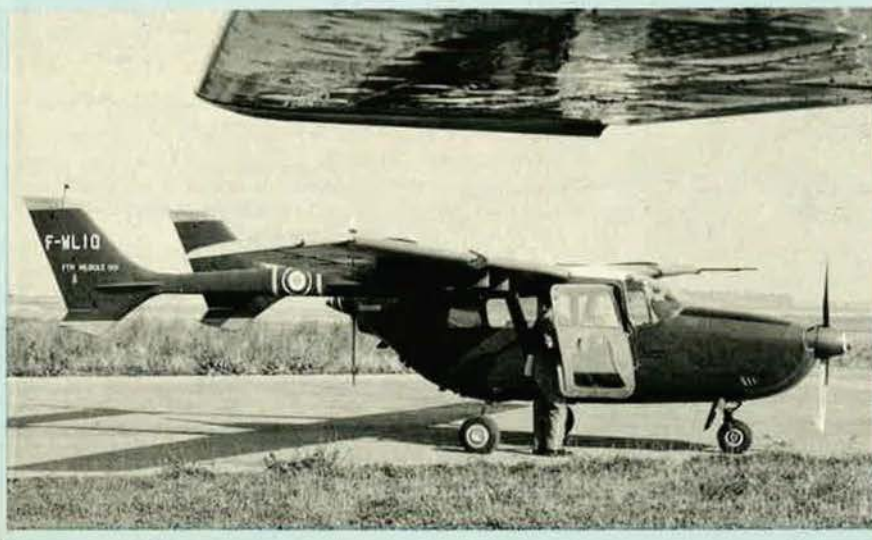
Prototype Reims-Cessna FTMA-Milirole (two 210 hp Rolls-Royce/Continental TS10-360-A engines)
