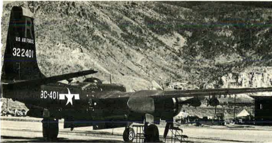
During the Korean War, B and C models of the Invader, now designated B-26, once more saw service. This Korean C with H2S radar was used for night bombing.
