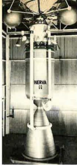
NERVA, a joint AEC-National Aeronautics and Space Administration program, is a nuclear-powered rocket for deep-space missions or long-duration orbital applications. Shown here at the Nuclear Rocket Development Station, Nev., NERVA produces up to 75,000 pounds of thrust in the vacuum of space by pumping super-cold liquid hydrogen through its nuclear reactor, where it is heated to very high temperatures so that it will expand with high energy through the nozzle.
