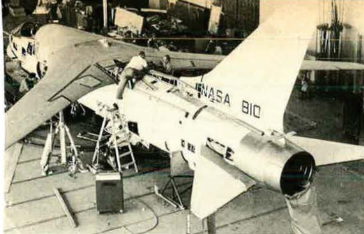
A supercritical wing, developed at NASA's Langley Research Center under the direction of Dr. Richard T. Whitcomb, is shown being installed on a modified LTV F-8, which subsequently attained speeds of Mach 1.15. Supercritical technology delays the drag rise associated with supersonic airflow until well into the transonic regime.
