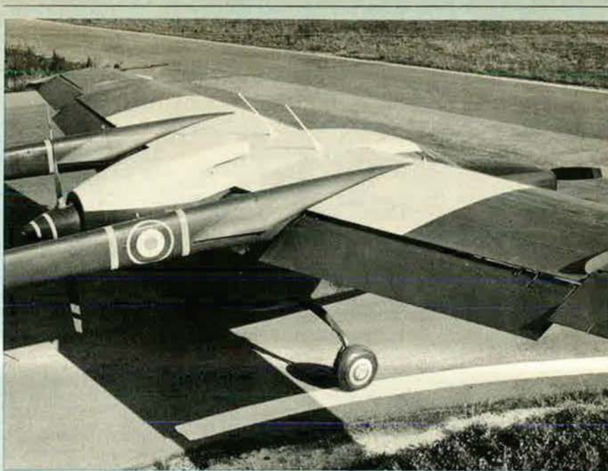
High-lift trailing-edge flaps of Reims-Cessna FTMA-Milirole general-purpose military aircraft
