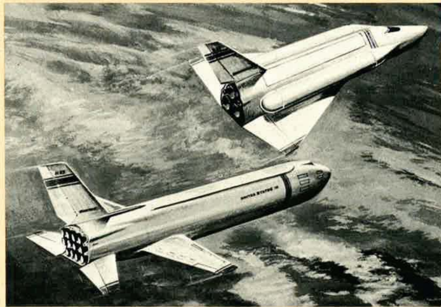
Reusable booster and orbiter, shown following separation, are fully flyable in the atmosphere to meet military requirements.
