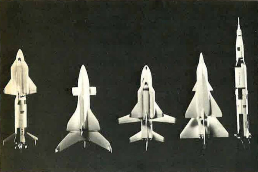
Saturn V, the workhorse of the Apollo moon-landing program, which has a payload capability for near-earth orbits of about 280,000 pounds, is shown here, towering above four Shuttle configurations that are currently under review as part of NASA's examination of phased versus concurrent system development. Shown from left to right are: Saturn IC expendable booster deploying an orbiter stage using external hydrogen tanks, as proposed by Grumman; a fully reusable booster-orbiter combination based on a McDonnell Douglas design; a Grumman orbiter with external tanks and a reusable booster; and a reusable North American orbiter and booster system.
