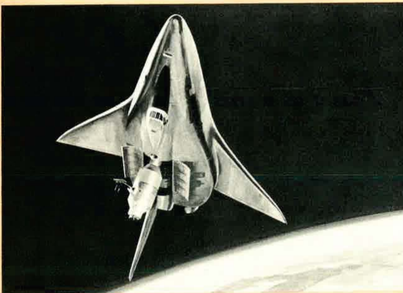
Orbiter stage is shown here delivering a space station module into orbit from its cylindrical payload bay.
