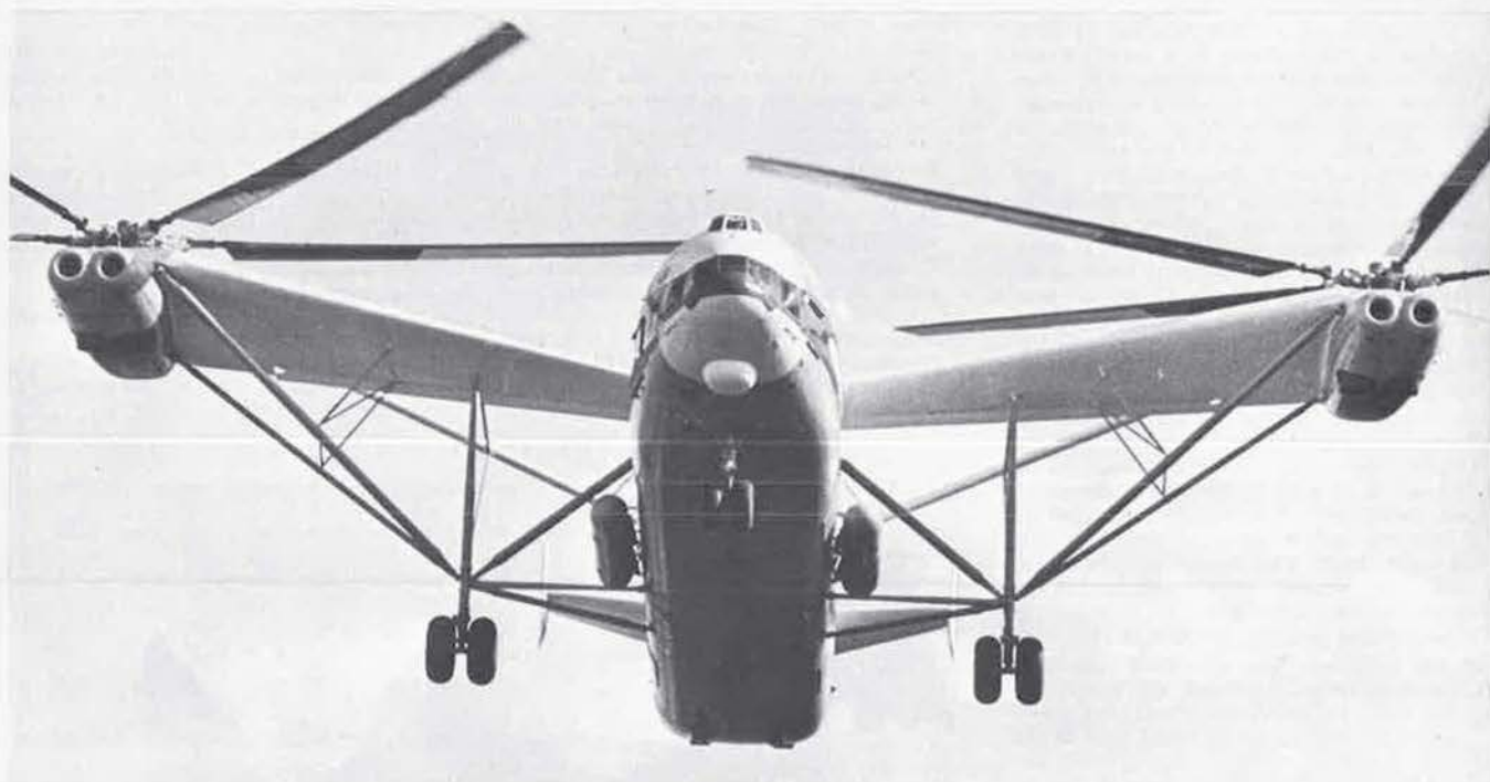
Head-on view of Mil V-12 (Mi-12) heavy-duty transport helicopter (four 6,500 shp Soloviev D-25VF turboshaft engines) (Tass)
