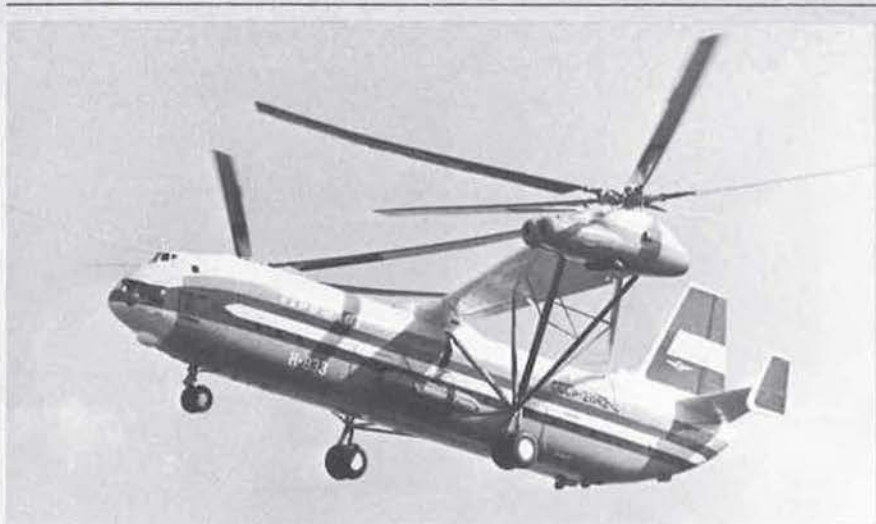
Mil V-12 (Mi-12) heavy-duty transport helicopter in flight (four 6,500 shp Soloviev D-25VF turboshaft engines) (Tass)
