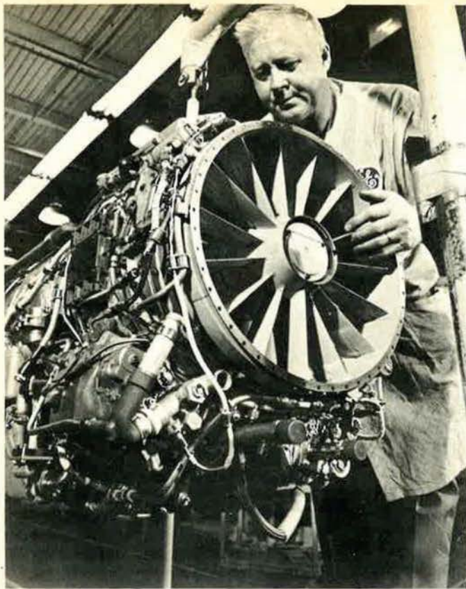
The T-38's two J85 engines, each with 3,850 pounds of thrust, give it supersonic performance and a phenomenal rate of climb. These engines now have logged some four million flight hours.
