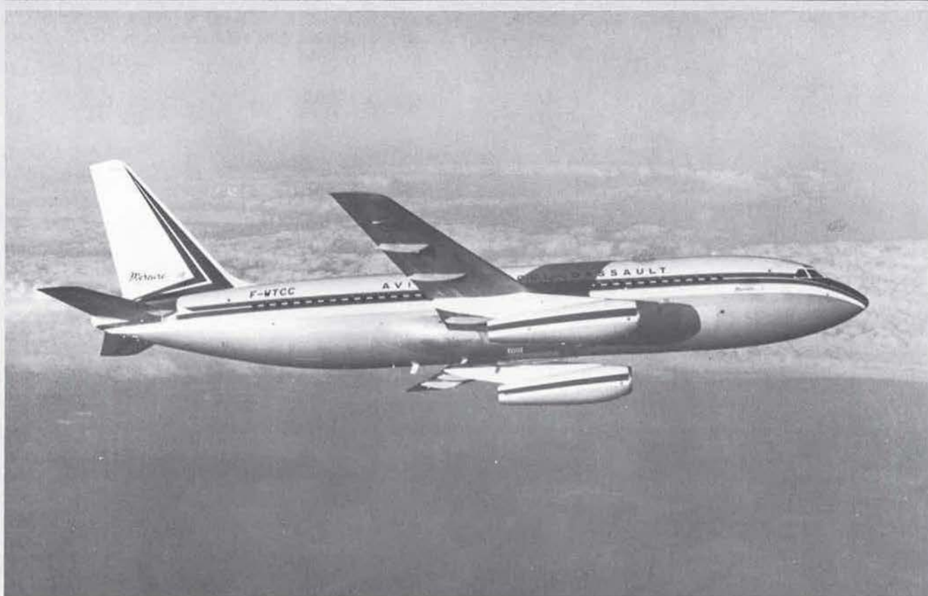
Aerial view of Dassault Mercure prototype high-capacity short-haul transport (two Pratt & Whitney JT8D-11 turbofan engines)
