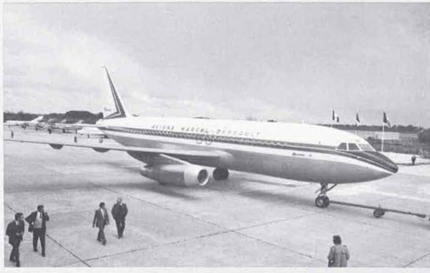
Dassault Mercure prototype high-capacity short-haul transport (two Pratt & Whitney JT8D-11 turbofan engines)
