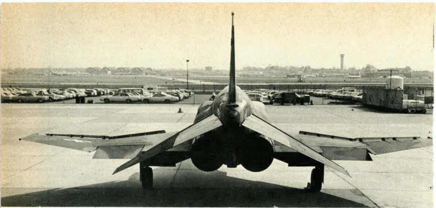
Experimental leading-edge slats give this F-4E the ability to maneuver at angles of attack well beyond the stalling point of an unmodified F-4E—with less power and with little buffet.
