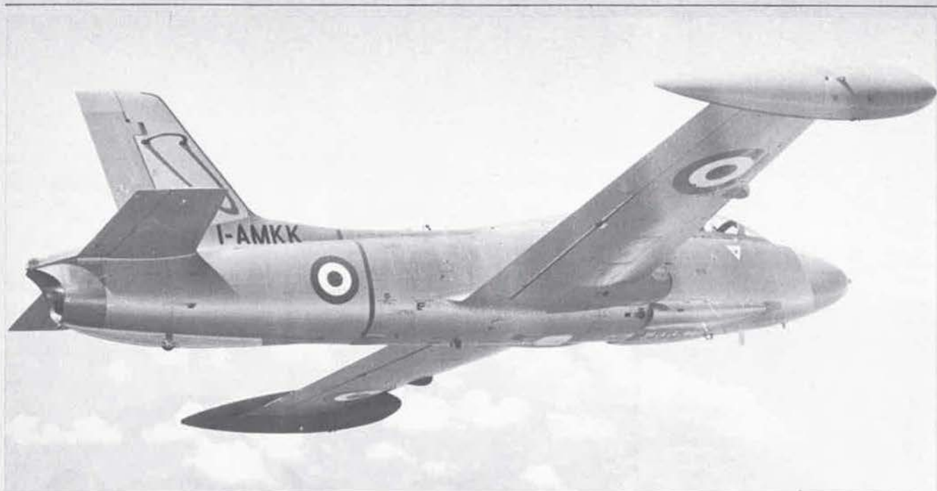
Prototype Aermacchi M.B. 326K single-seat operational trainer and light ground attack aircraft
