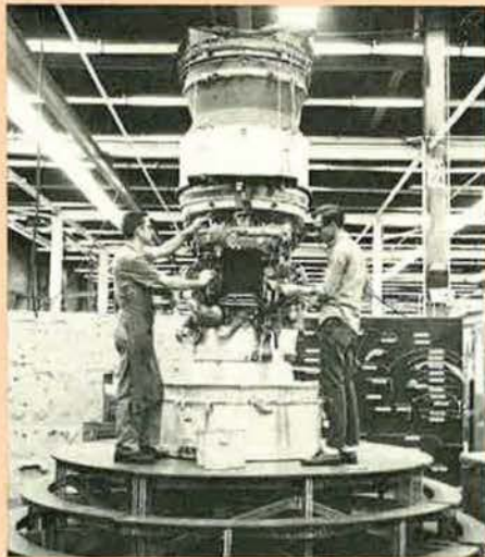
Left, mechanics repair a Liberty-12 engine at Rockwell Air Depot in the late 1920s. Right, a Pratt & Whitney TF33 engine being overhauled at AFLC's Oklahoma City facility. The TF33, used by the B-52H and other USAF aircraft, exceeds the Liberty in power and complexity by orders of magnitude.
