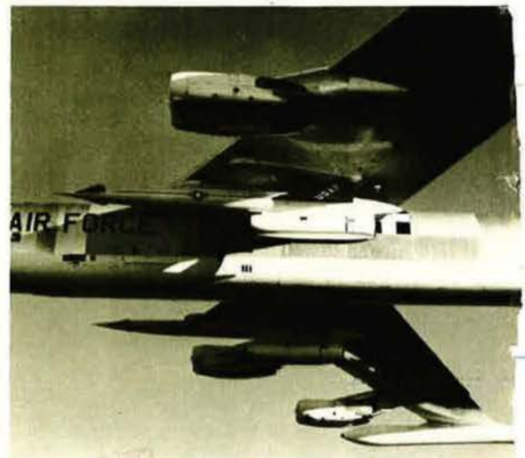
The B-52, shown here with two Hound Dog missiles, has been able to accept the increased volume, weight, and power requirements of new electronic systems, thus extending its operational life.
