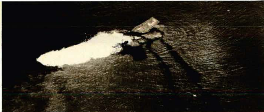
The ruggedly built aircraft carrier Saratoga , anchored more than 500 feet from Zeropoint, finally sank seven and a half hours after the Baker shot.
