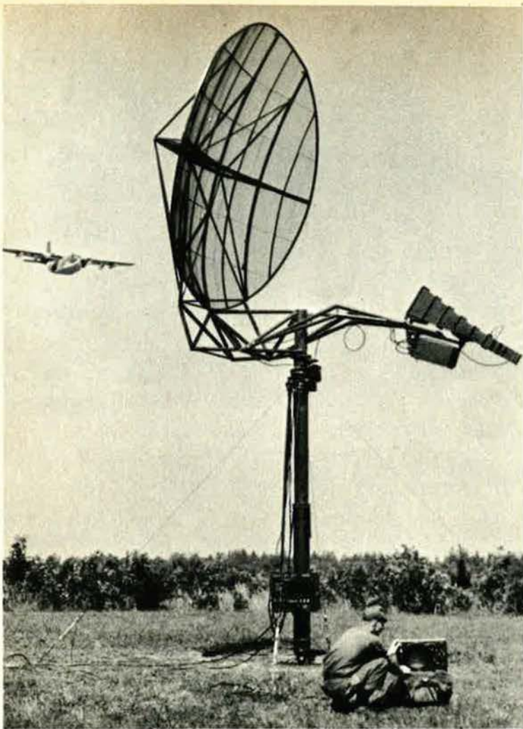
This lightweight, air-transportable, solid-state electronics radar weighing less than 600 pounds can be set up in thirty minutes. It was developed by Rome Air Development Center to detect low-flying, high-performance aircraft.
