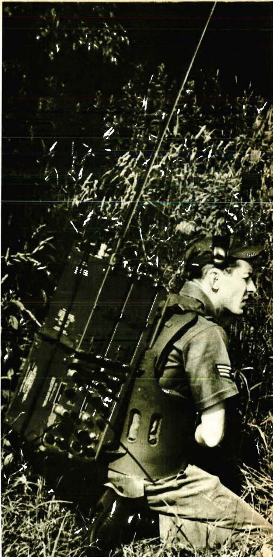
Designed by the Rome Air Development Center, this forty-eight-pound radio pack provided enough communications equipment for one man in the field to operate a forward-control command post.
