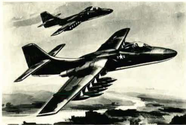
Northrop Corp.'s A-X prototype is known as A-9A and could be powered by either GE or Avco Lycoming engines. Low cost and ruggedness characterize the two designs.
