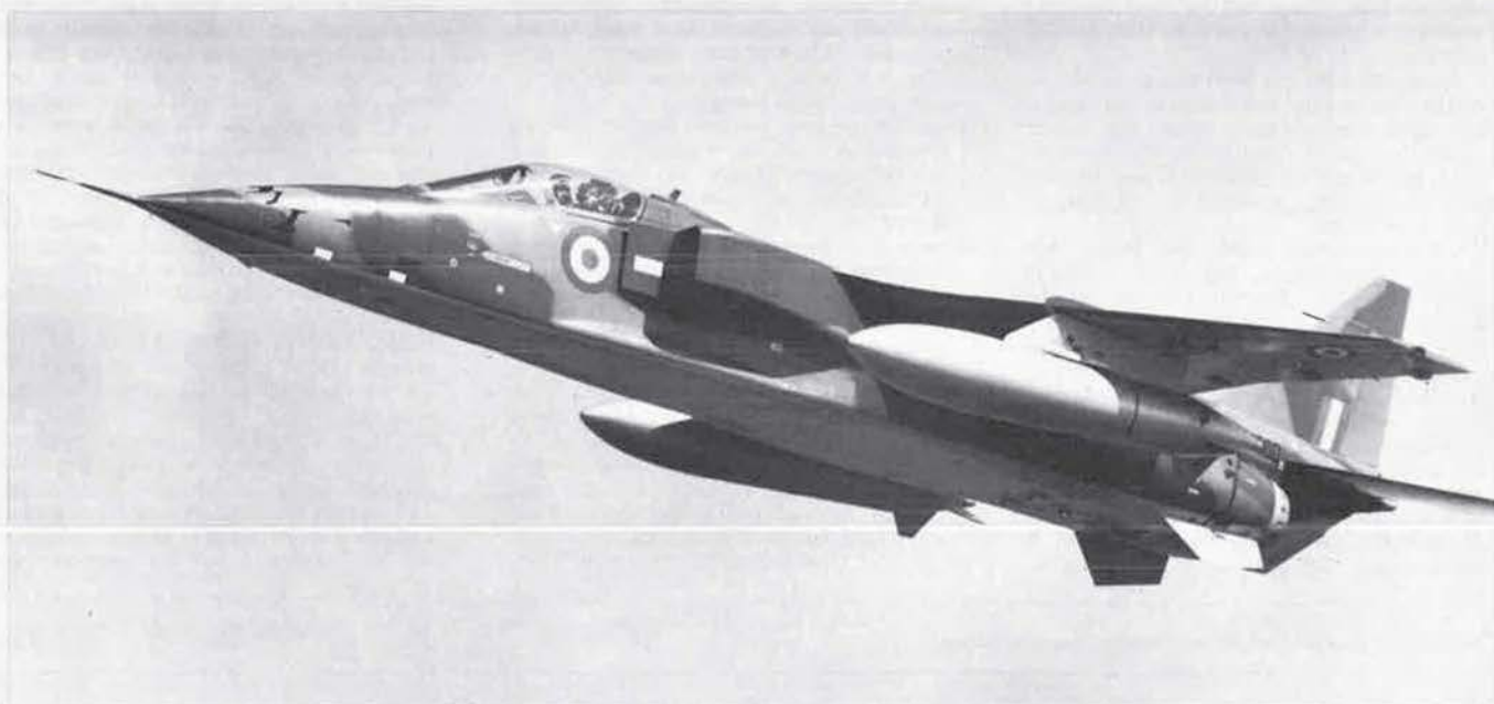
Jaguar S-06, first prototype of the single-seat tactical support version for the RAF, with underwing drop-tanks
