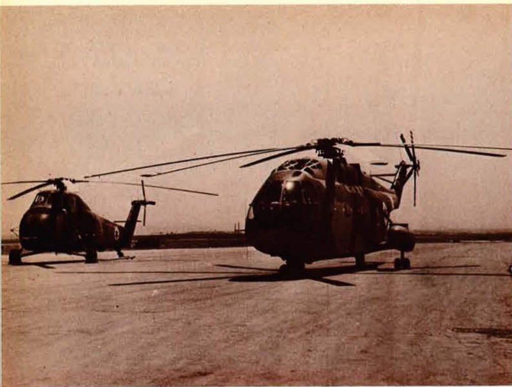
Helicopters play an important role in the Israel Air Force, in keeping with Israel's doctrine of military mobility. Above, at right, a French-built Super Frelon assault craft is lined up on the runway alongside a Sikorsky UH-34 utility helicopter.
