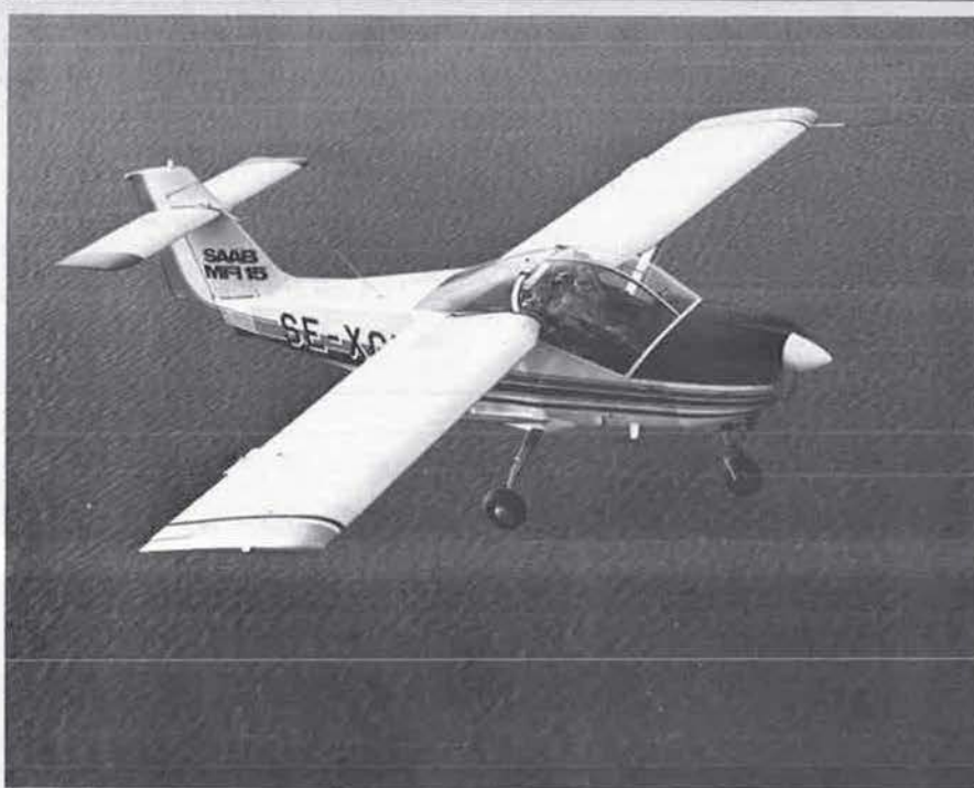
Saab-MFI 15 in production configuration, with 200 hp Lycoming IO-360-A1B engine and tricycle landing gear
