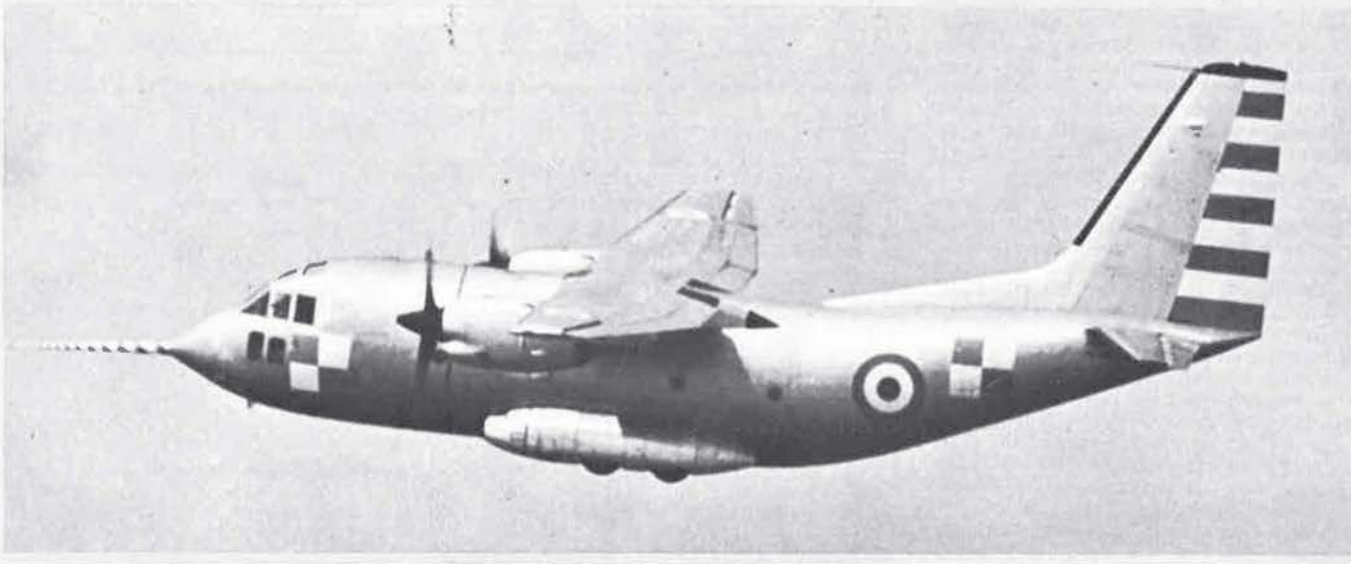
Fiat G222 general-purpose military transport (two 3,400 shp General Electric T64-P-4D turboprop engines)
