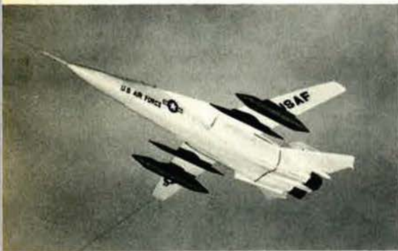
Variable-geometry fuel tanks developed by Whittaker Corp. are shown on model configuration. Full tanks (outboard) “shrink” to missile-like slimness (inboard) as fuel is transferred. Empty tanks are designed for supersonic speeds.
