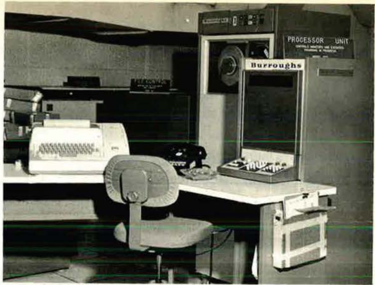
Computer capability is crucial to the mission of the Air Force Data Systems Design Center. This is the Center's Burroughs B-3500 computer system.
