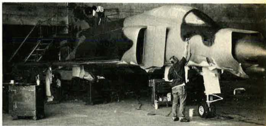
Personnel of the Ogden Air Materiel Area, Hill AFB, Utah, camouflage an F-4 Phantom as the final touch in the aircraft's overhaul and modification.
