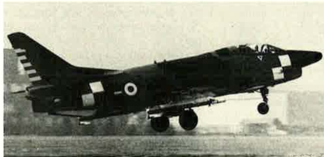
Fiat's G-91 YS, undergoing development for the Swiss Air Force, makes a test flight. The YS has special electronics and a third set of subwing pylons to carry Sidewinder air-to-air missiles.
