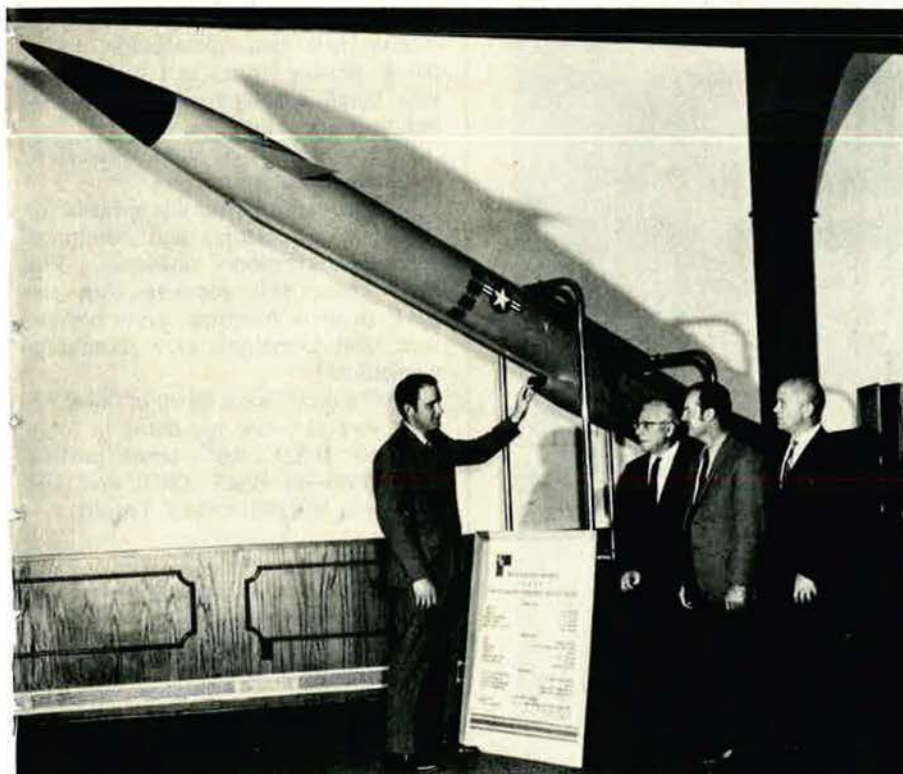
A new generation of missile targets is being developed by Beech Aircraft Corp. for the services with this high-altitude supersonic target (HAST). Sponsored by the Air Force Systems Command Armament Laboratory, HAST's hybrid rocket engine will utilize solid or liquid propellants and hit Mach 4 and 100,000-foot altitudes.
