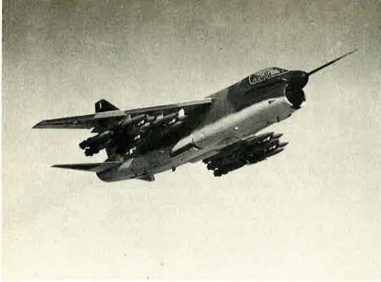
TAC's newest fighter, the A-7D Corsair II, can deliver ordnance almost equal to its own empty weight. This one is carrying twenty-four 550-pound bombs.
