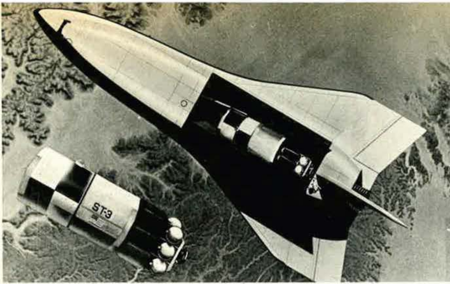
One of many artists' conceptions by NASA of the reusable Shuttle. The two-stage vehicle would be launched vertically, with both stages returning to earth after performing payload-delivery missions. Shuttle would largely end the "throwaway" booster era.
