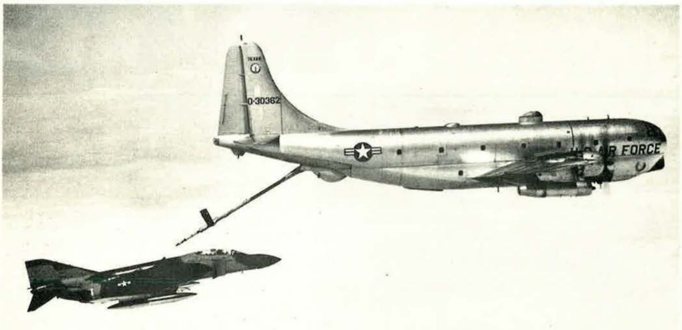
USAFE gets significant air refueling support from Air National Guard, demonstrated here in German skies. Guard maintains a permanent KC-97 refueling operation based at Rhein-Main AB, Germany.
