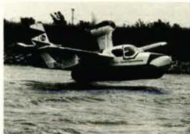
The ACLS-equipped LA-4 has landed and taken off on water, and has traversed muddy, ice-covered fields with ease.
