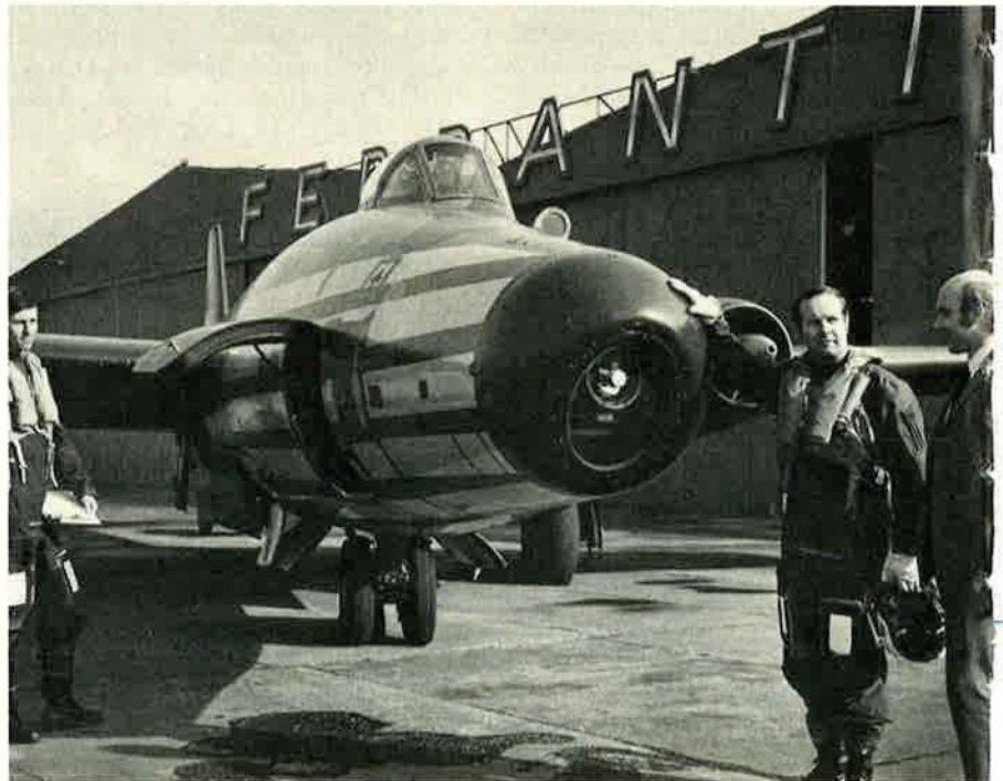
RAF's new Laser Ranger and Marked Target Seeker, in the nose of this modified Canberra, has flown for the first time. Ferranti Chief Test Pilot Len Houston, left, and Tech Rep John Maberley discuss the unique target ranging device.
