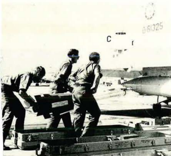
Minnesota ANG weapons-loading team handles tricky job of stowing Falcon missile aboard munitions bay of an F-102.
