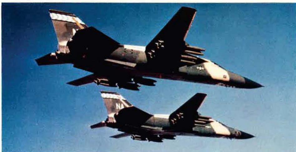
Fowler flaps and full-span slats (visible here), and multiple-disc, antiskid brakes allow the F-111 to land in a couple of thousand feet without a drag chute.
