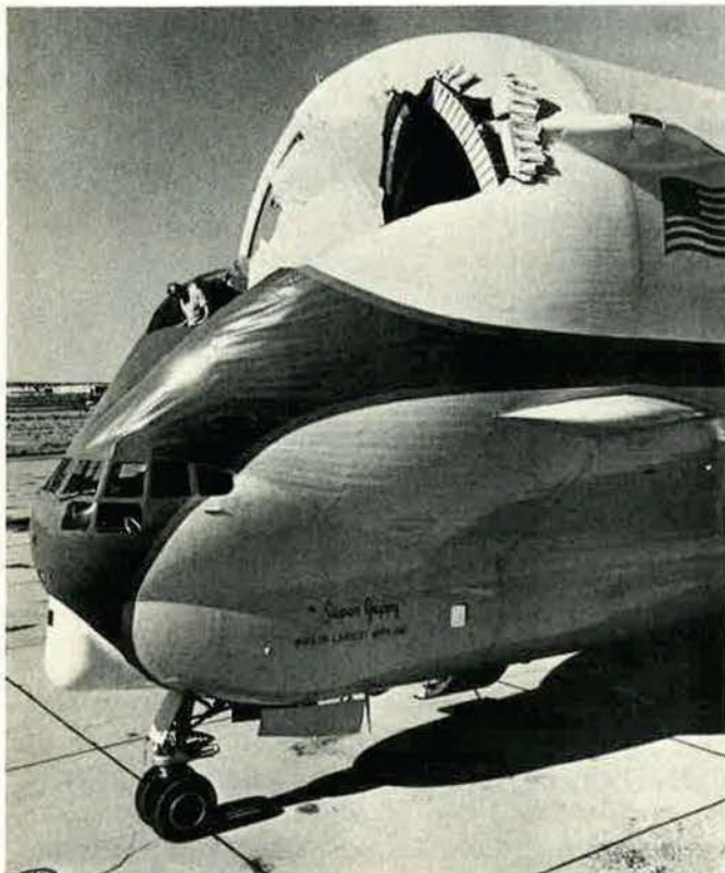
Miraculously, the Guppy made it back with a twenty-three-foot hole in her nose, imploded by the force of a test dive.
