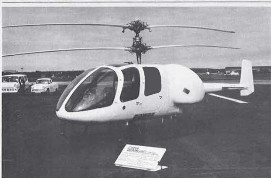
Cierva Rotorcraft CR.LTH-1 utility helicopter (two 205 hp Rolls-Royce Continental IO-360 engines) (Air Portraits)
