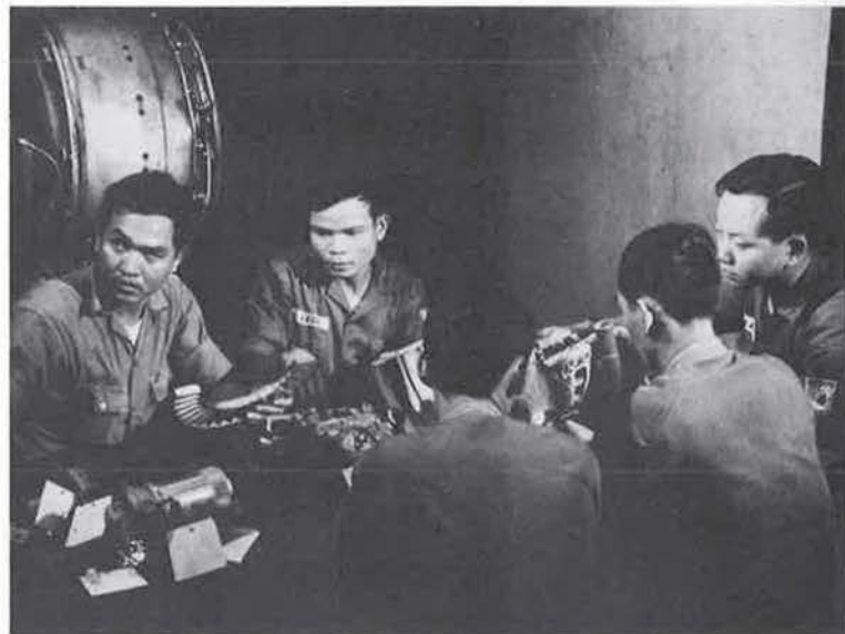
VNAF airmen strip down a CH-47 Chinook helicopter engine as part of the training received from US Army aviation personnel at Phu Loi Army Airfield, Vietnam. When the training is completed, the choppers are turned over to the Vietnamese.
