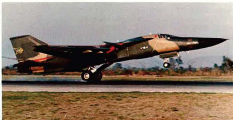
Fowler flaps and full-span slats (visible here), and multiple-disc, antiskid brakes allow the F-111 to land in a couple of thousand feet without a drag chute.
