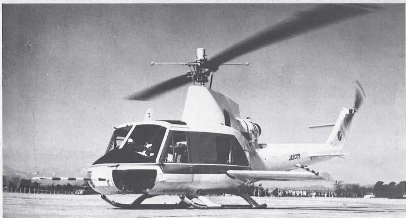
Another view of the Fuji XMH high-speed winged research helicopter, converted from a company-owned Fuji-Bell 204B
