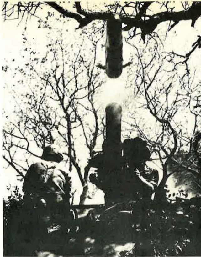
US Army's new TOW antitank missile, recently deployed to infantry units, is caught by high-speed camera during test firing. TOW, built by Hughes Aircraft Co., can destroy any known enemy armor at ranges of more than a mile, and can be fired from ground tripods, a variety of vehicles, and from helicopters.
