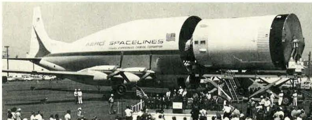
A "shocking disregard for aerodynamic aesthetics" allows the modified C-97 to carry this third stage of Saturn IVB, the booster that powers Apollo moon rockets from earth orbit to lunar orbit.
