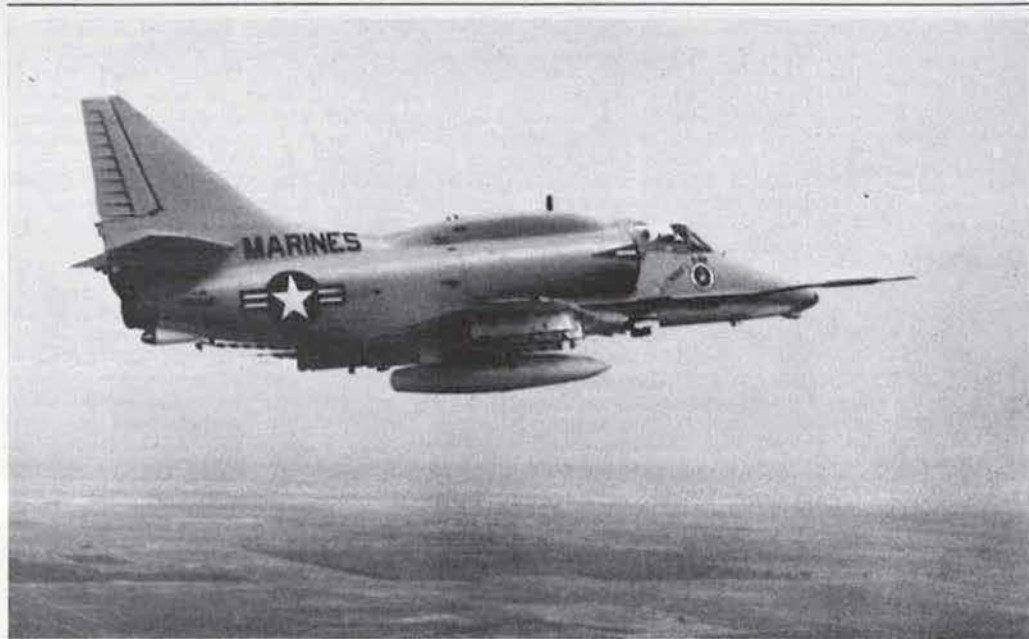
McDonnell Douglas A-4M Skyhawk attack aircraft (Pratt & Whitney J52-P-408A turbojet engine)
