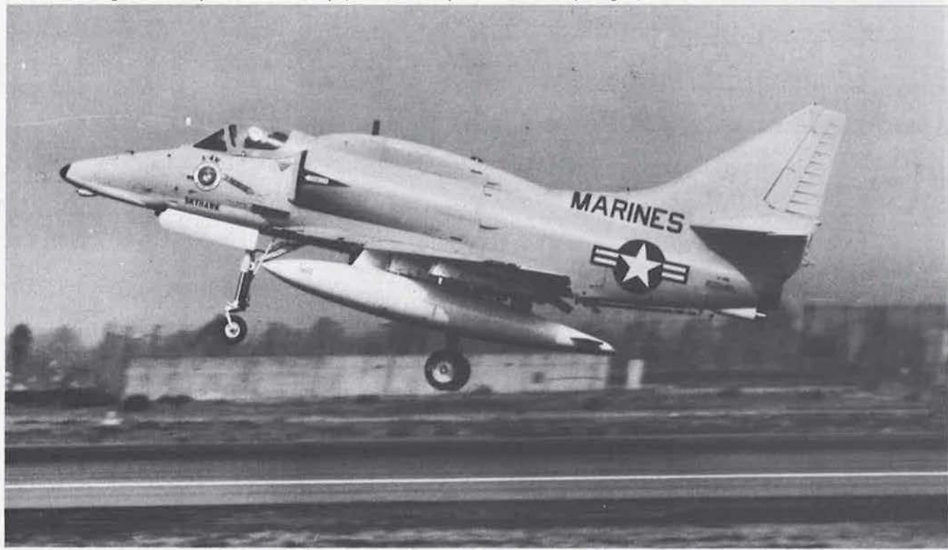
McDonnell Douglas A-4M Skyhawk attack aircraft (Pratt & Whitney J52-P-408A turbojet engine)
