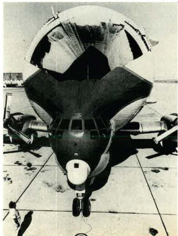
Miraculously, the Guppy made it back with a twenty-three-foot hole in her nose, imploded by the force of a test dive.
