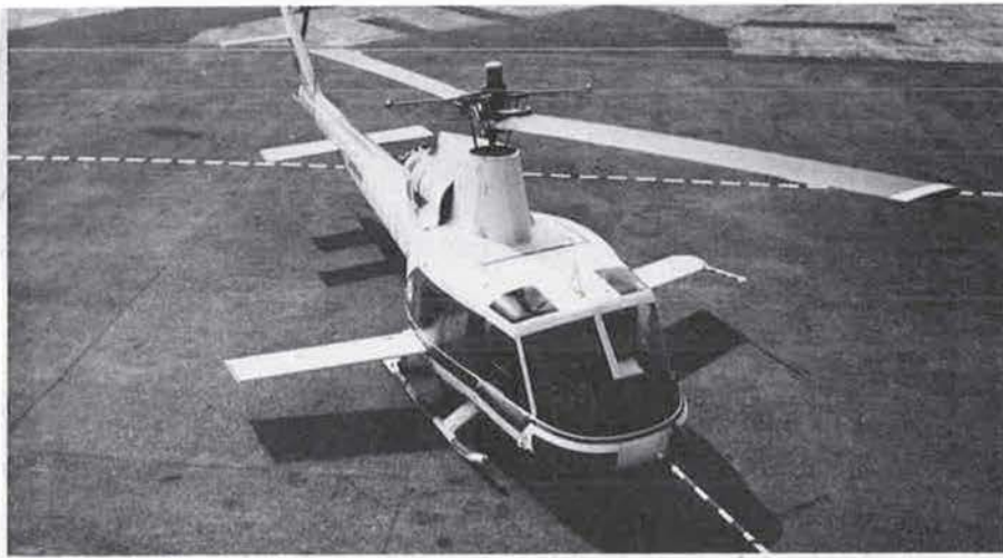
Fuji XMH high-speed winged research helicopter (converted from a company-owned Fuji-Bell 204B)
