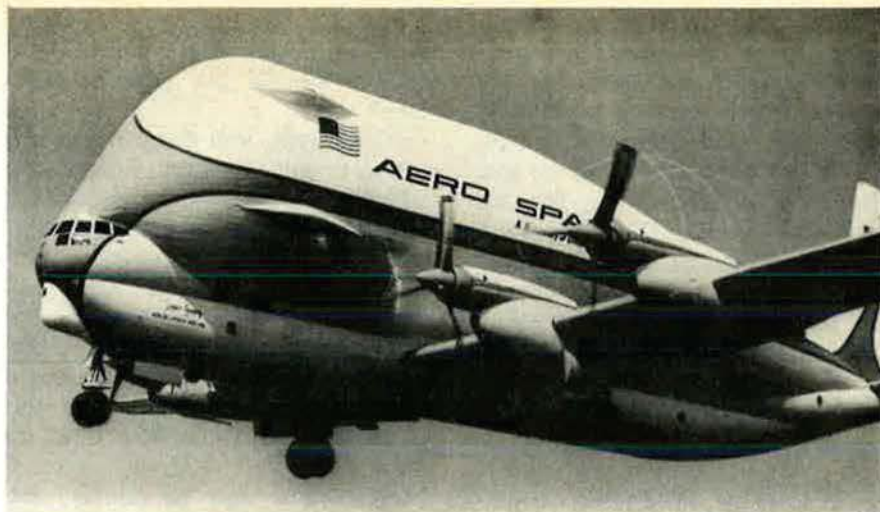
Super Guppy's cargo compartment is larger than C-5A's. Projections behind the cockpit are hinges for her swinging nose.
