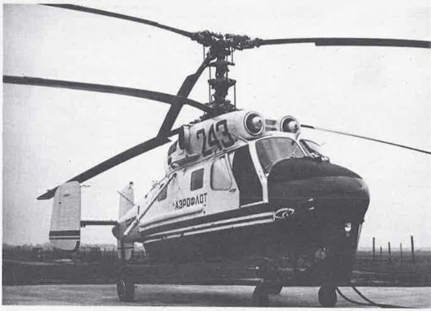
The Ka-25K commercial flying-crane helicopter demonstrated at the 1967 Paris Air Show. A detachable under-nose gondola, containing a rearward-facing pilot's seat with dual flying controls for use during loading and unloading, replaces the radome of the military anti-submarine version (Tass)
