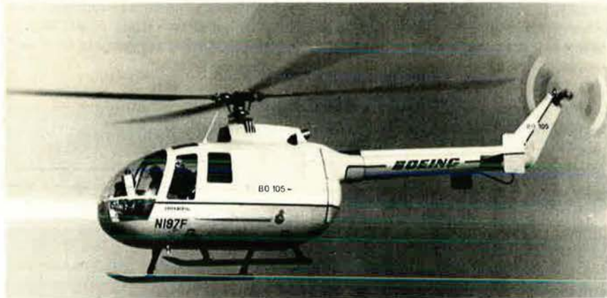
Germany's first successful postwar helicopter, the Bo105, has reached the mass-production stage. A twin-engine aircraft, the Bo105 has as its power source a unique rigid and hingeless rotor that utilizes fiber-glass technology.
