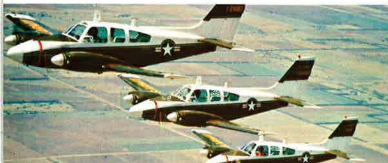
In service at Ft. Rucker since 1965, the Beechcraft T-42A was selected as a twin-engine instrument and transition trainer after a 2-year competitive evaluation. Its record of 90% ready rate is proof that it was a wise choice.
