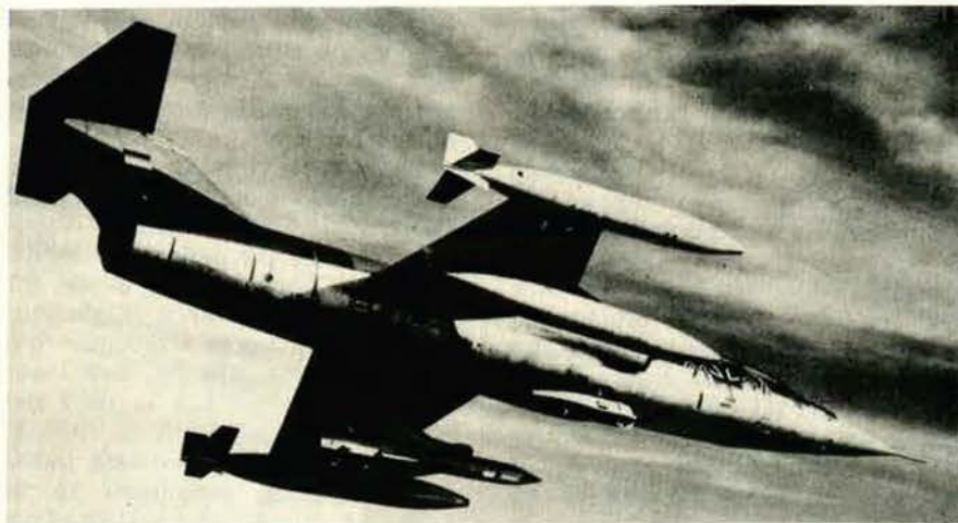
A Luftwaffe F-104G carrying a Cormoran streaks toward a target in a practice attack. While most details of the new missile remain under security, it is known that the weapon is supersonic, with a range of forty miles and jam-proof guidance.
