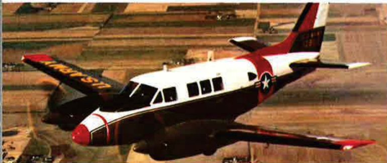
In service since 1964, the twin turboprop Beechcraft NU-8F provides a 1280 nm range and a cruise speed of over 200 knots.
