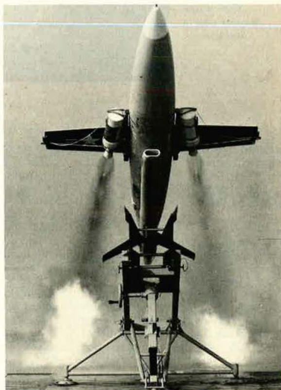
Pictured here is the Chukar jet-powered target drone that will be employed in training NATO anti-aircraft missile crewmen on the island of Crete in the Mediterranean. Ventura Div. of Northrop Corp. produces the missile and will supply service at the training installation under a three-year contract. See accompanying text for further details.
