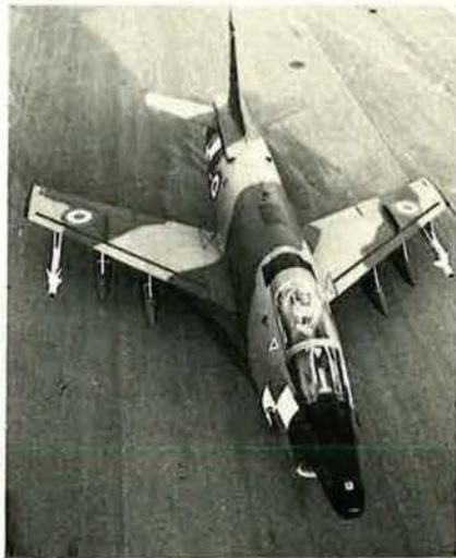
This Fiat G-91 YS has been developed specifically for the Swiss Air Force and equipped with a third set of subwing pylons to accommodate Sidewinder air-to-air missiles for defense.
