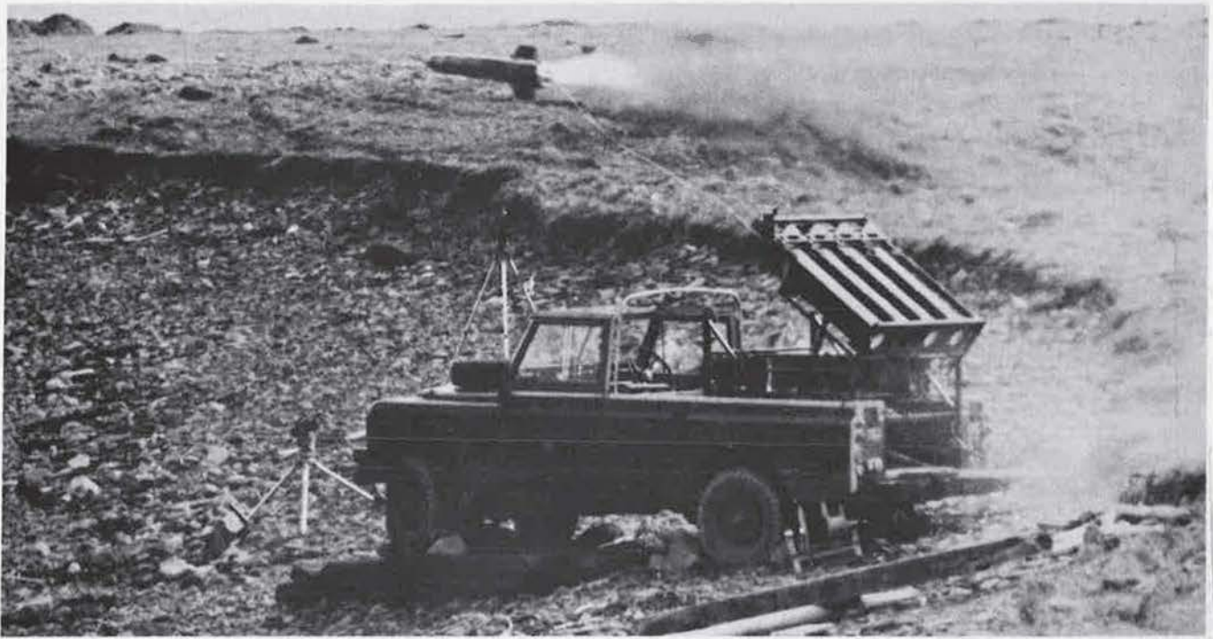
Swingfire long-range anti-tank missile at moment of launch from a pallet mounted on a Land-Rover
