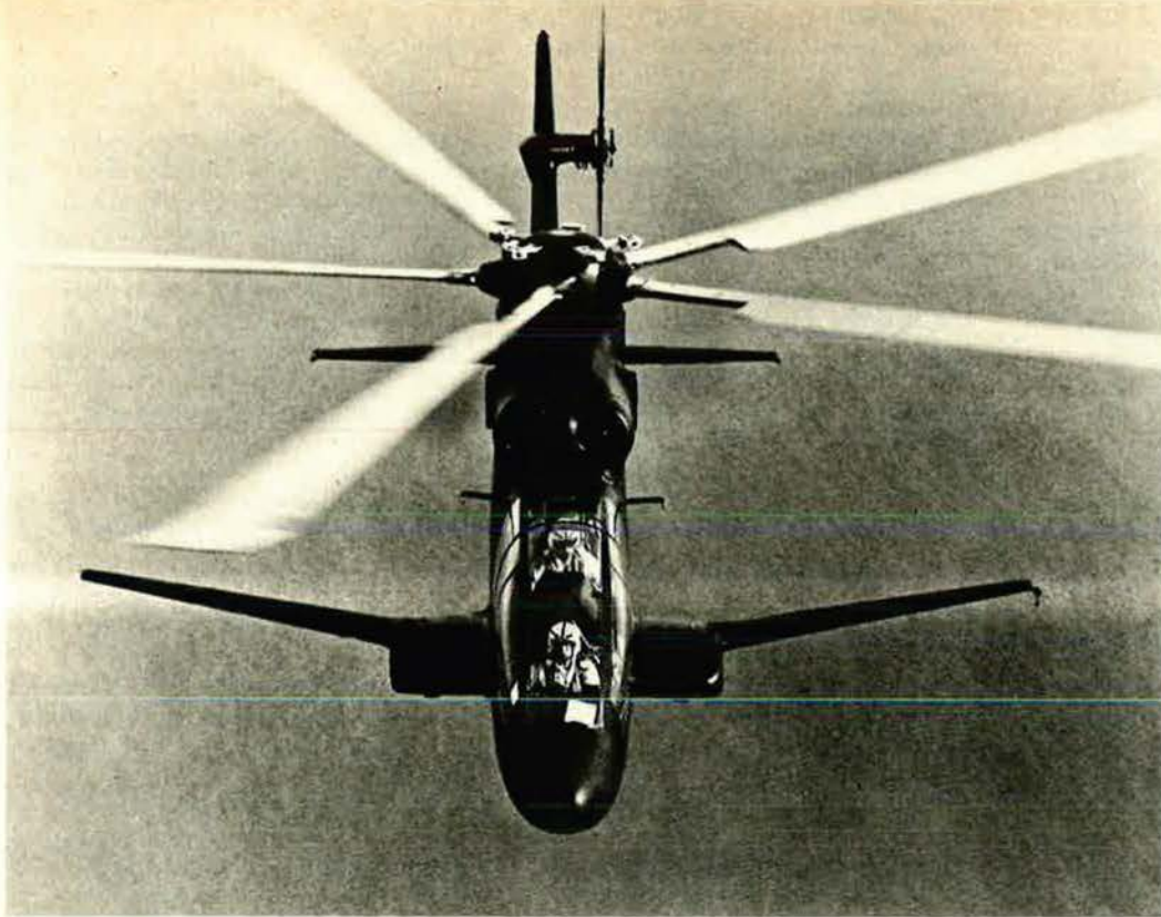
Sikorsky's new S-67 high-speed helicopter can be equipped with a variety of weapons: guns, cannon, grenade launchers, rockets, and missiles. The twenty-eight-foot wing provides some of the lift, and wing-mounted speed brakes allow a steeper dive angle. The S-67 also has an airplane-type vertical fin and a controllable horizontal stabilizer. Its streamlined rotor head fairing greatly reduces drag. (For additional details, see page 107.)
