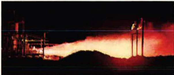
Powerhead (Fuel Turbopump, Pre-Burner and Main Case) for XLR129 reusable rocket engine undergoes static test.
