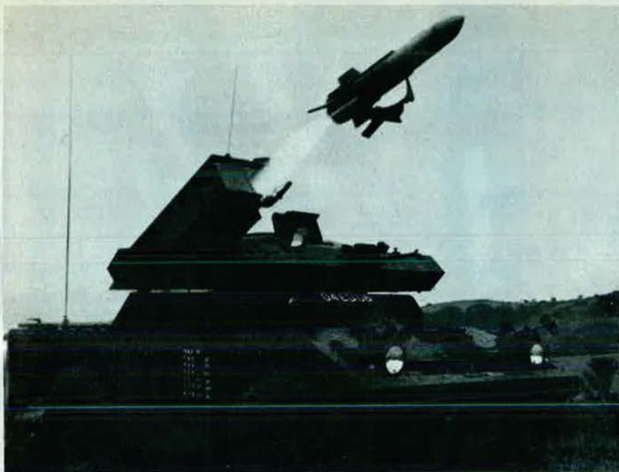
Swingfire long-range anti-tank missile system installed on a Ferret scout car of the Royal Armoured Corps
