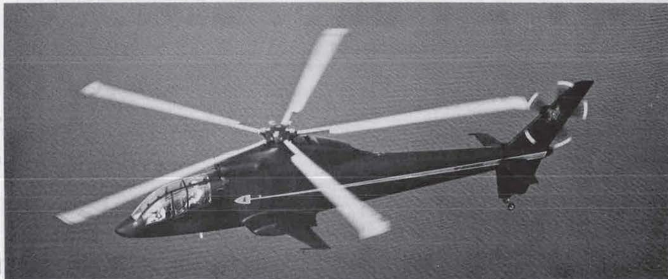
Prototype Sikorsky S-67 Blackhawk combat helicopter (two 1,500 shp General Electric T58-GE-5 turboshaft engines)
