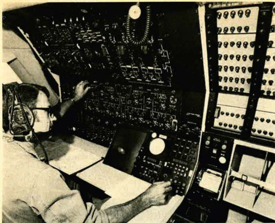
Reflecting the complexity of USAF's C-5 transport is just this one control panel onboard. Switches, gauges, and dials monitor such subsystems as fuel and oil, hydraulics, pneumatics, and electrical circuits in the huge craft.
