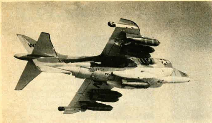
A Hawker Siddeley V/STOL Harrier in US Marine Corps markings struts its stuff while toting 8,000-pound bomb load. Deliveries of the V/STOL begin in 1971.
