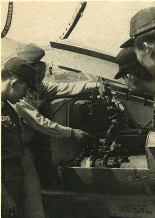
One of the most successful techniques in Vietnam has been the mounting of Miniguns on combat aircraft. And among the most serious students of the Minigun have been South Vietnamese, here studying the weapon on an A-37.
