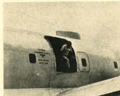
Teledyne McCormick Selph, Hollister, Calif., is testing "high-energy exit systems" for military and commercial use. It has been determined that many crash fatalities are the result of a lack of operable fuselage exit points.
