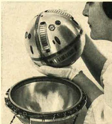
Northrop is a major designer and builder of navigation and guidance systems for long-range subsonic and supersonic aircraft. The heart of one such system is this unique spherical platform.
