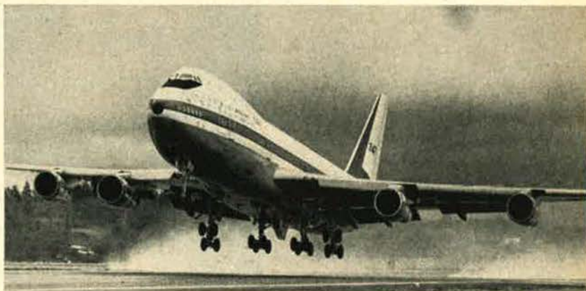
Northrop saved more than 2,000 critical pounds in designing the 153-foot fuselage for the magnificent 747 airliner.
