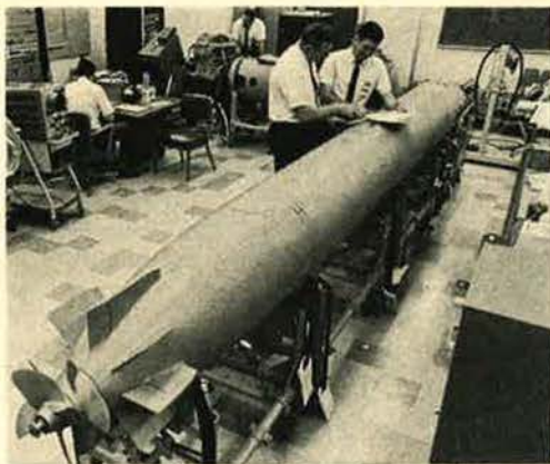
This underwater vehicle designed by Northrop for the U.S. Navy to simulate a full-sized submarine will permit significant savings in anti-submarine warfare training.
