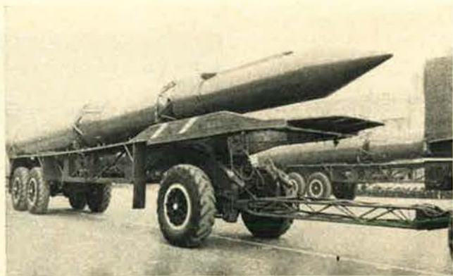
Soviet strategic forces include more than 800 SS-11s and SS-13s. Shown here is the solid-fueled SS-13 missile.
