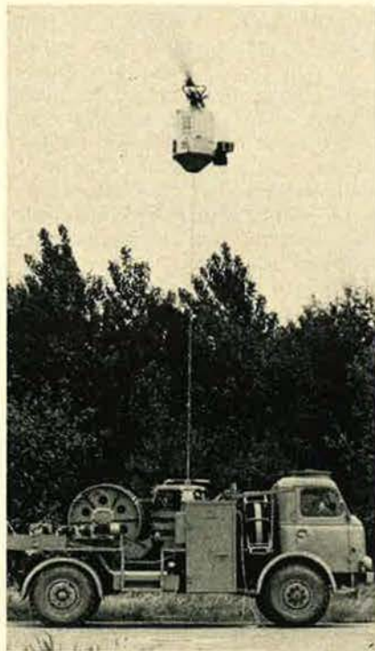
The Dornier Do.32K Kiebitz tethered observation platform undergoes a test launch from its truck-mounted ground-support vehicle. From moderate altitudes it could provide field commanders with much-needed reconnaissance.
