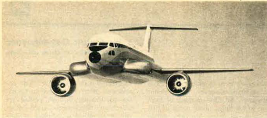
One of the projects for a high-speed fan-lift V/STOL airliner studied by Hawker Siddeley, the HS 141 will seat 100 passengers, cruise at more than 600 mph, and operate at ranges between 150 and 1,300 miles. Two types of engines—a set for vertical flight and a set for horizontal flight—are to be utilized.
