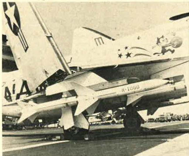
A radar-controlled Sparrow III air-to-air missile is shown mounted aboard an aircraft. Built by Raytheon Co., Sparrow III is the main armament of the F-4 Phantom interceptor. It is also the system upon which NATO's Seasparrow cooperative development program is being based.
