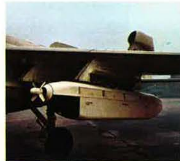
Advanced pod-mounted ECM system
