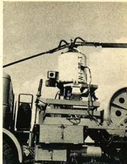
The Kiebitz is shown aboard the cradle of its truck mount. Much information and the probable future use of the observation device are still under security wraps. Its vehicle-mounted support gives Kiebitz cross-country mobility.
