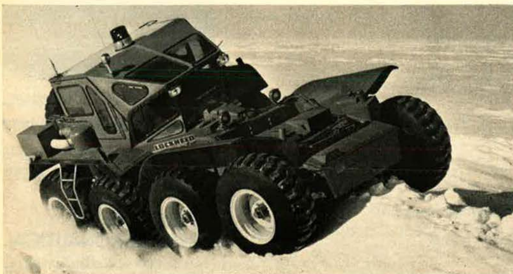
While most of us are looking forward to autumn's golden weather, some have already experienced winter, especially those involved in tests of Lockheed's unique Twister. The off-road vehicle's recently completed Arctic trials are the latest in a four-year series that included performance in terrain ranging from marshlands to desert sands.
