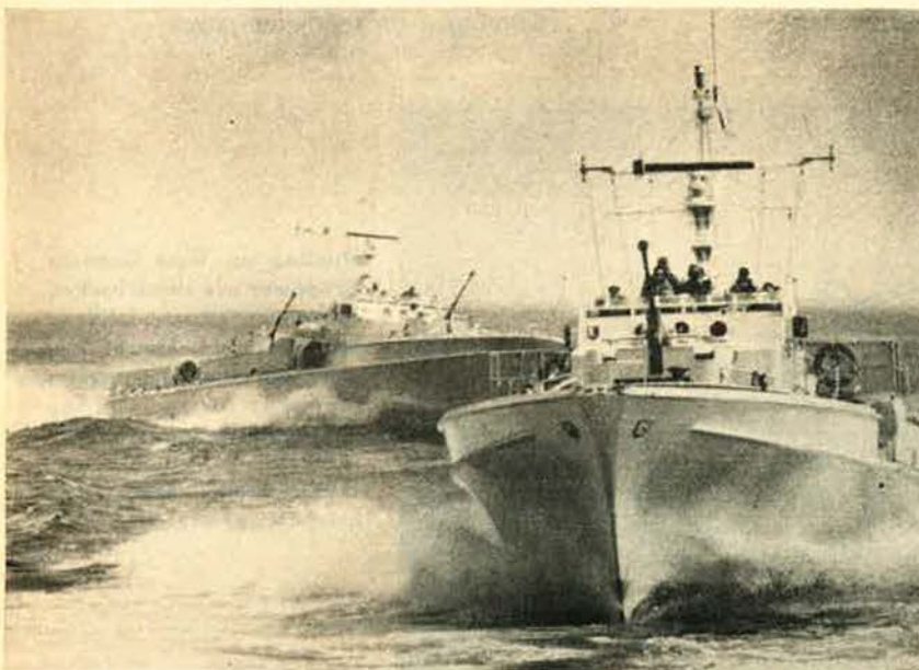
German Navy motor torpedo boats undertake a patrol. German naval forces are slated to receive new submarines as well as missile-armed, fast MTBs. The type shown here are of the Jaguar class.
