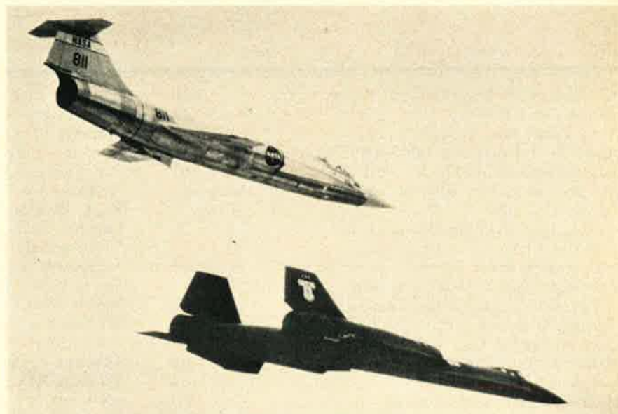
High in the skies over Southern California, a "blackbird" YF-12A research aircraft—the world's fastest interceptor—is shadowed closely by a "chase" Starfighter. The planes, both built by Lockheed-California Co., work for NASA in training astronauts and observing the performance of high-speed aircraft undergoing tests at Edwards AFB.
