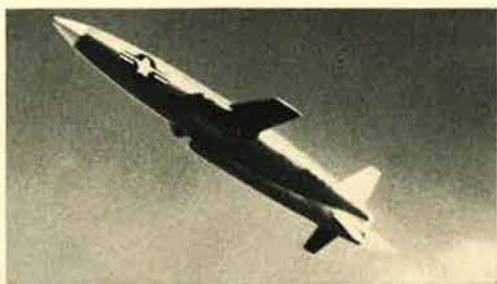
The most modern target in service for low-level surface-to-air missile training, the MQM-74A has the lowest cost per mission in its performance class.
