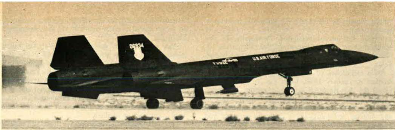
The YF-12A, a record-breaking Mach 3 interceptor, was developed rapidly under a tightly structured, orderly management approach.
