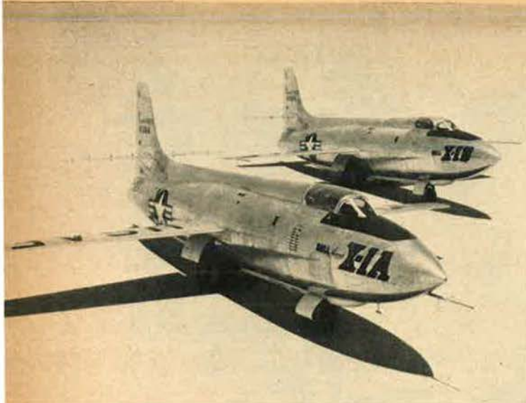
Bell Aircraft's X-1A and X-1B, derived from the supersonic X-1, attained Mach 2 speed and reached altitudes above 90,000 feet.
