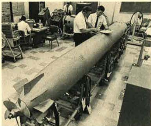
This underwater vehicle designed by Northrop for the U.S. Navy to simulate a full-sized submarine will permit significant savings in anti-submarine warfare training.
