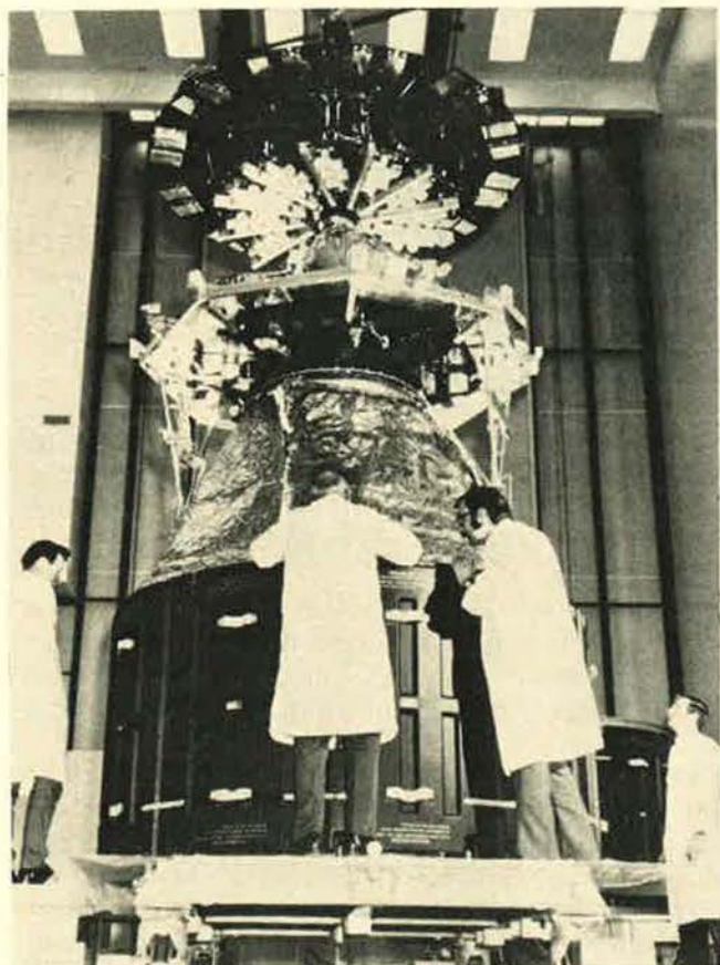
Technicians work on a full-scale thermal model of the world's largest communications satellite—Intelsat-4—two of which are to be assembled by the British Aircraft Corp.
