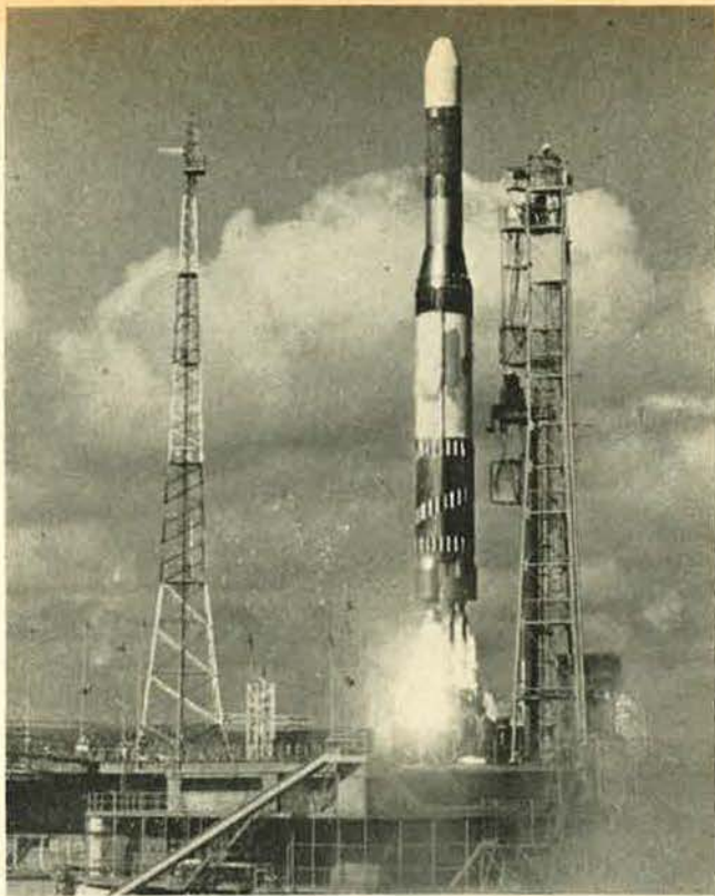
Europa 1 first and second stages undergo launch from Australia's Woomera range during a test series there.
