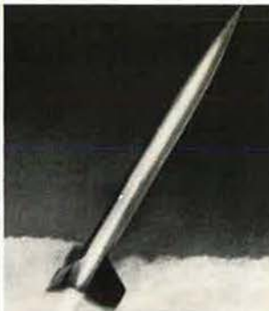
1946 Supersonic ASR-1 Aerobee used by USN in upper-atmosphere research programs.
