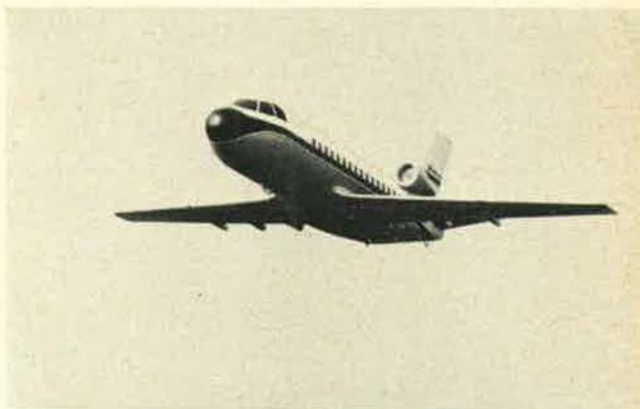
The VFW 614, Germany's first passenger jet airliner, is designed for economic operations on feeder and regional routes. Its twin jet engines are mounted atop the wing.
