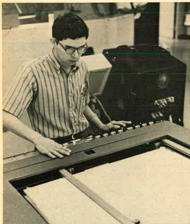
Aircraft flying in and around the West Coast Test Center are followed by this X-Y Recorder and are monitored by operators who are in constant contact with the MFSO.
