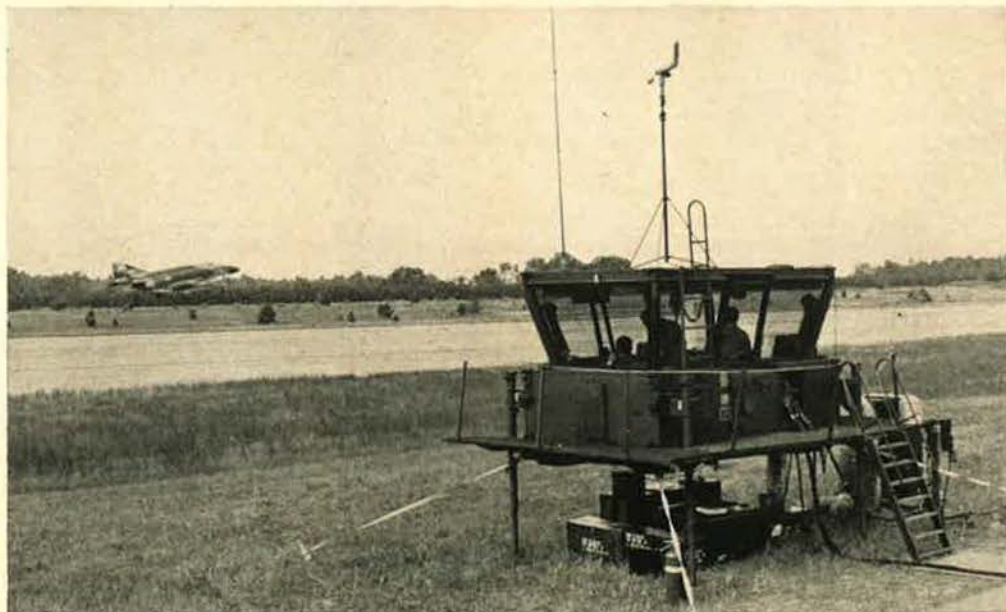
The challenge to airlift capability in the Coronet Bare operation was formidable. A fleet of thirty-two TAC C-130s was engaged, backed up by MAC C-141s. They brought in some 3,000 tons of cargo, 1,160 personnel, and 451,000 gallons of POL. Among the equipment essential in running a modern airfield is the AN/TSW-6 mobile control tower at the left.
