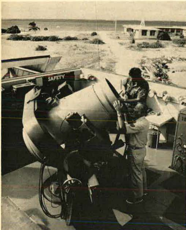
This Baker-Nunn camera, operated by ADC's Fourteenth Aerospace Force, is capable of photographing an object the size of a basketball at a distance of 25,000 miles in space.
