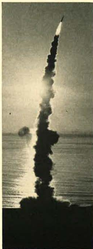
A three-stage, solid-fuel Minuteman ICBM is launched from a test silo at Vandenberg AFB, Calif. Six wings of the solid-propellant missile totaling a force of 1,000 form the backbone of SAC's missile strength. Minuteman III versions are designed to employ Multiple Independently Targeted Reentry Vehicle (MIRV), capable of carrying up to seven nuclear warheads to assigned targets.
