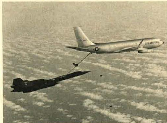
An SR-71, the world's most advanced strategic reconnaissance aircraft, is refueled by a KC-135 Stratotanker. The SR-71 can fly at more than three times the speed of sound.
