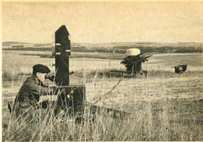
An upcoming close-quarter air defense system is BAC's Rapier, which promises competition for Tigercat. The supersonic weapon, designed for one-man operation, is highly mobile and can be mounted aboard tanks or APCs.
