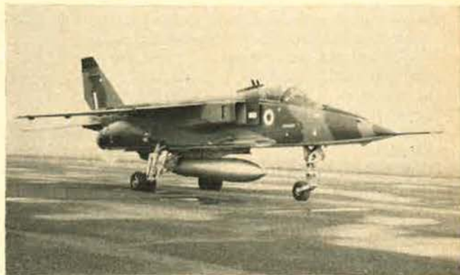
The BAC/Breguet Jaguar strike-trainer program is proceeding. This is the Jaguar S.06 version on the runway. It carries a 264-gallon fuel tank and is armed with two 30-mm cannon. The aircraft's flexible design fits it for a variety of operations: tac support, recce, and training tasks.
