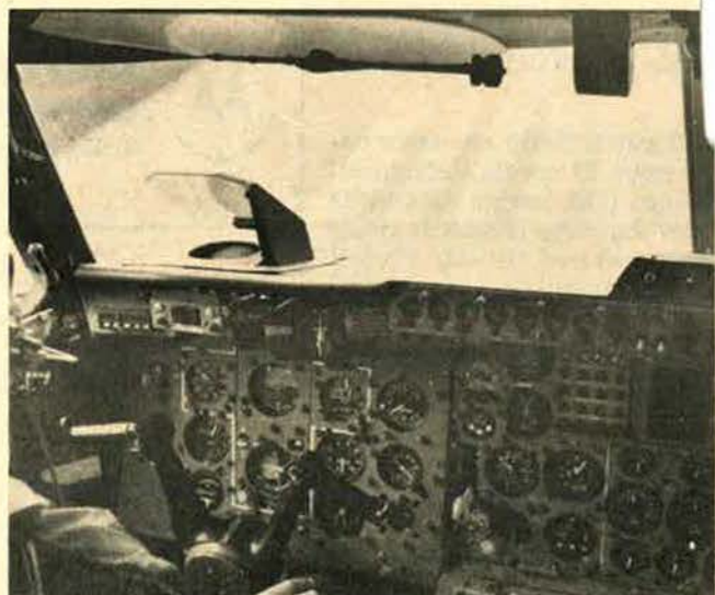
A Short Belfast XR 371 makes a fully automatic, hands-off landing at Amsterdam's Schiphol Airport during recent trials of the Smith Mk29 autoland system. The Belfast is the world's first military transport aircraft to become operational with the fully automatic blind-landing system.
