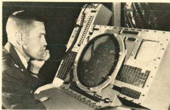
Lt. Col. Charles J. Turner checks out display console built by Hughes Aircraft Co.'s Fullerton, Calif., facility for the Air Force's 407L program. Such lightweight, multipurpose electronic gear is being integrated into the overall role planned for future mobile centers handling tactical air operations.
