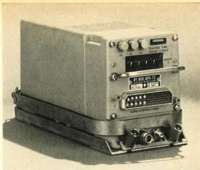
Microminiaturized AN/APX transponder, which is compatible with the commercial system for FAA air traffic control.
