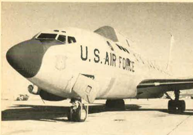
A flying camera platform, this NKC-135A jet aircraft is one of four specially equipped planes recently added to the Air Force Eastern Test Range inventory. The aircraft will participate in AF R&D programs analyzing the effects of reentry on missiles and on other space objects.
