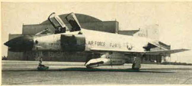
Shown on this F-4 Phantom is a pod housing a high-performance bomb-delivery system that permits great accuracy in tracking targets. The new system is being built for the Air Force by Philco-Ford's Aeronutronic Division, of Newport Beach, Calif., and has passed a series of tests.
